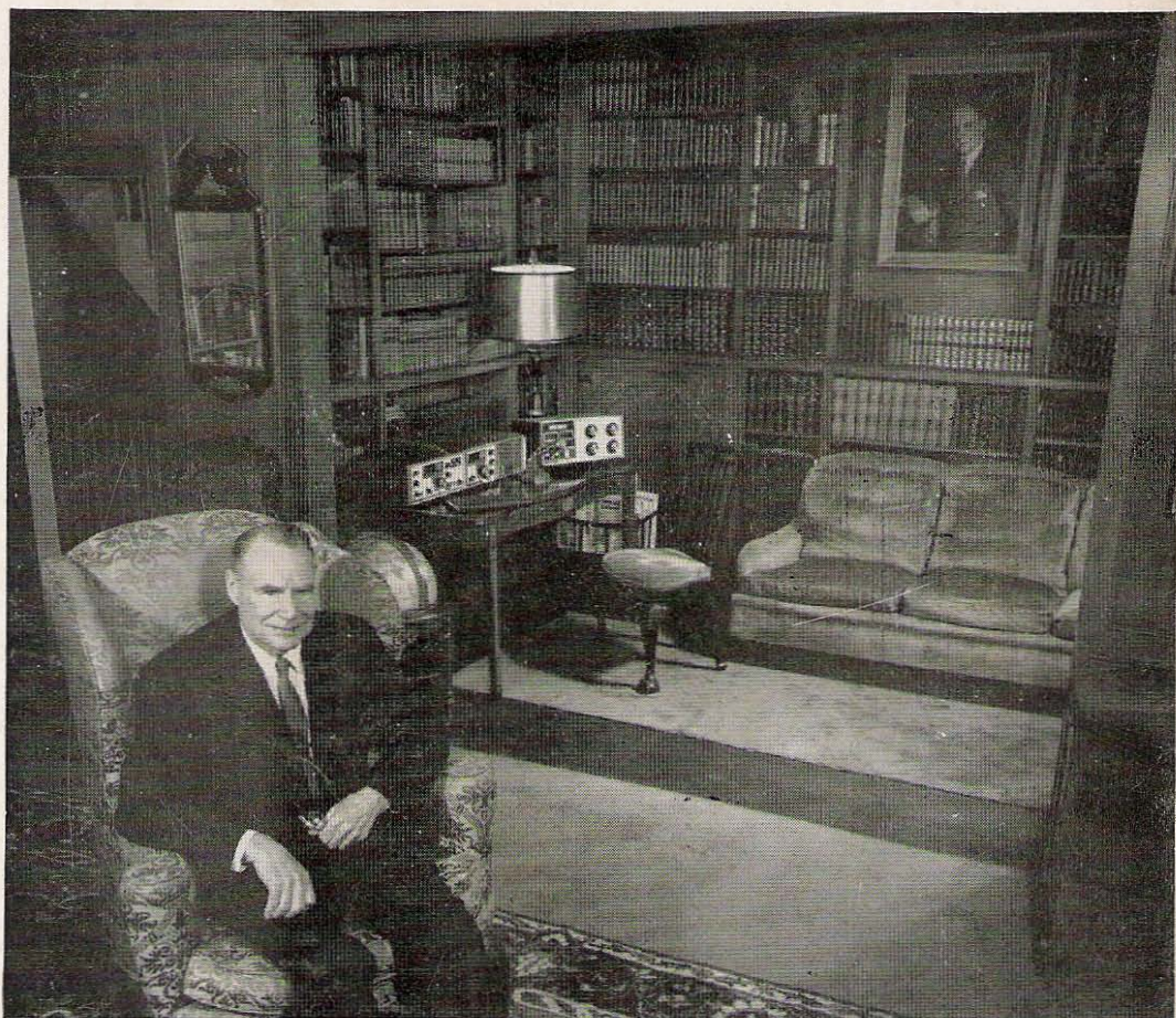
Amateur station W1AUC includes the NCX-5 Transceiver with digital dial, the NCX-A AC Supply/Speaker Console, the VX-501 VFO Console (all in walnut cabinets), and the NCL-2000 2 KW Linear Amplifier.
