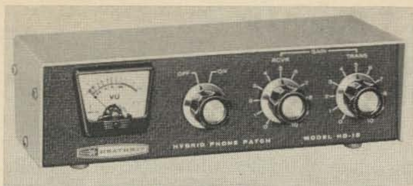
Fig. 4. The Heath HD-15 Hybrid Phone Patch employs a VU meter for monitoring input level to the telephone line and indicating correct null adjustment.
