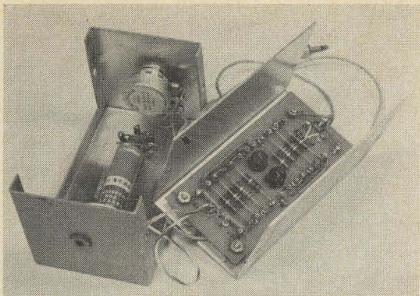
Balanced transistor amplifier for photovoltaic cell light meter. This shot was taken with a 4 x 5 inch camera.
