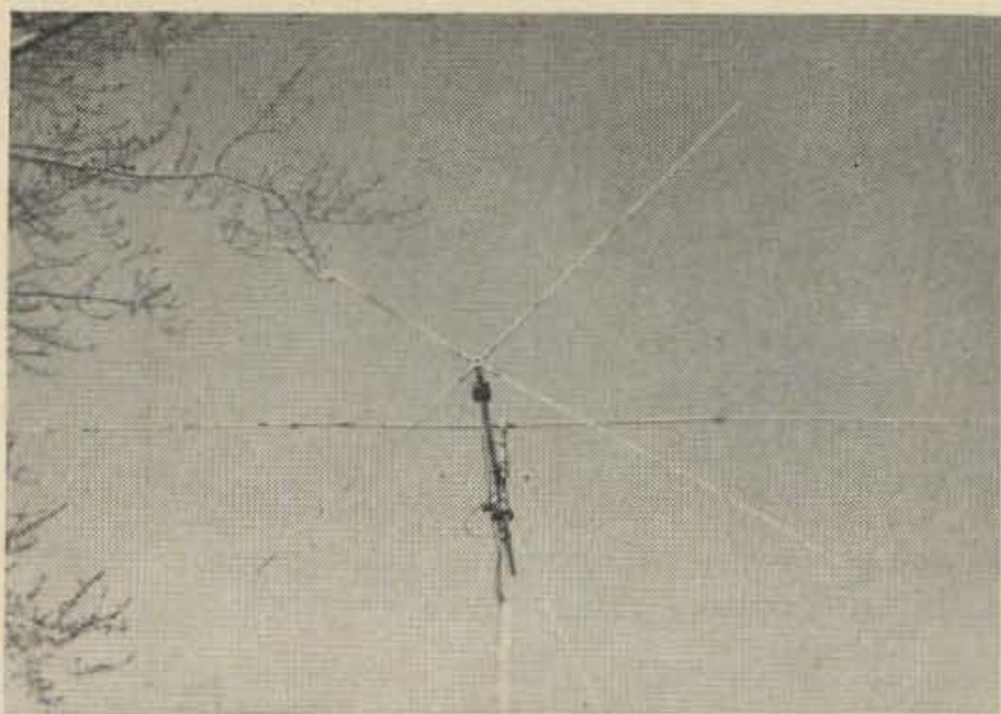
Here's the dipole in place between the two elements of the quad.
