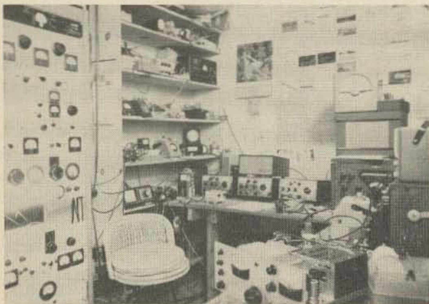
Part of K6RIL's shack. The six meter Swan 120 is in the right foreground. The rack on the left contains a kilowatt and transverter for 432 MHz, a 2 kW PEP rig for six and a 2 kW amplifier and transverter for 144.
