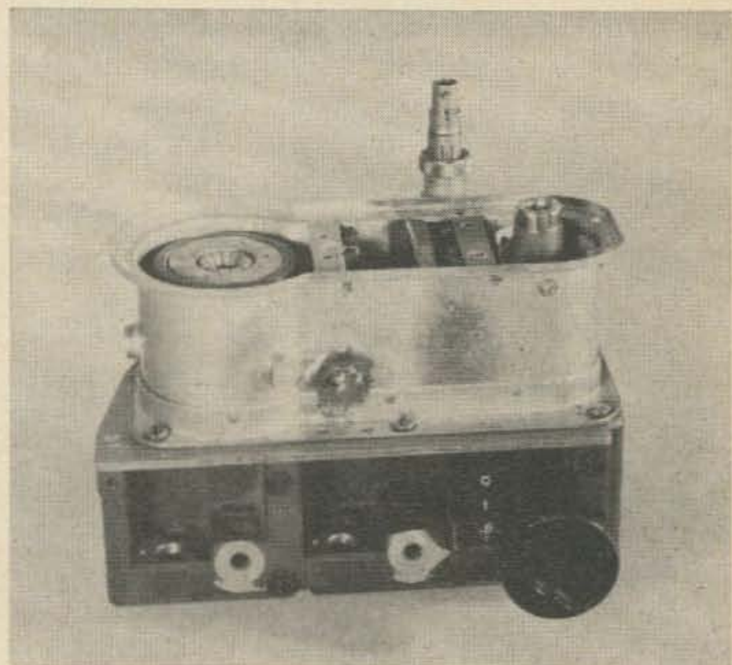
Front view of the cavity assembly and gear housing before installation of the cathode cavity plate.
