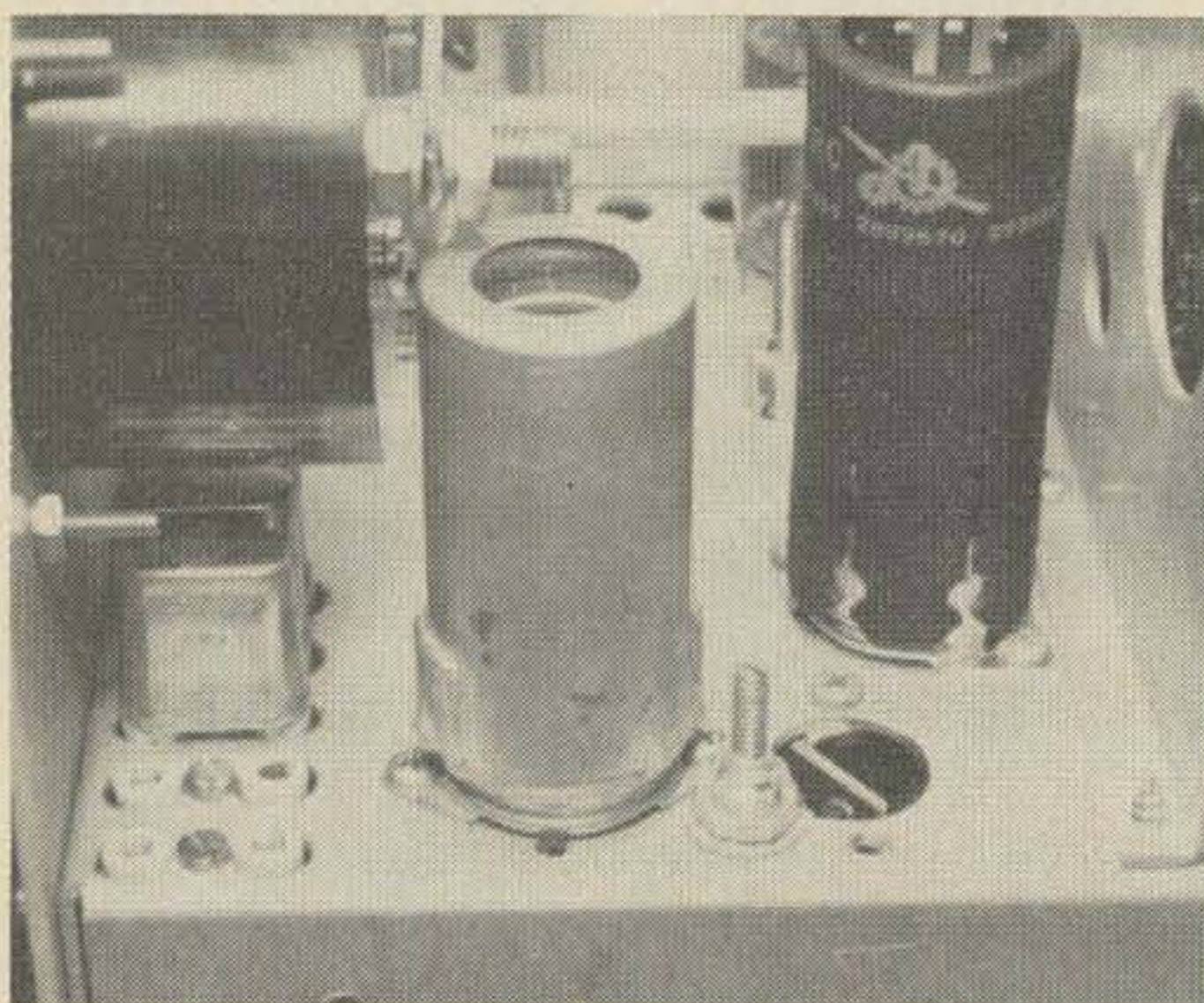
The new local oscillator and driver tubes and crystal sockets are mounted below the meter. The extra hole in the foreground was evidently punched by a previous owner. Hole in the final compartment wall was for the original final socket.
