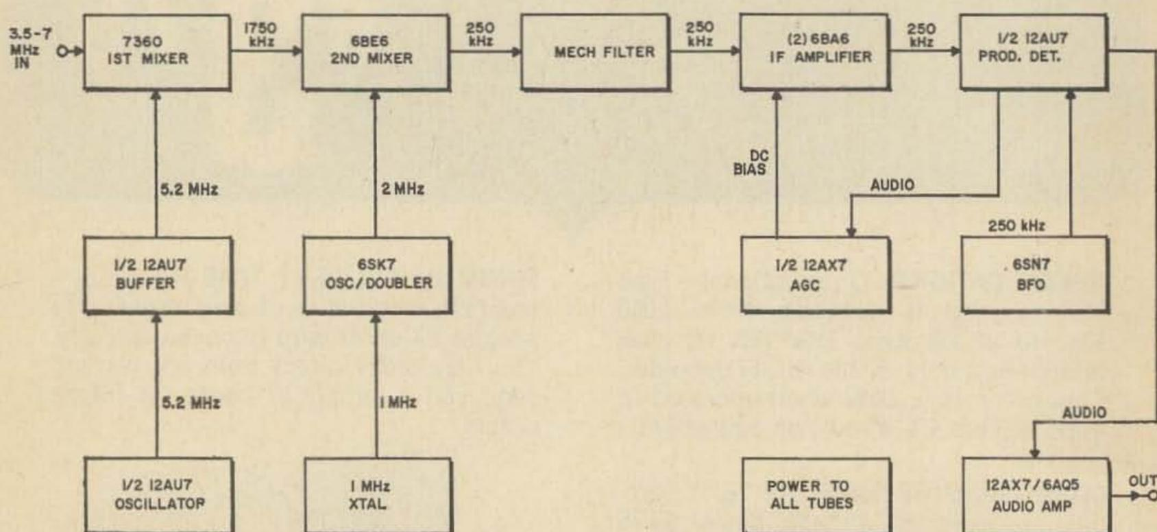
Fig. 1. Block diagram of the receiver.
