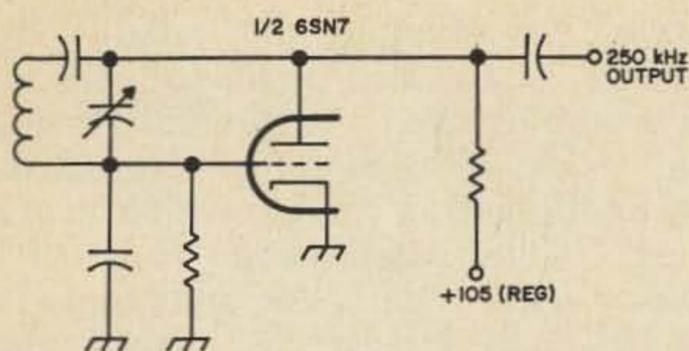
Fig. 6. BFO circuit.
