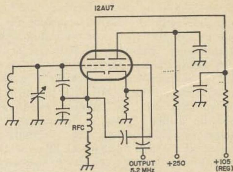
Fig. 2. Schematic of the oscillator circuit.
