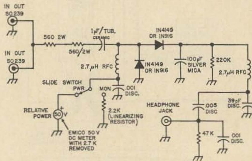
Fig. 1. Schematic for the Monitor.
