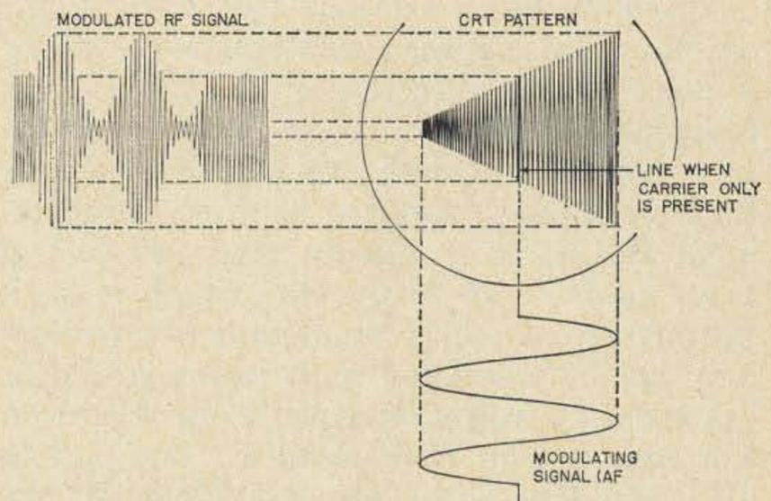
Fig. 12—Modulation-monitor pattern for checking quality of AM signal is developed in manner very similar to Lissajous figures as shown here. Pattern shown represents about 98% modulation (100% was not used in order to show how the negative-peak trace is developed). Audio signal should be taken from the modulator output, and RF signal sampled from the antenna feedline or antenna tuner, to get proper phase relationship and produce straight-sided patterns.
