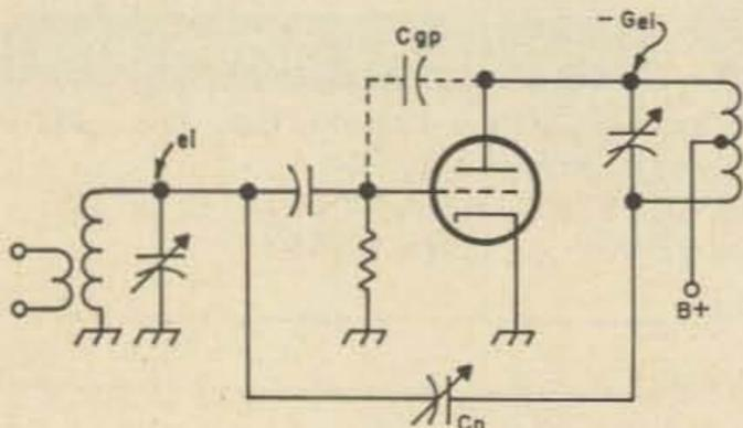
Fig. 1. Typical grounded cathode amplifier circuit.
