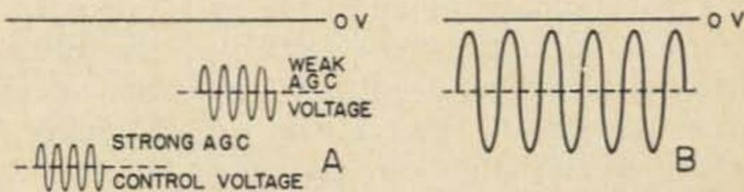
Fig. 5. AVC control voltage usually is not applied to large-signal *if* or audio stages because the output would be distorted under small-signal conditions. The signal is only small at the input end of the amplifier.
