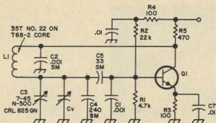
Fig. 2. Vackar oscillator circuit
