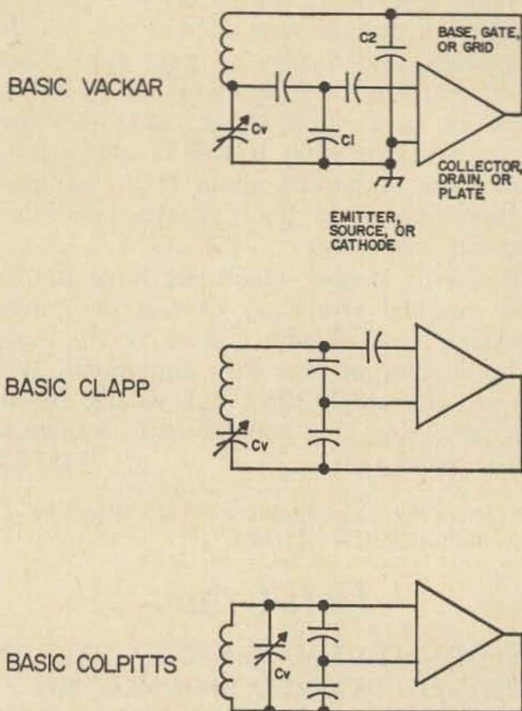
Fig. 1. Basic Colpitts and Clapp circuits are shown with The Vacker for comparison.
