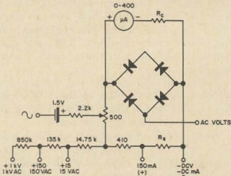
Here's a way to use a 150 mA VOM as a 0-450 micrometer—an increase in sensitivity of 333-fold. It takes no transistors, batteries, diodes, or, for that matter, wire or solder. The whole job can be done in five seconds.
