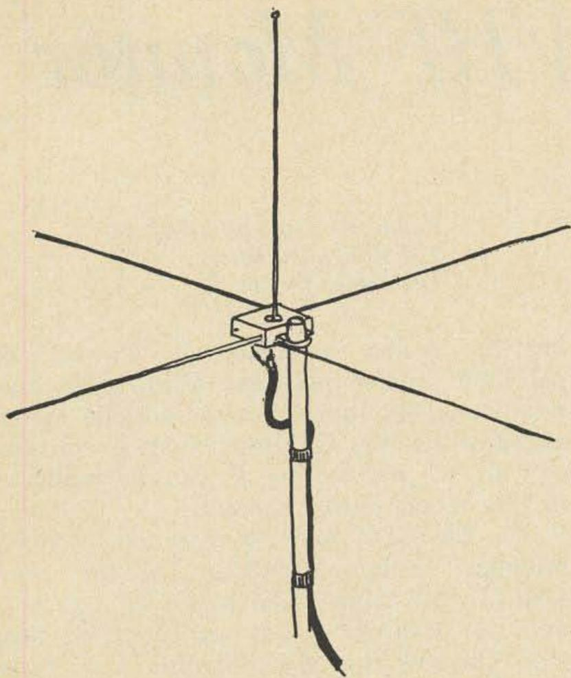
Fig. 2. The completed ground plane.
