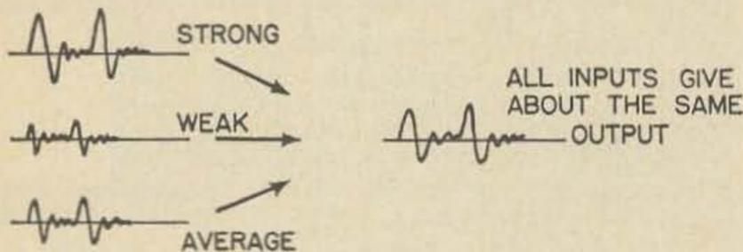
Fig. 1. AVC system adjusts system gain for a roughly fixed output voltage, independent of changes of input amplitude.
