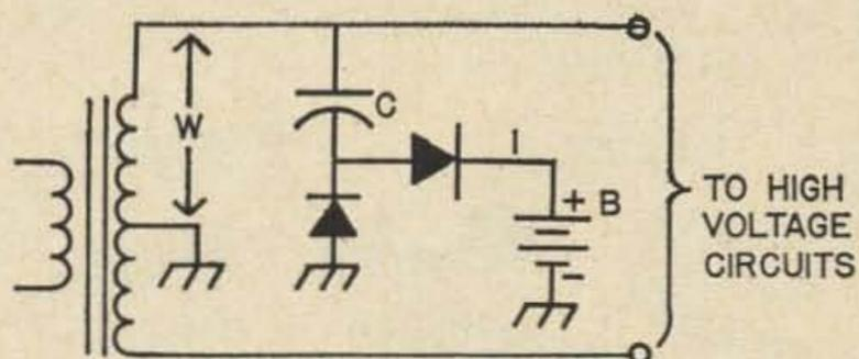
Fig. 4. Charging from a high-voltage transformer.
