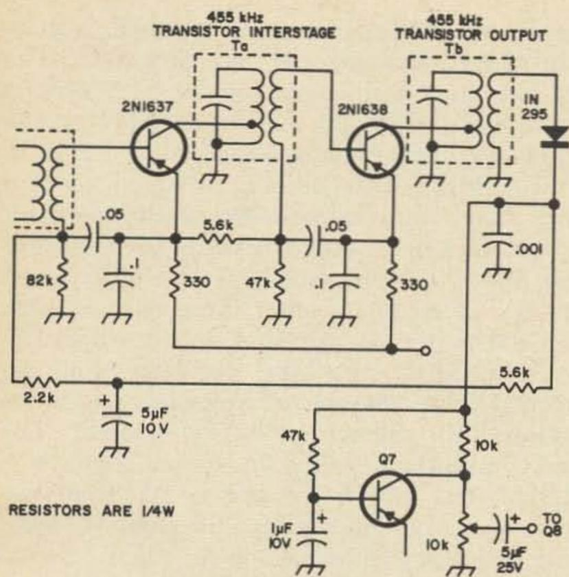
Fig. 3. Optional 455 kHz *If* Strip to replace module.
