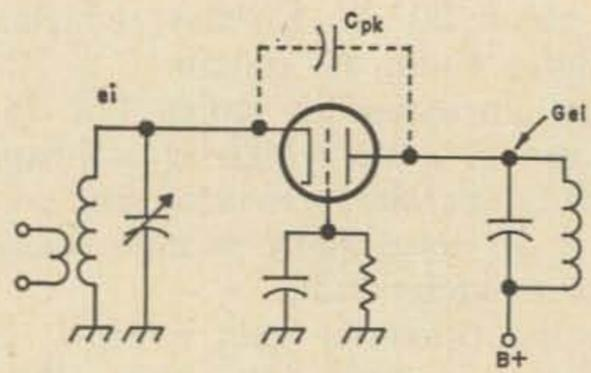
Fig. 2. Grounded grid circuit.
