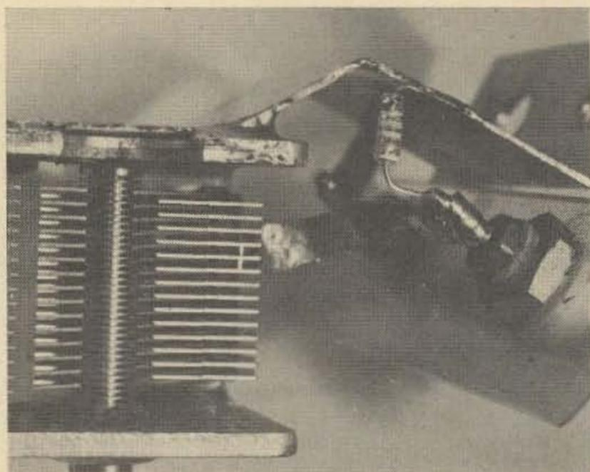
Inside view of mounting of diode and straps connecting the binding posts to the capacitor.
