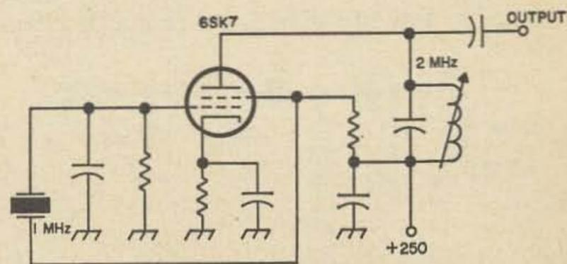
Fig. 3. Second conversion oscillator.
