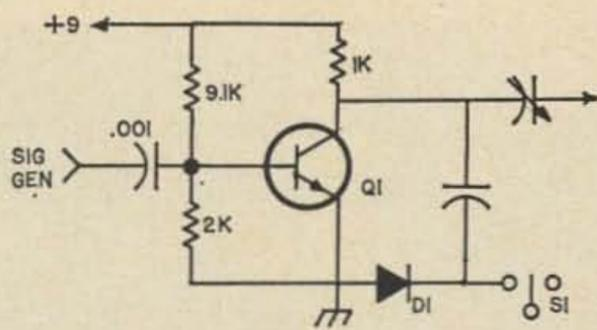
Fig. 5. Common emitter amplifier.
