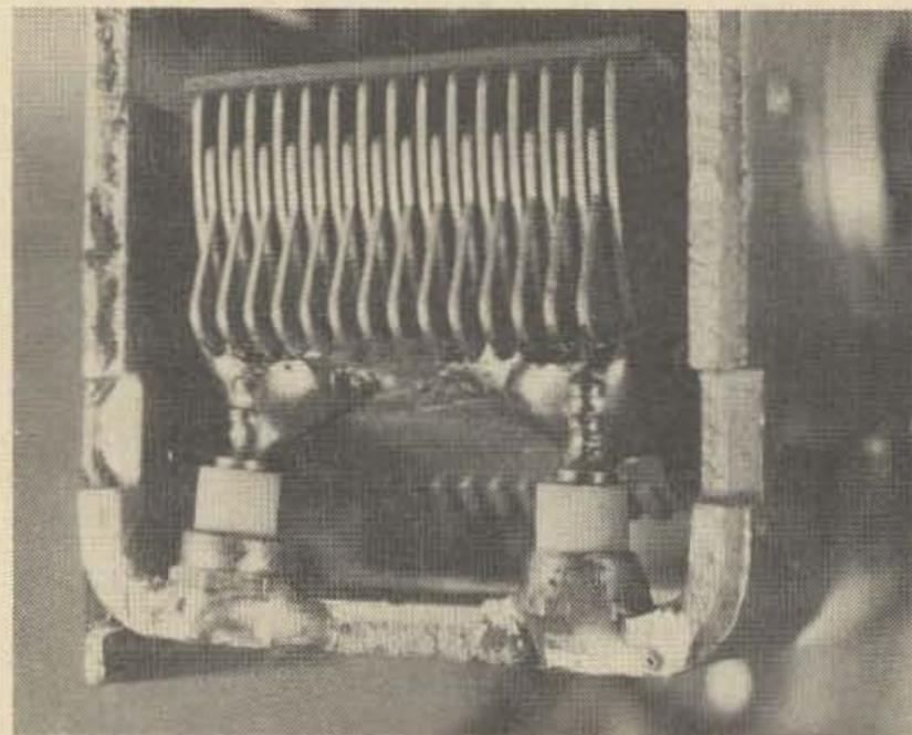
Inside view of variable capacitor (C3) showing the two ceramic standoffs for support of the stator.
