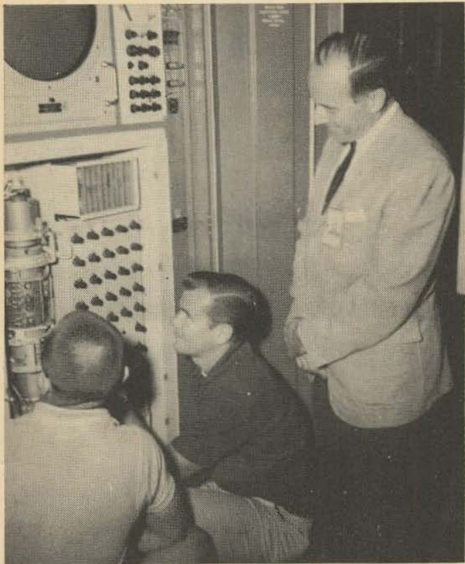
Looking at some of the more complex electronics gear. This is a system that adds maps to the radar display, and transmits the appropriate part of the resulting image to one of the radar repeated consoles.
