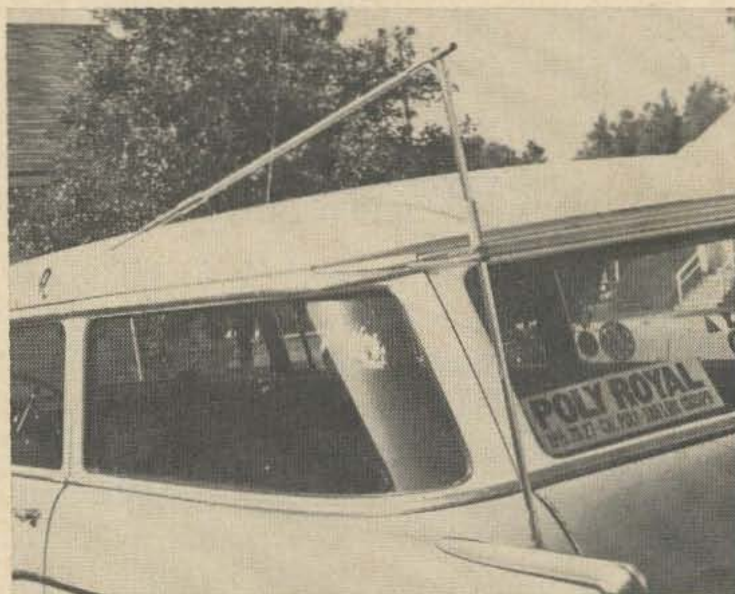
The advantages of a collapsible whip antenna are many. You may want to reinforce the whip to halt wild swaying when cornering by using an insulated brace mounted on the car body.
