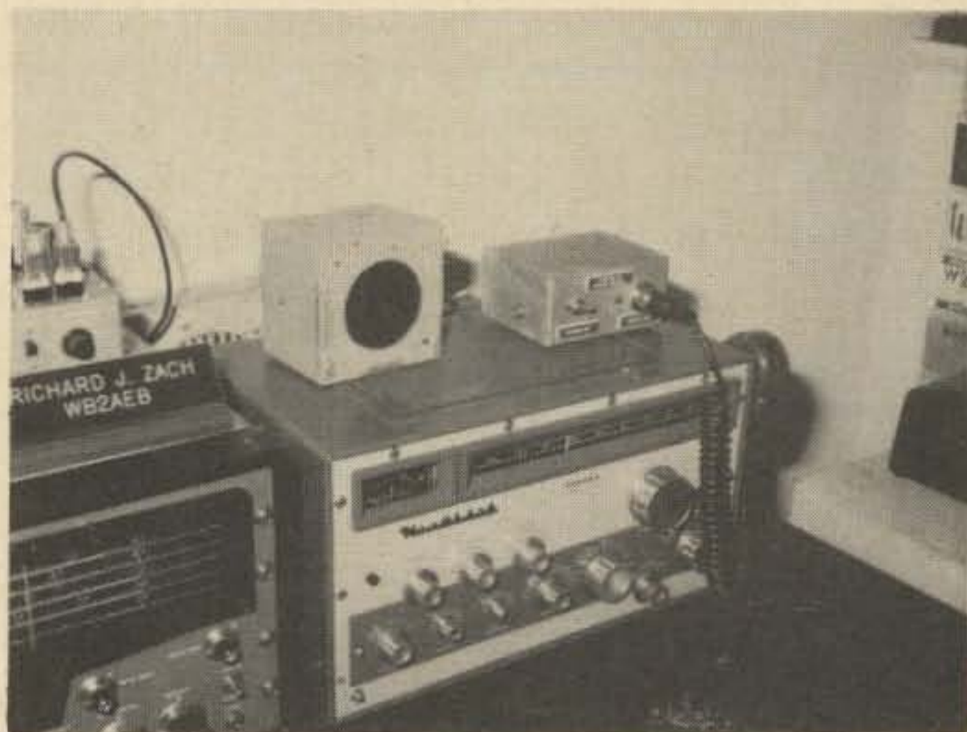
The remote unit can be tucked into even the most crowded shack. Note remote speaker muting switch (quite handy).
