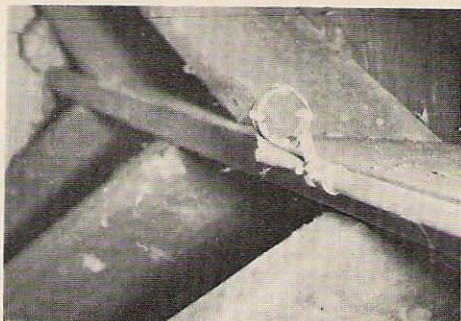
Fig. 9. Coil mounted on antenna element.
