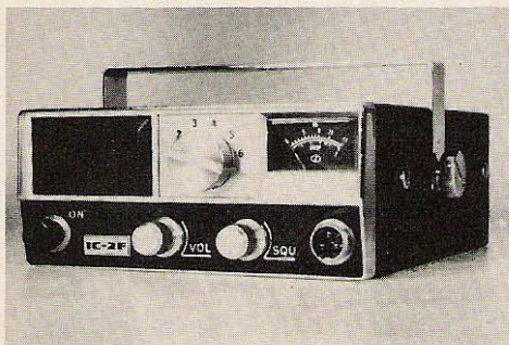
An act that's hard to follow. The Varitronics import, Model IC-2F, is a compact unit that combines transistors and ICs, packs a 10W punch, and includes circuit that shuts down rf output when the vswr on the antenna gets uncomfortably high.
