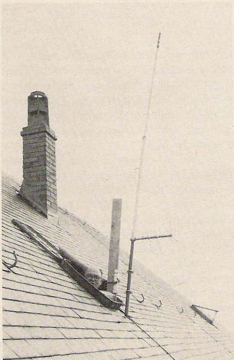
The Mini Products C4 multiband coaxial vertical dipole on the Hotel Meyer at Beaufort from which G3BID/LX radiated, with the head of G3BID visible in the skylight.
