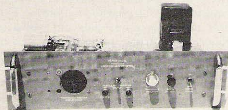
The controls from left to right are memory select, speed control, audio volume, power. The speaker is at the far left, and two power supplies are mounted on the top.
