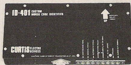
The Curtis ID package. The terminal strip gives access to all control, voltage and ground points needed for fully automatic operation.
