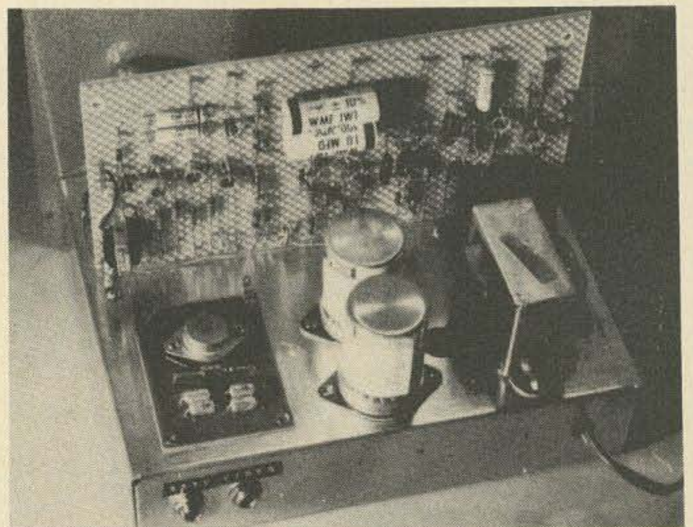
Fig. 4. Interior view of the completed SSTV test generator. Front panel controls (not shown) include power, function selector (S1), horizontal frequency, and the grey scale adjust (R1). The remaining pots are mounted on the chassis between the circuit board and the front panel. The rear portion of the chassis contains power supply components. The small circuit board includes bridge rectifier diodes and a zener and regulating transistor.
