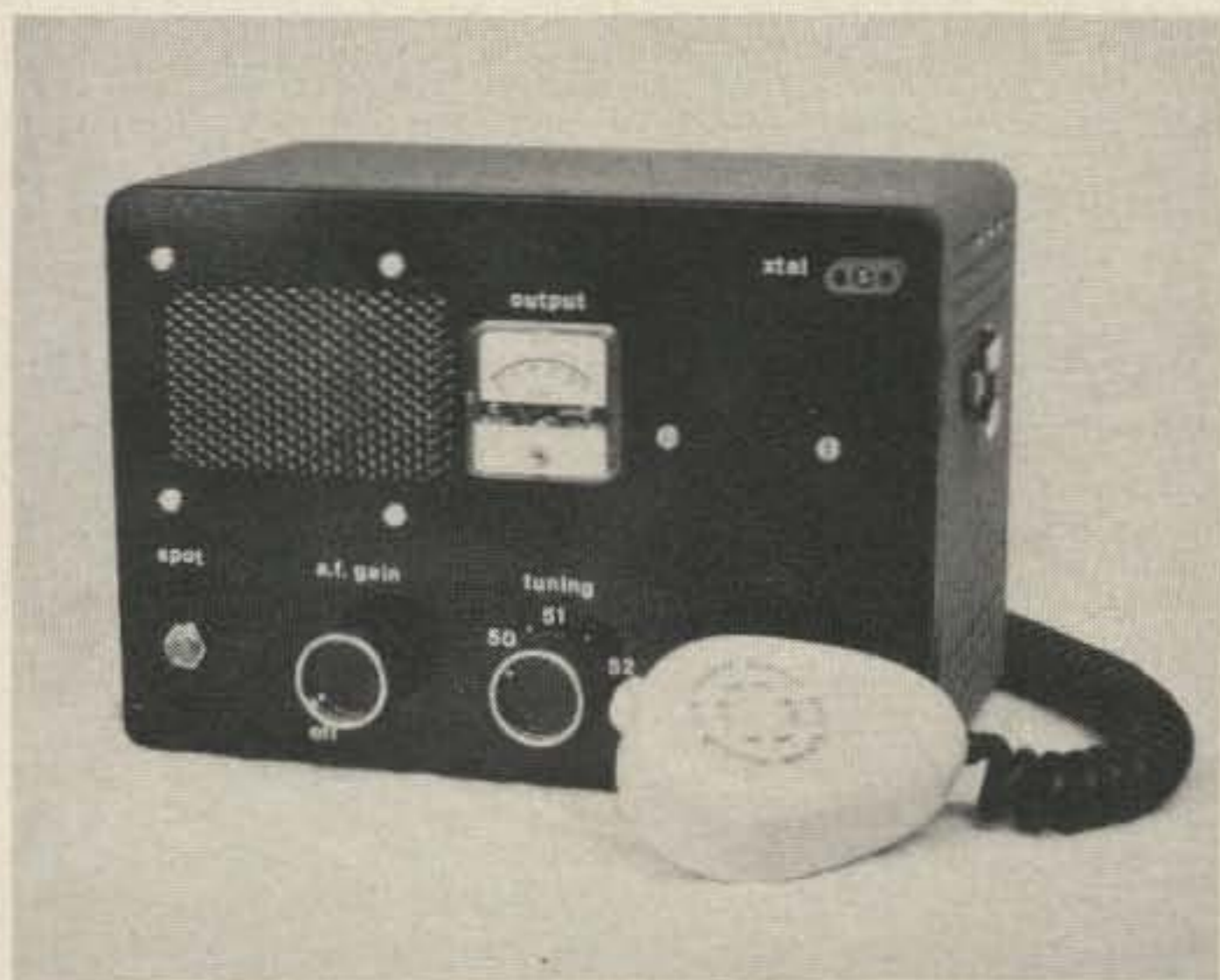
Author's "Sixer" ready for mobile operation. New panel is not essential but helps to cover up hole left by removed transmit-receive switch. Note new tuning scale.
