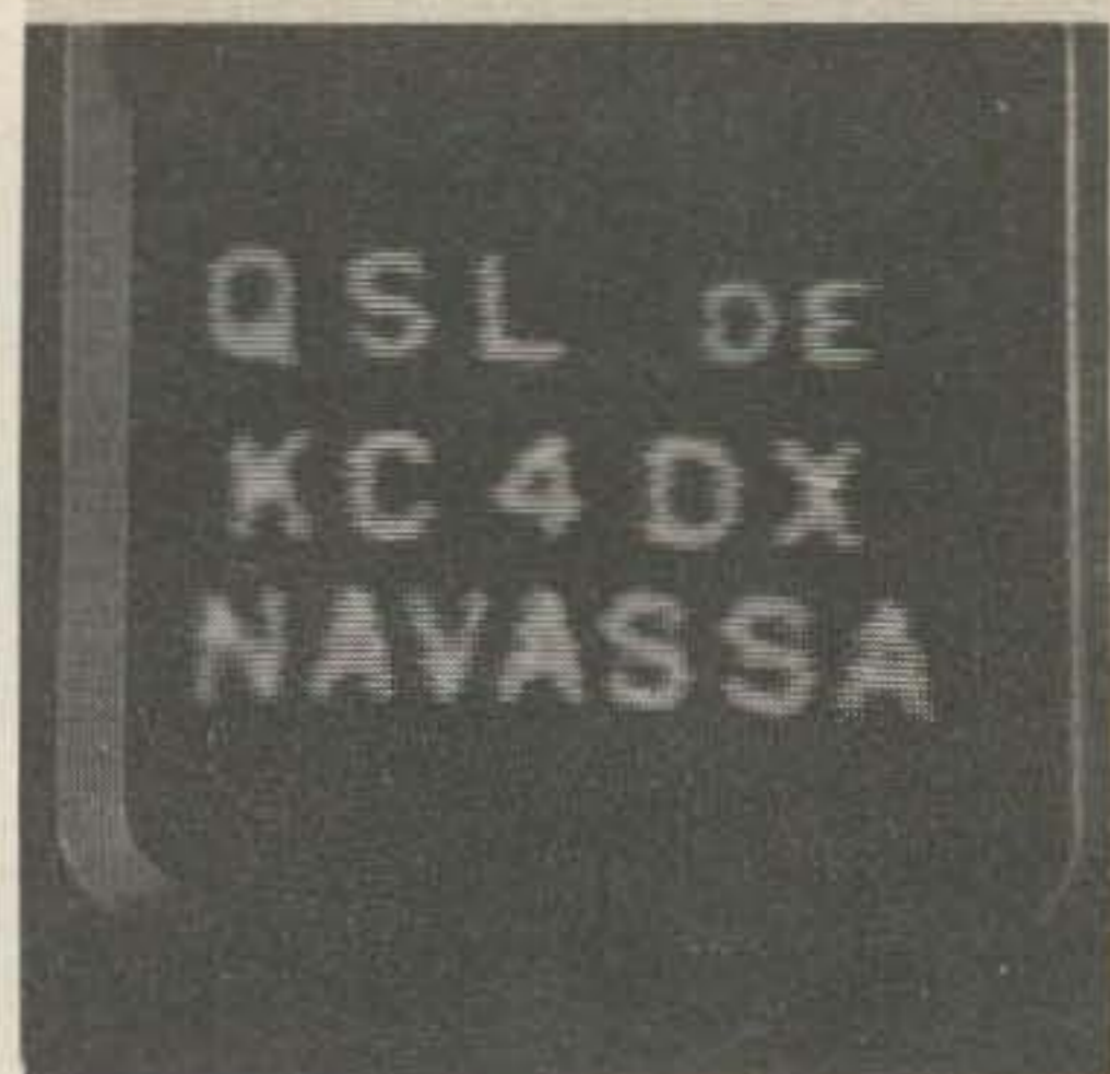
Slow scan television QSL sent from Navassa via a $17 cassette tape recorder and received by W8YEK and photographed from his monitor. The el cheapo battery operated recorder does result in slightly quivery letters.
