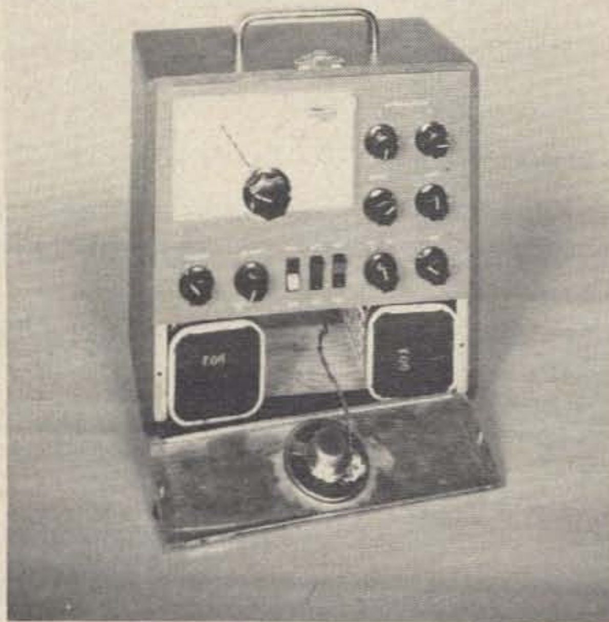
Two front views of the transceiver, one showing battery compartment behind loudspeaker panel. Note how panel space is conserved by placing SWR meter within dial assembly.
