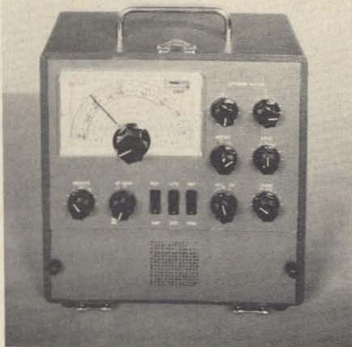
Two front views of the transceiver, one showing battery compartment behind loudspeaker panel. Note how panel space is conserved by placing SWR meter within dial assembly.
