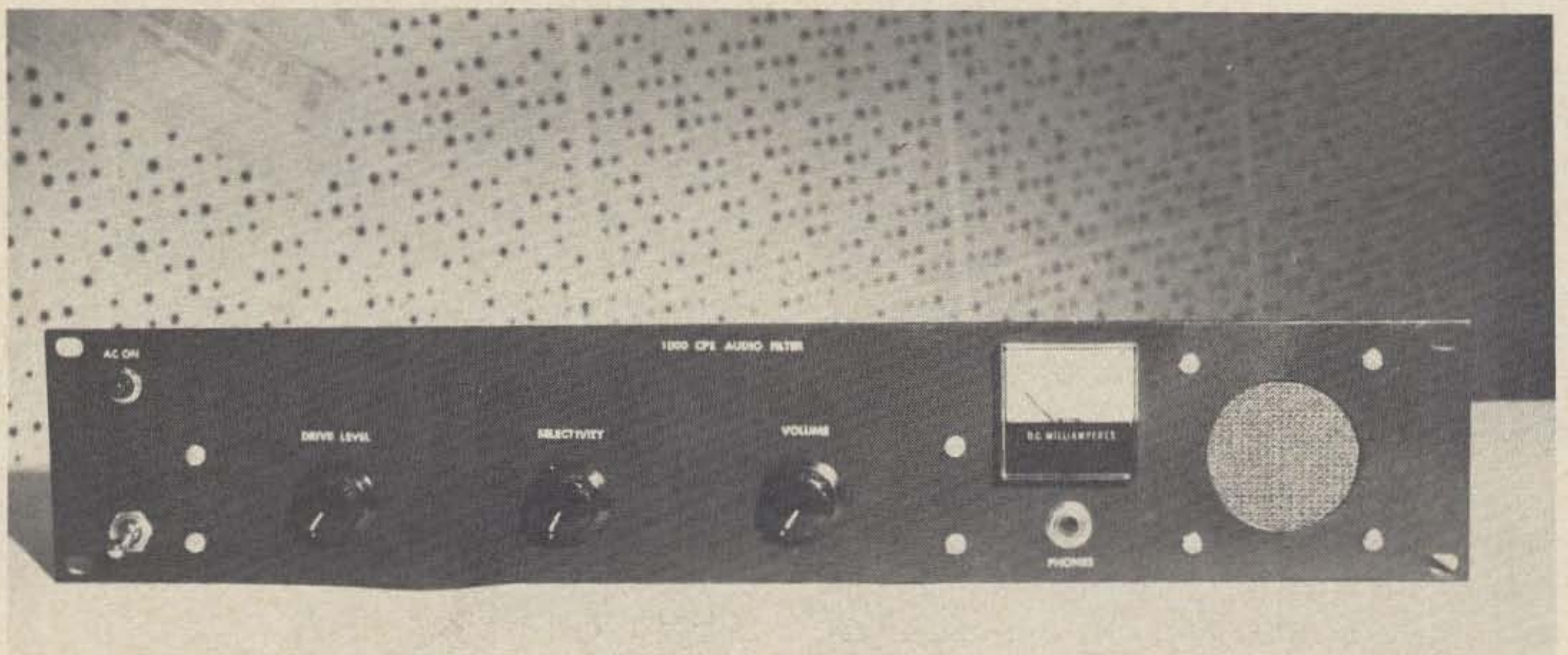
The filter can be assembled for rack mounting as shown or in its own box as a receiver accessory.
