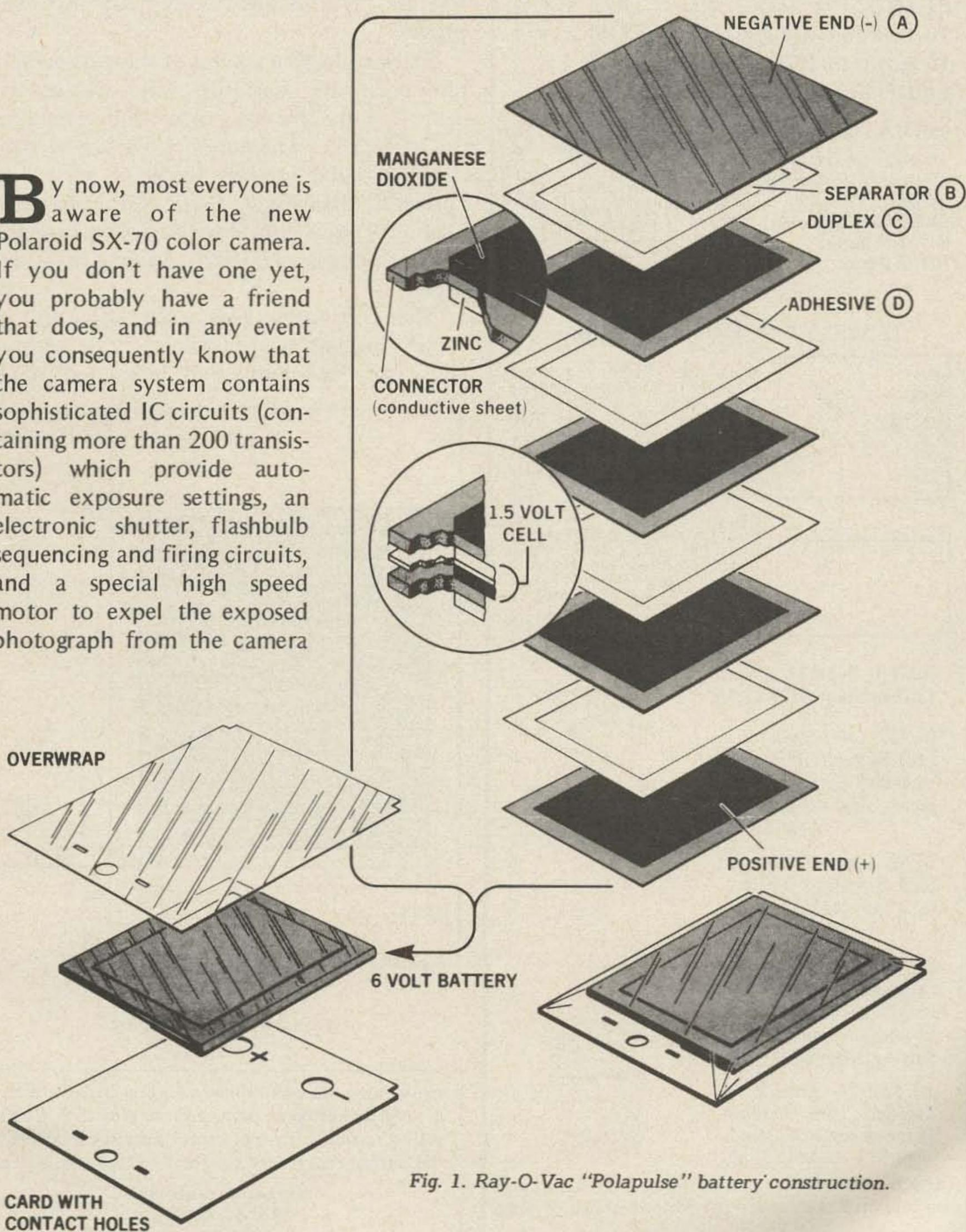
Fig. 1. Ray-O-Vac "Polapulse" battery construction.
