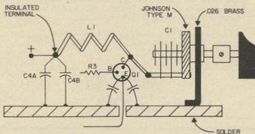
Fig. 5. 432 MHz amplifier using coil and capacitor tuning. Side view, layout of rf components.
