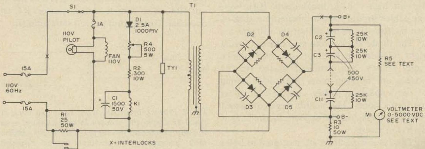
Fig. 1. Schematic of the 3000V power supply. The diode stacks D2–D5 are constructed of 8–2.5A 1000 PIV series connected diodes each. Shunted across each diode is a 470K 1W resistor and a .01 1000V disc capacitor. C2–C11 should be 500  $\mu$ F with a minimum voltage rating of 450V dc. K1 is a P&B type PR3DY, 24V dc coil with 25 amp contacts. T1 has a 2200V rms secondary with a 500 mA minimum rating. The thyrector is a G.E. 6R520SP4B4.
