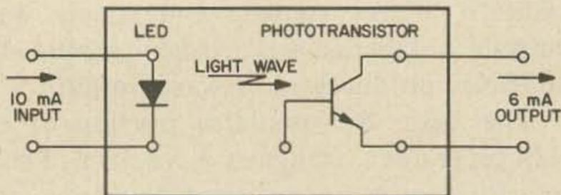
Fig. 2. Internal circuit of optical coupler IC. The input and output devices are completely isolated from each other. 10 mA through the light emitting diode will produce a current flow of about 6 mA from collector to emitter of the phototransistor.
