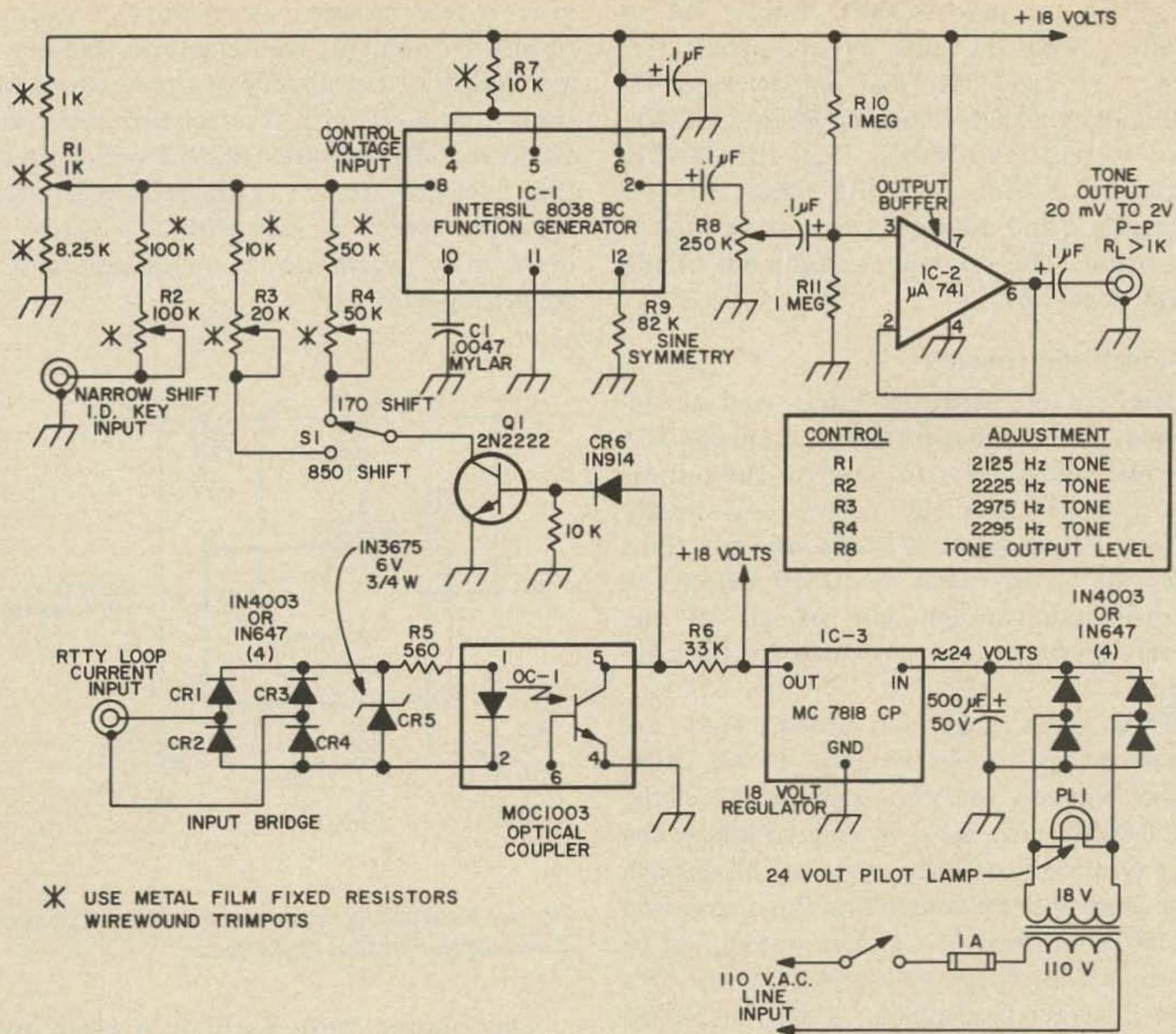
Fig. 3. Circuit schematic of the universal AFSK generator.
