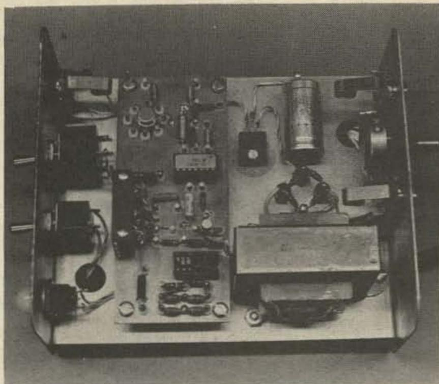
Interior view of the AFSK generator. The tone frequency adjustment pots are positioned so that they may be adjusted through the vent holes in the side of the case. The tone output and narrow shift key jacks located on the rear panel with the tone level adjustment pot.
