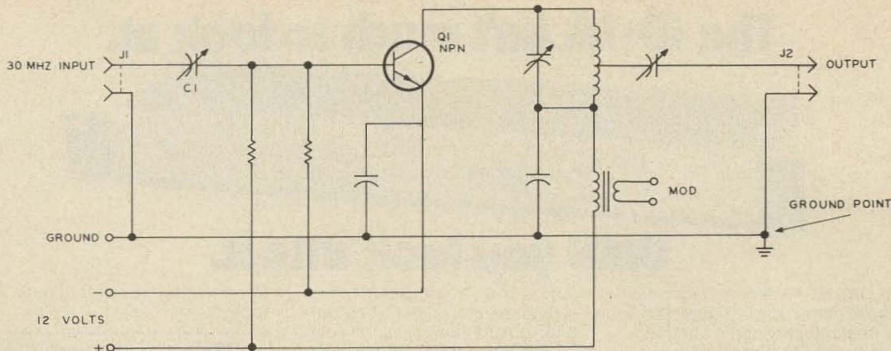
Fig. 2. Test circuit, 30 MHz region. Note. The "ground" point may be connected to either the positive or negative battery terminal, or left open dc-wise.
