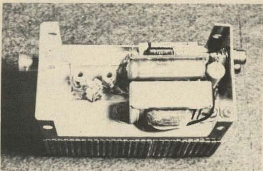
*Bottom view of transmitter showing mounting of audio board and modulation transformer. Capacitor at extreme right near power connector is 100  $\mu\text{F}$  unit across power input used to provide good filtering and low impedance when batteries are used. Parts layout is not critical here but try to keep audio stages away from final rf stage as much as possible to avoid rf pick up.*
