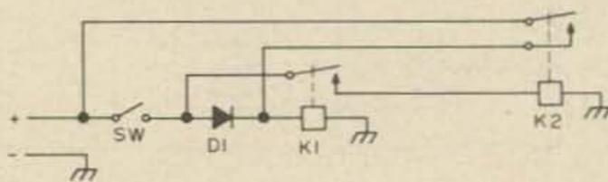
K1 on first and off last. K2 on last and off first. Handy for Pentode or Tetrode power amplifiers where K1 controls plate volts and K2 controls screen volts - overload dekeying, etc. Thanks W8UFN.
