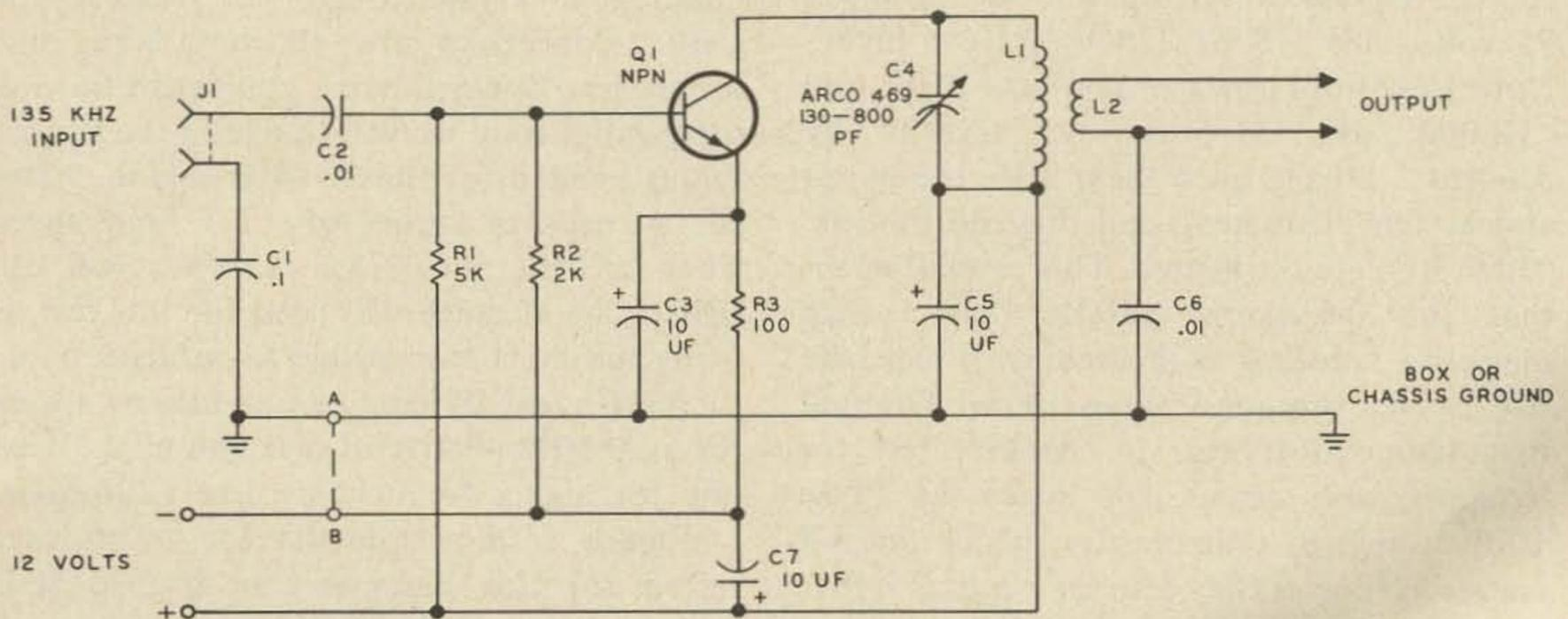
Fig. 1. VLF test circuit. I-f stage, 135 kHz.
