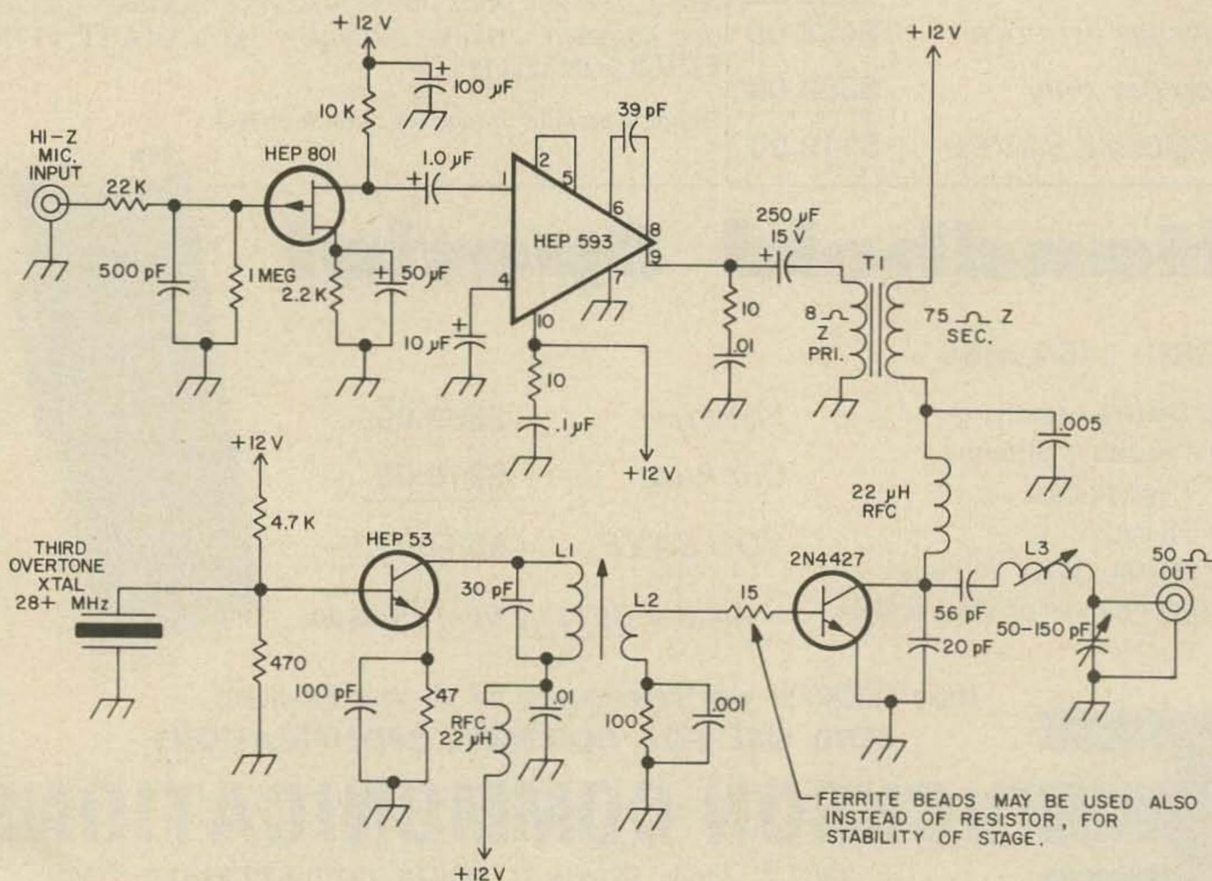
Fig. 1. Schematic of "Little Bill" transmitter. L1 - 13 turns No.28 P.E. CW, L2 = 2 turns link on cold end, L3 = 13 turns No.28 P.E. C.W.. All coils close wound on 6 mm diameter slug-tuned ceramic forms.
