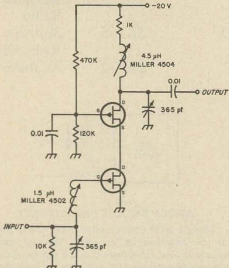
This 30 MHz if stage uses two FET's connected in the cascode arrangement to provide 20 dB gain without neutralization; the bandwidth is 4 MHz. Both FET's in this circuit are 2N3819, MPF105 or TIS34. With a negative supply voltage, the 2N4360 or TIM12 would be suitable.
