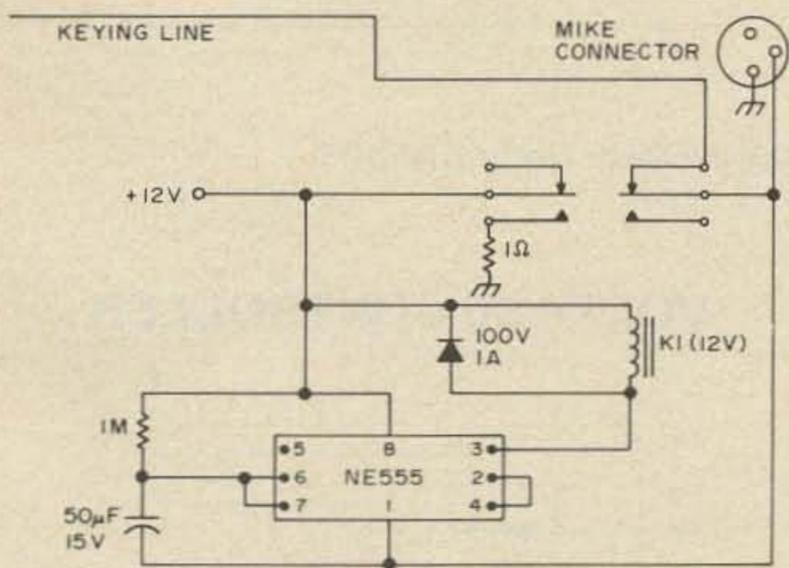
This circuit is designed to timeout your rig before it times out the repeater. It uses a simple 1 minute 59 second timer. It is shown wired for a TR22 but can easily be modified to work with any rig. Total cost about \$5. From the 31/91 KaChunker.
