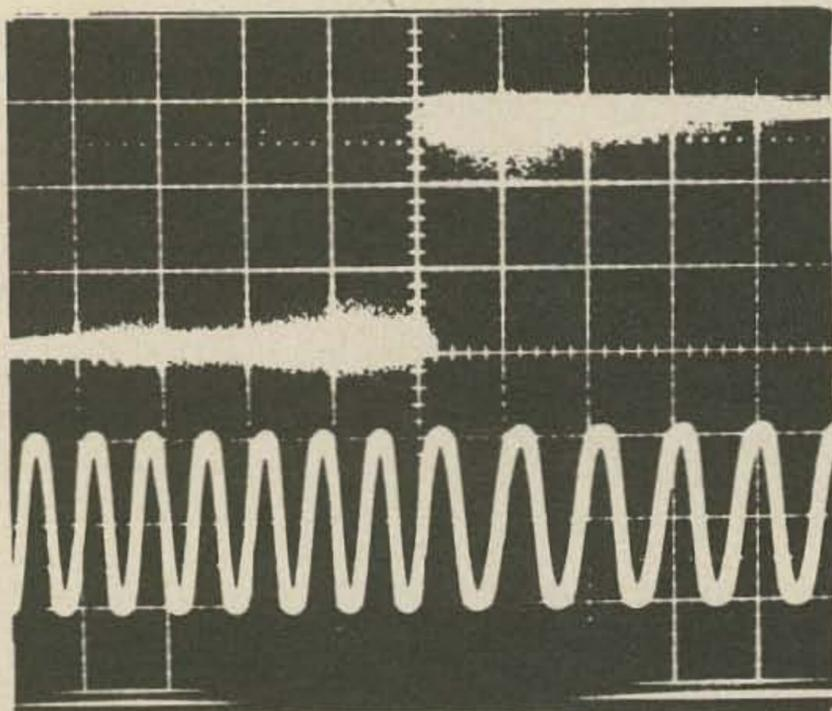
Frequency shift waveforms. Top trace shows input current waveform switching from SPACE to MARK. Bottom trace shows AFSK generator tone output switching from 2975 to 2125 Hz. No transients are present and the amplitude remains constant. Output is 2V peak to peak.
