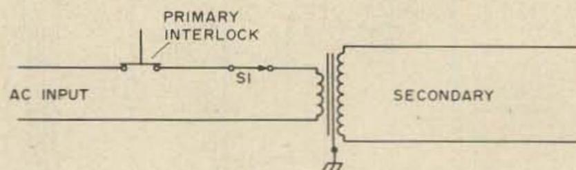
Fig. 2. Primary interlock. When removing cover or panel of supply the primary interlock should open thereby preventing the supply from being accidentally energized. A homebrew spring operated switch or commercial pressure switch works well. The primary interlock must have ample current carrying capability.
