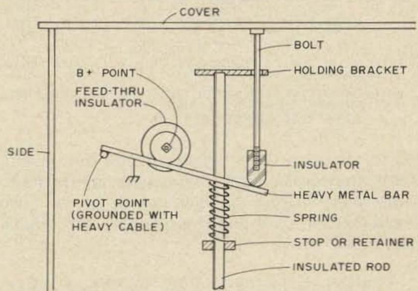
Fig. 3. Secondary interlock. Removing the cover permits the metal shorting bar to move up and contact the B+ point, thereby shorting any dangerous voltage to ground. As long as the cover is removed the B+ point will be grounded. This assembly must be mechanically strong and not subject to movement or bending.
