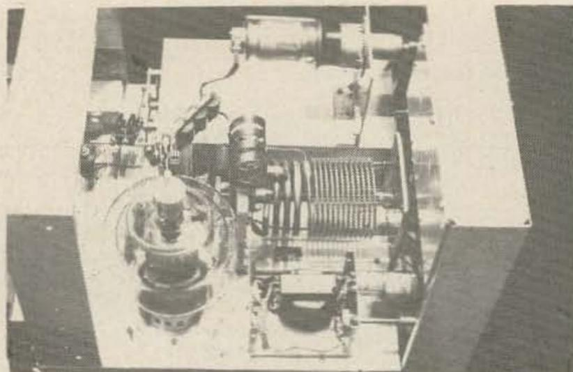
Looking down on amplifier's alc enclosure cover removed for photo. Note: also vacuum variable mount. Relative field strength enclosure and 2.5 mH rfc is located in upper left.
