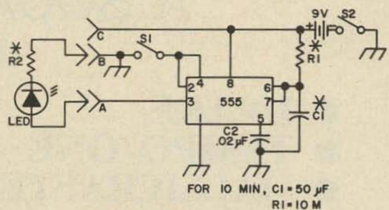
Fig. 1. Schematic of the 10-minute timer. See text for a discussion of R1, C1 and R2.
