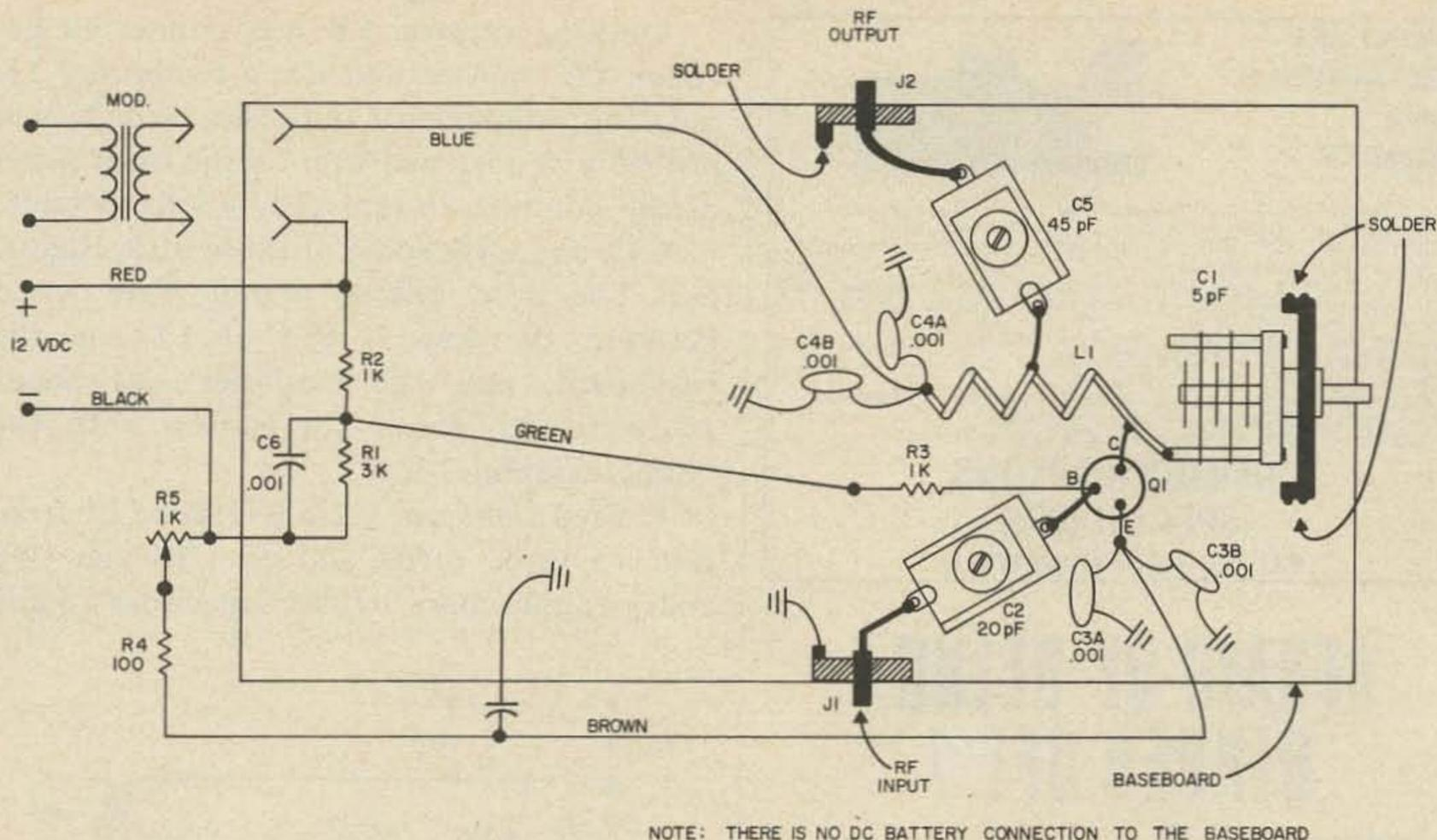
Fig. 4. 432 MHz amplifier using coil and capacitor. Top view.
