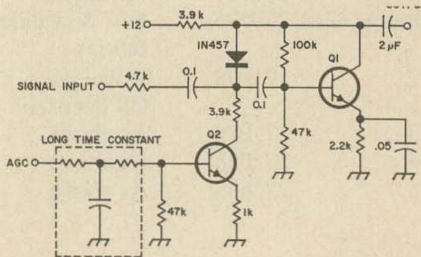
This super AGC circuit only requires two transistors to obtain up to 60 dB of control. Q1 and Q2 are 2N1613 or HEP-254.
