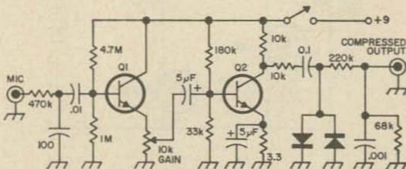
Two stage clipper/preamp will increase the talk power of your rig. Transistors Q1 and Q2 are 2N1304, 2N2926, 2N3391, SK3011, or HEP 54. The diodes are IN456 or HEP-158.
