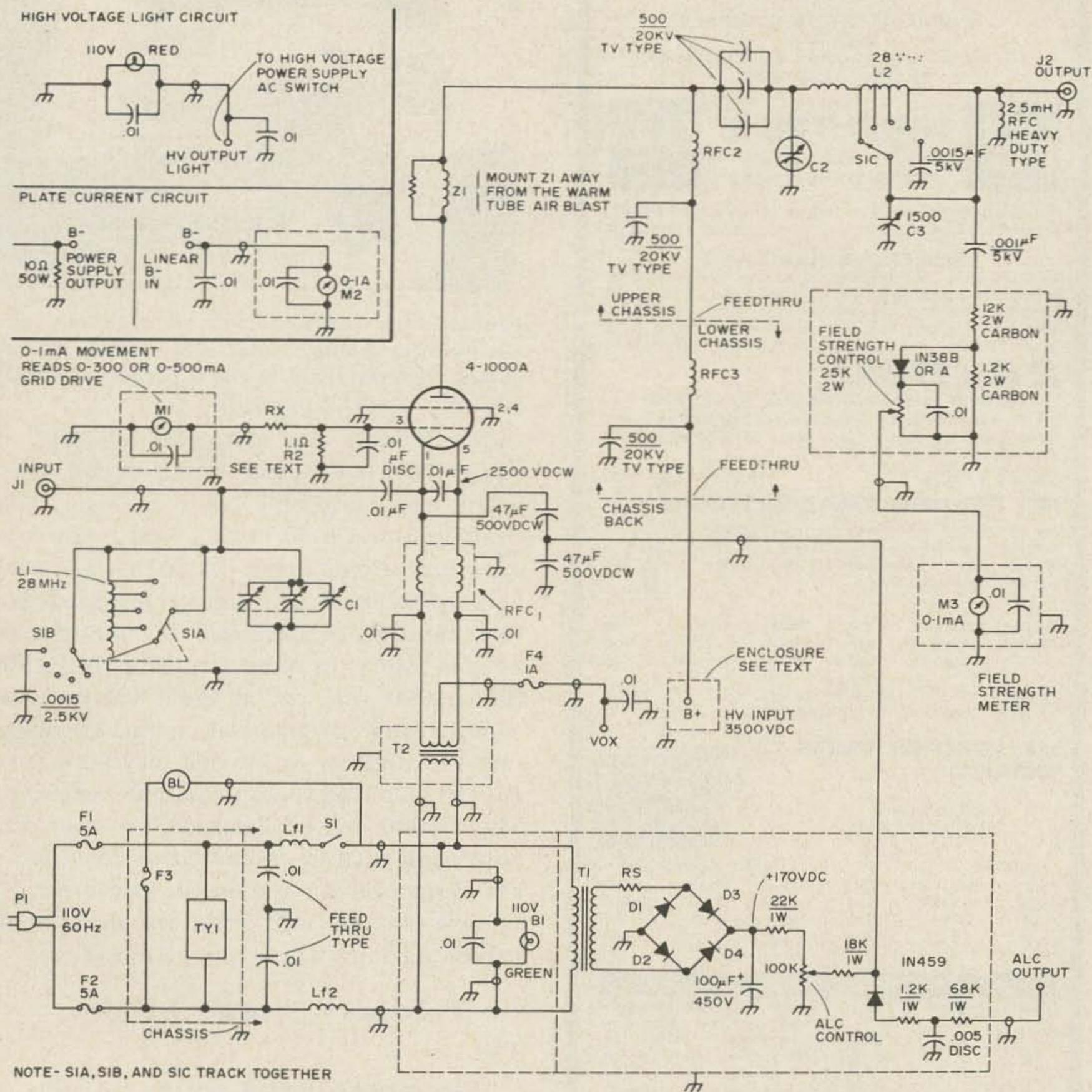
Schematic diagram of the modern 4-1000A, Class B, grounded grid, linear amplifier.
