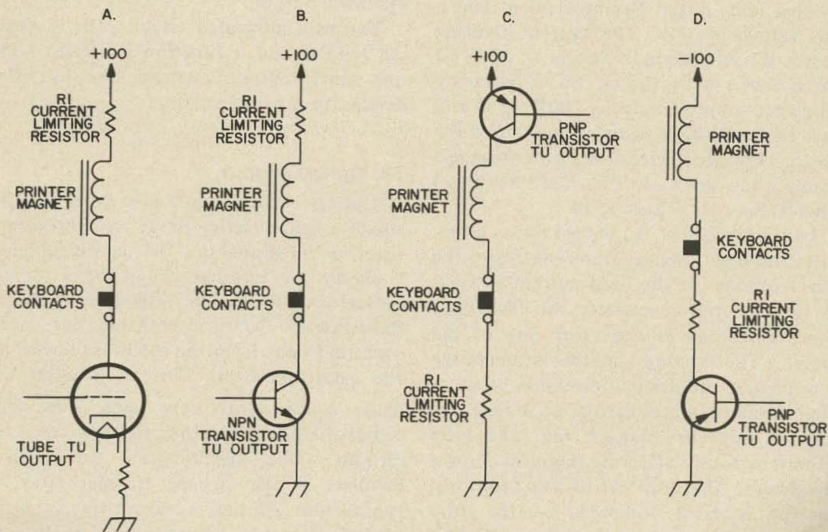
Fig. 1. Typical RTTY loop circuit: a - TU with tube output and positive loop supply. b - TU with NPN transistor output and positive loop supply. c - TU with PNP transistor output and positive loop supply. d - TU with PNP transistor output and negative loop supply.
