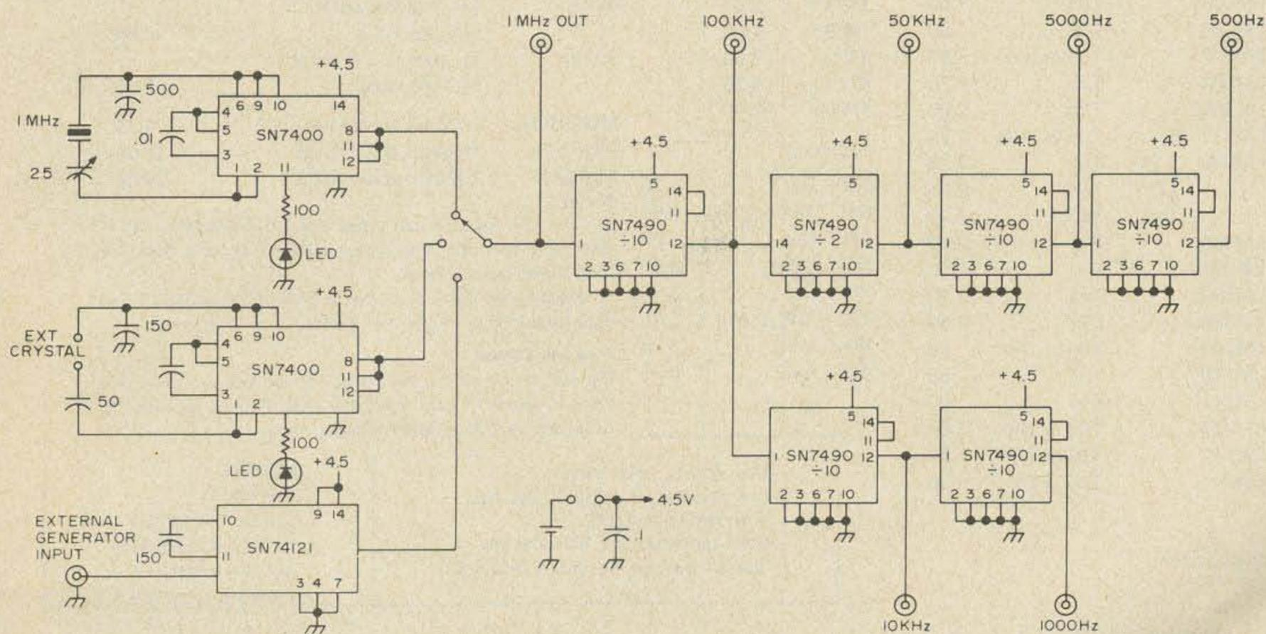
Fig. 1. Diagram of universal frequency generator. Output frequencies shown are for using 1 MHz oscillator.
