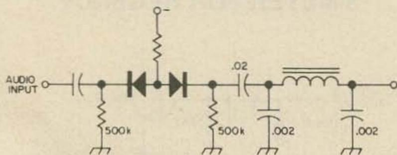
A good clipper for AM or FM use includes adjustable clipping level and a harmonic filter.
