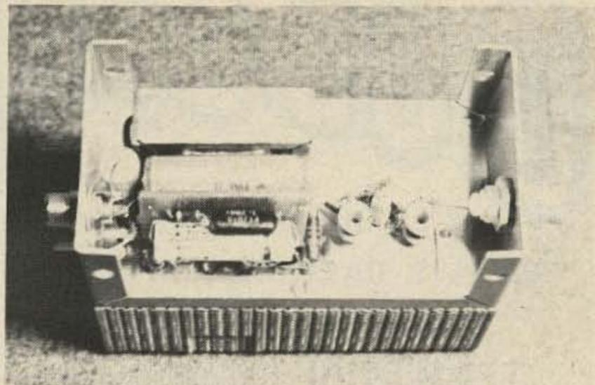
*Bottom view of transmitter showing parts placement. Note antenna connector on left apron to allow very short lead to pi-network. Photo shows double pi-network originally used but later revised to single pi output, see text. Modulator components shown on right side with board containing all audio parts except transformer which is fastened to box directly.*
