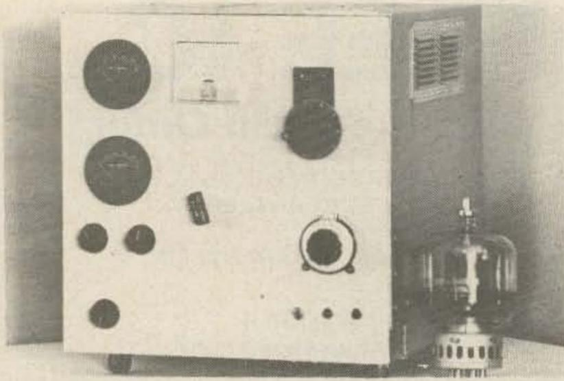
Front view. Meter upper left grid drive, lower left relative output, center plate current. Three controls in lower left. Alc far left, relative output sensitivity right, cathode tuning lower left. Front center control band switch. Upper right turns counter. Lower right loading control. Switch, on and off. Green filament light left. Red high voltage light right. Note: air vents on side.
