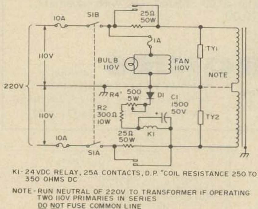
Fig. 4. Alternate 220V primary circuit for use with 220V transformers. The components are similar to those used in the original circuit except two thyrectors are used and the relay K1 is a double pole type.
