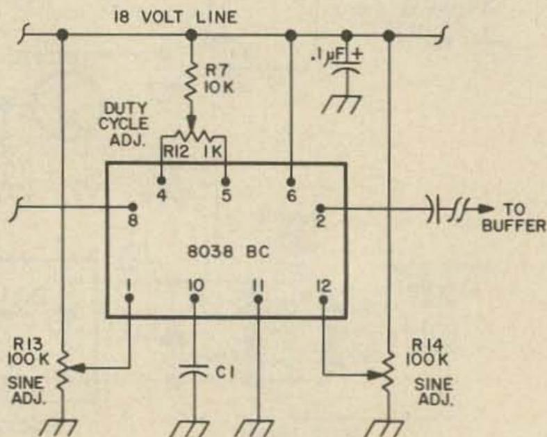
Fig. 4. Function generator with optional controls to reduce sine output distortion.
