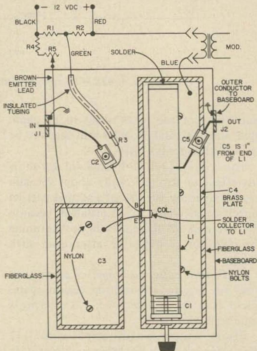
Fig. 6. "Super strapline" 432 MHz amplifier. Top view.
