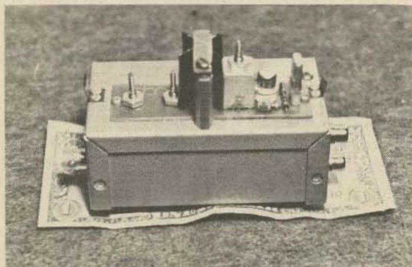
Top view of transmitter with shield cover removed to show general layout of components. Finned heatsink on final transistor is home made from aluminum sheet and painted flat black. Stand off supports small strip of plastic to hold heatsink in place and keeps transistor from being damaged if jarred accidentally. Crystal oscillator on right with its coil mounted in an old i-f can and amplifier on left with pi-network. Note small spring clips to hold shield cover in place on each end of mini-box.
