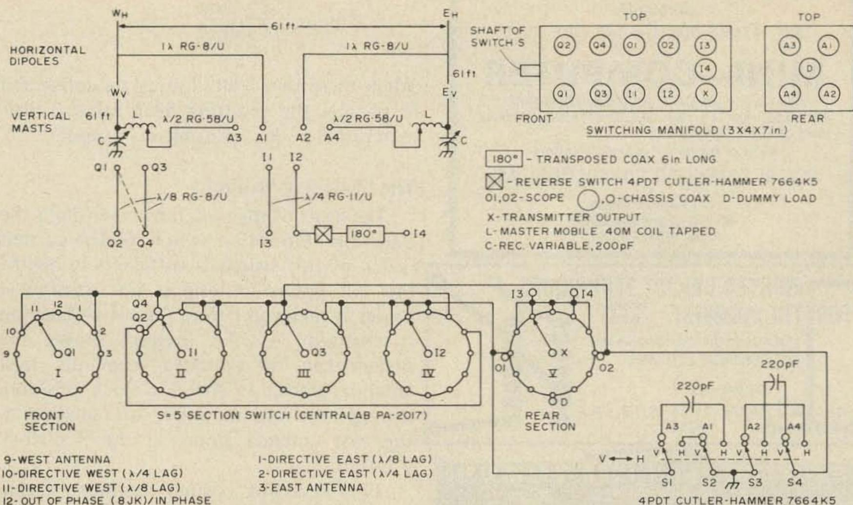
Fig. 1. Horizontal and vertical phased array circuitry. Only three switches need be used for instantaneous switching. See text for details.
