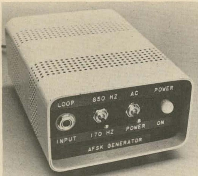
Front view of the AFSK generator. Controls include the shift selector switch and the power switch. The loop input jack is isolated from ground with shoulder washers.
