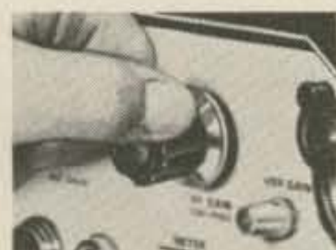
Built-in 100 kHz & 25 kHz calibrator. Keeps your dial scale accurate to 2 kHz.
