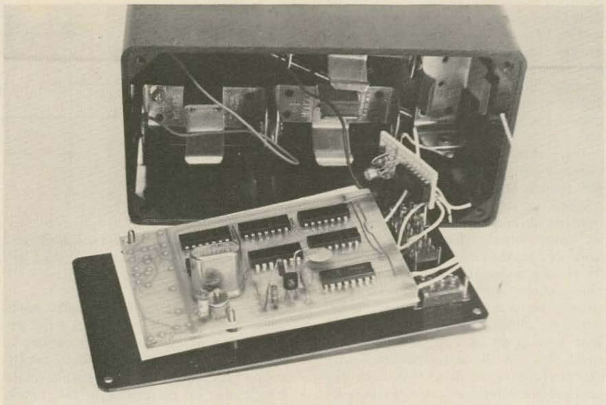
This shows how the timebase board is mounted. Note that there are no components at the top of the board. The top of the board is reserved for the power supply parts which are not used with the battery supply.
