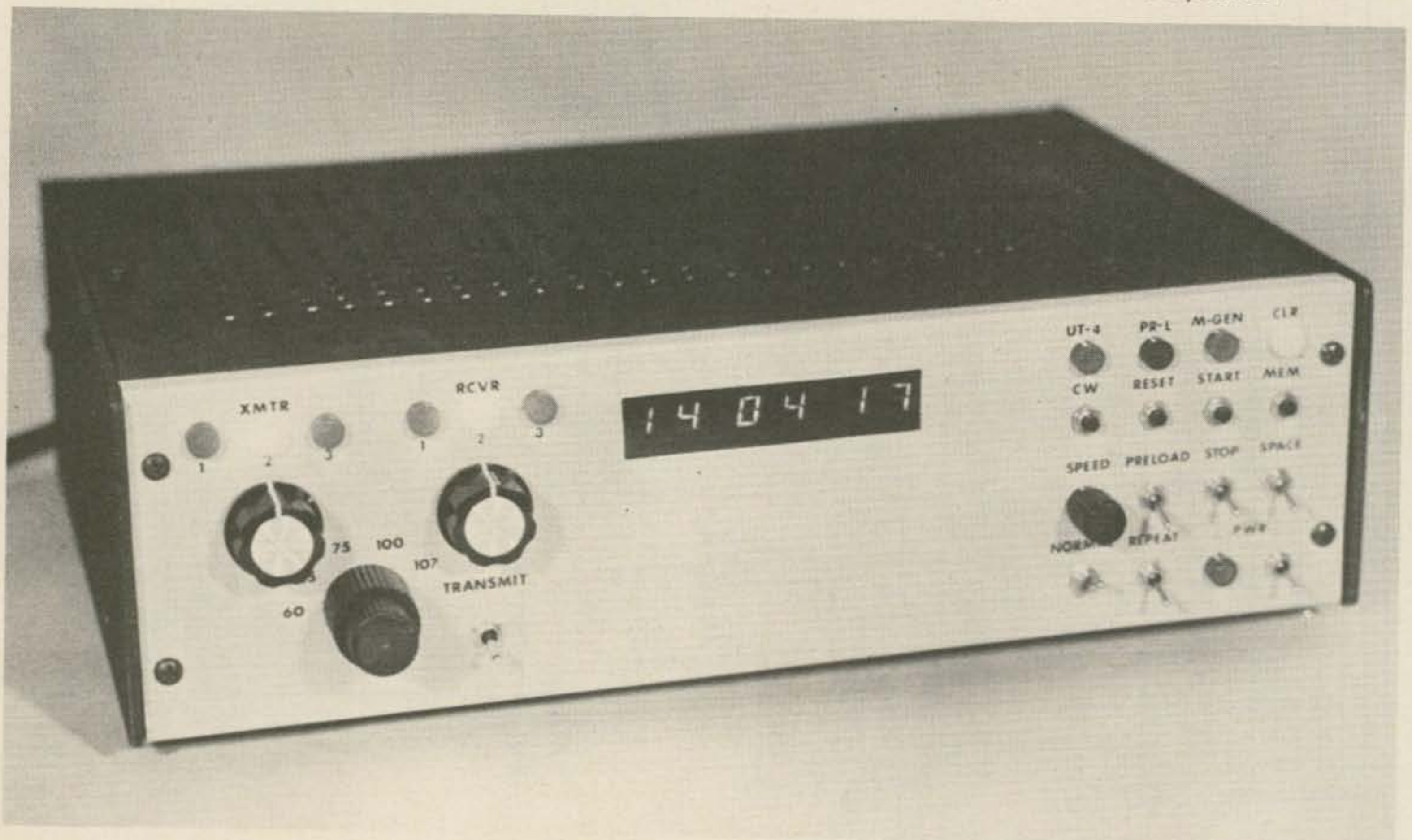
Completed clock. This control unit built by K1ZPX houses the DDTMG, a UT-4, the necessary power supply, and switching circuits to select interfaces to several receivers and transmitters.
