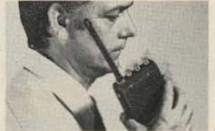
Flexible "rubber duckie" antenna, matched to transceiver, is included plus jack for external antenna.
