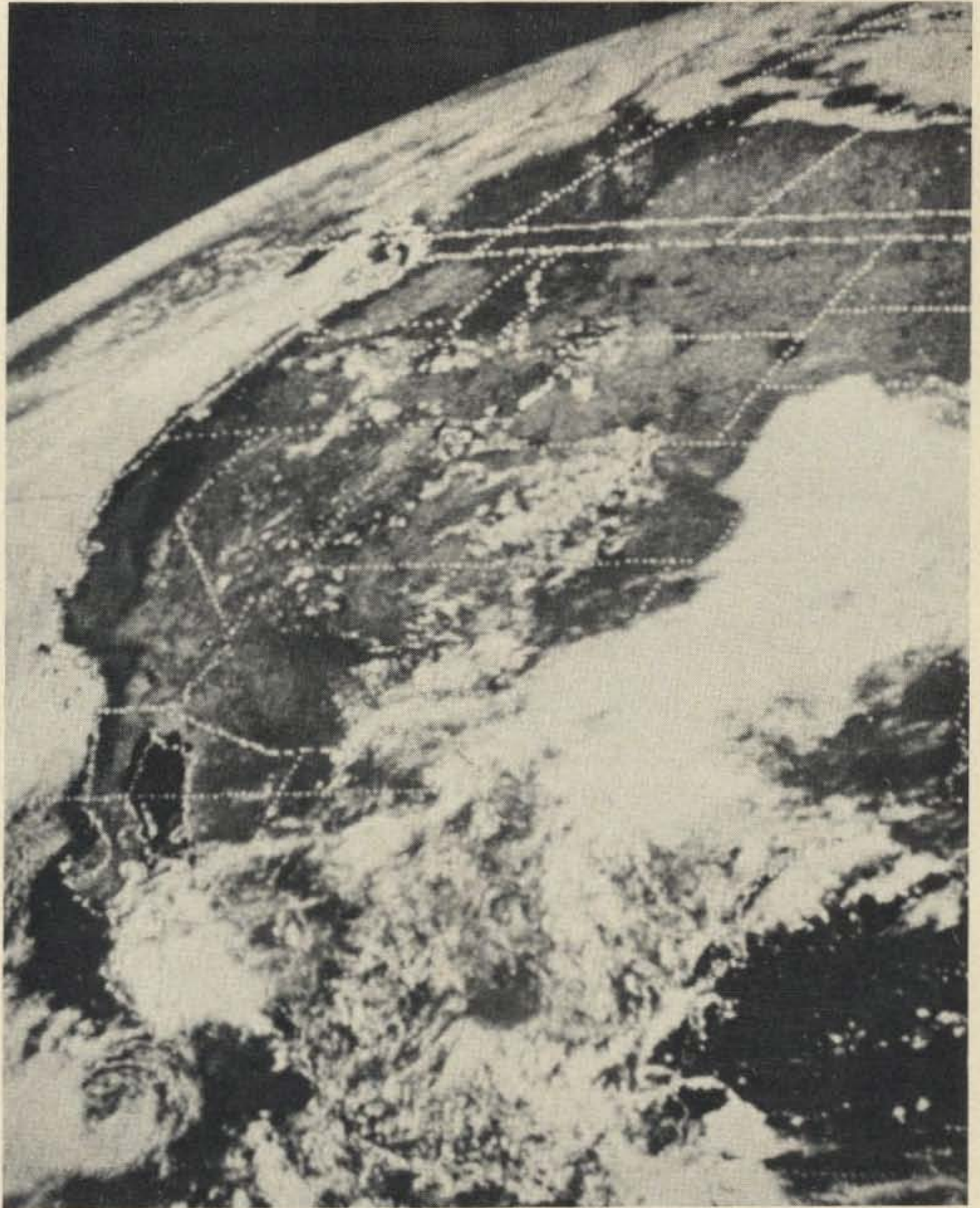
Photo 3. An example of an SMS S band (1691 MHz) WEFAX transmission as received and displayed by Roy Cawthon of Atlanta, Georgia. Such pictures are derived from the very high resolution spin scan radiometer on the spacecraft, which takes both visible and IR pictures of the full earth disc as seen by the satellite. The pictures are gridded on the ground and re-transmitted through the satellite. Operational versions of this series (GOES satellites) will transmit such pictures and a variety of other WEFAX products. The development of effective, low cost S band converters is one of the major challenges facing amateur satellite experimenters.
