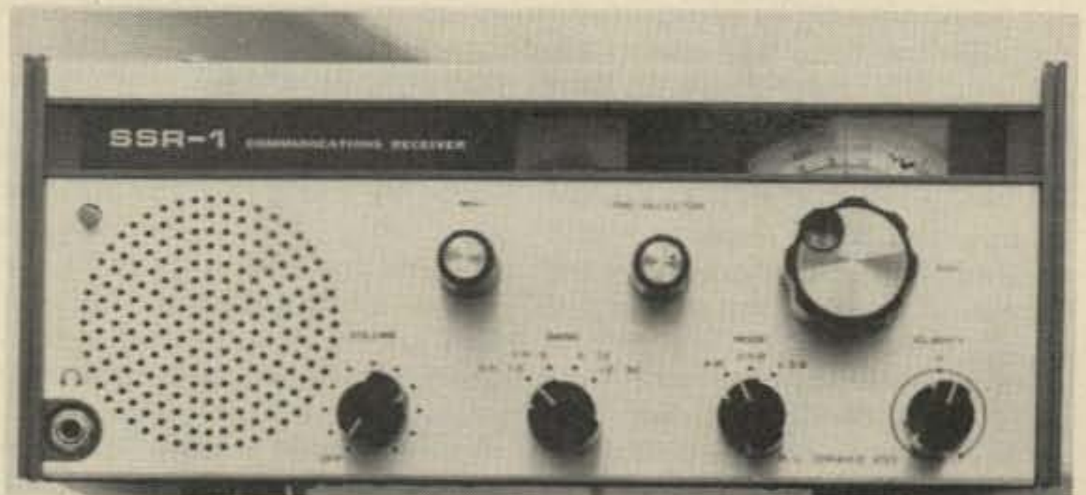
The Drake SSR-1 receiver, with a simple layout and 500 kHz through 30 MHz coverage.
