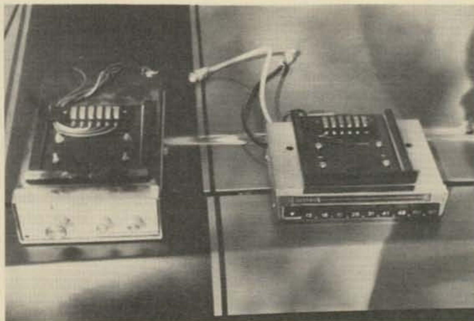
View showing slide mounts on the rig and SW converter.
