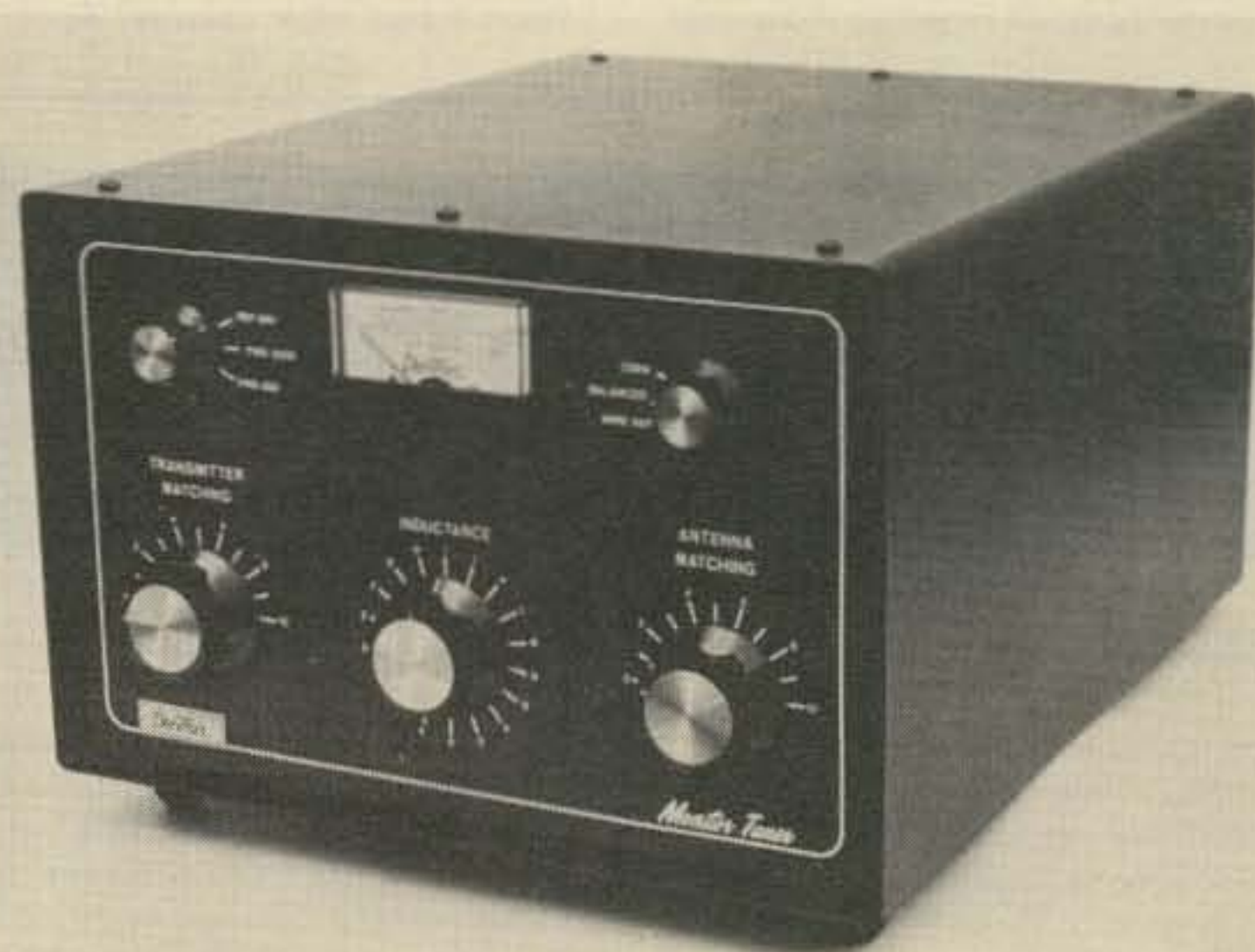
The Dentron Radio Monitor Tuner — basically the same unit as the Super Super Tuner, but with an swr/power meter built in.
