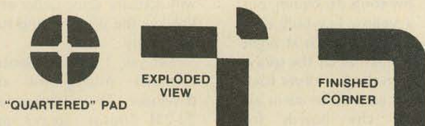
Fig. 2. Rounding the corners using cut pads.
