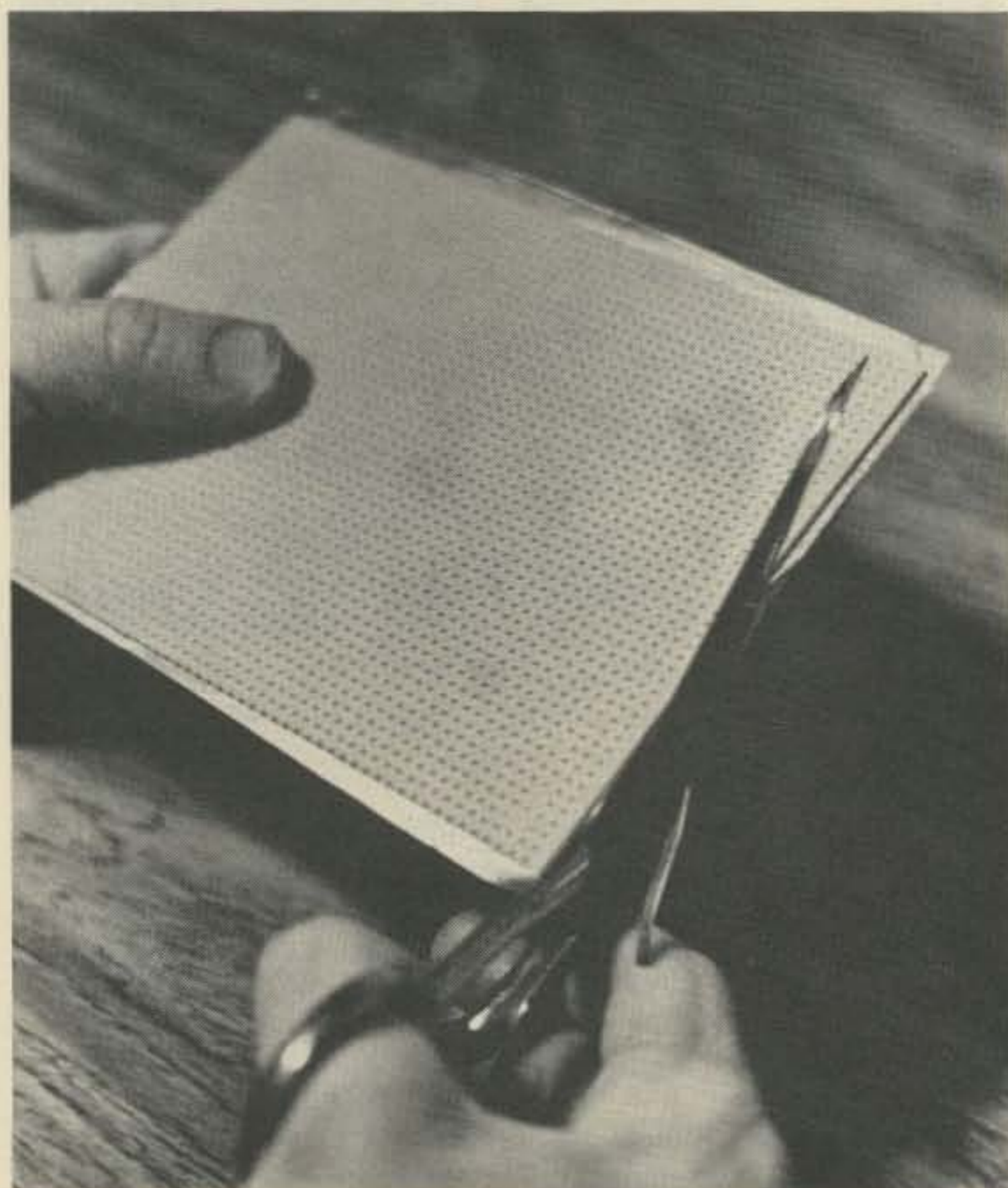
Fig. 6. As your final step, trim away any excess copper with a pair of scissors.
