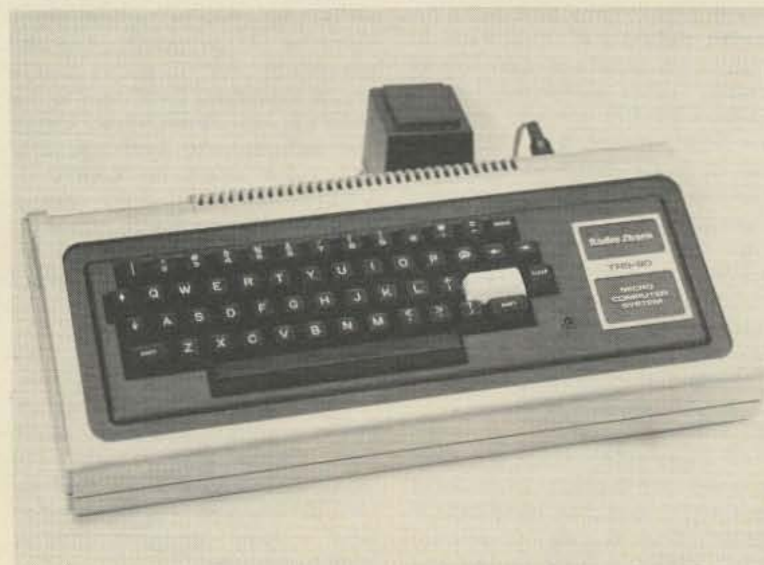
The new Radio Shack TRS-80 Microcomputer System features a built-in 53-key professional-type keyboard and one of the most advanced microprocessor chips available today, the Z-80.
