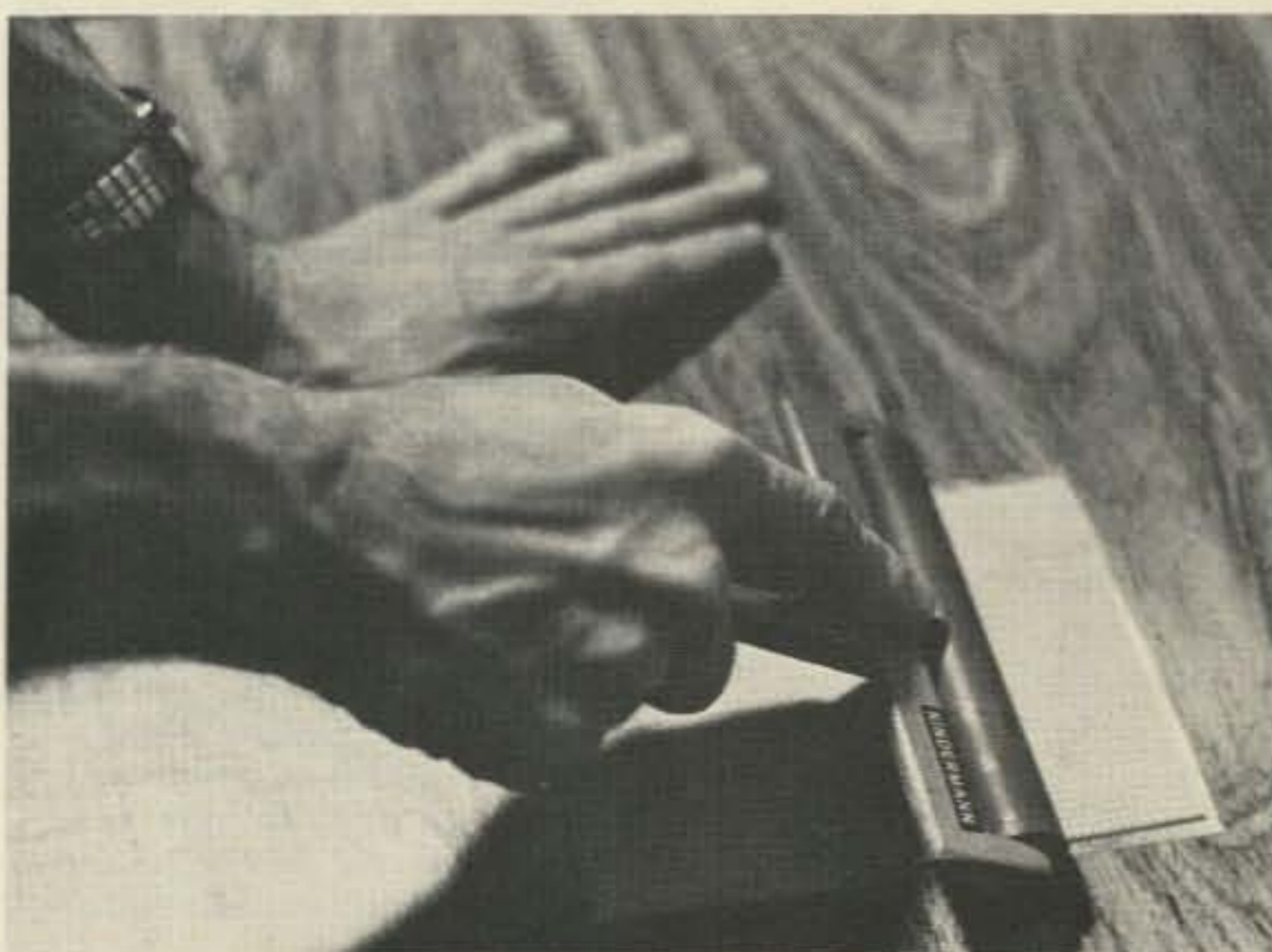
Fig. 5. I used a photographic roller to apply even, heavy pressure to the joined pieces, but you can use the palms of your hands.
