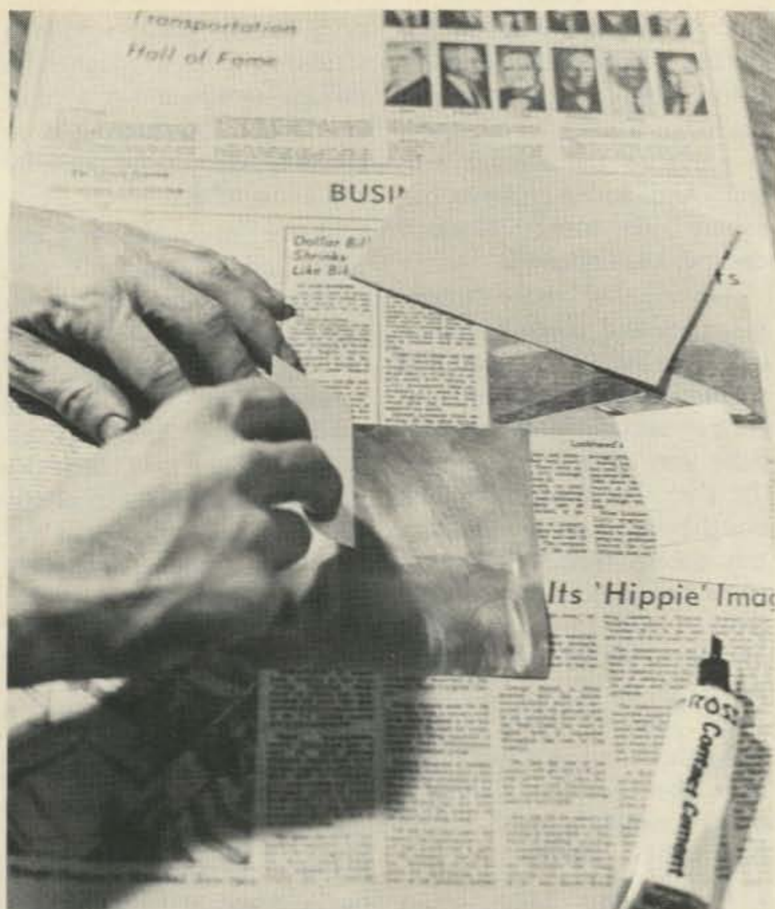
Fig. 3. Apply thin, even coats of contact cement to the copper and phenolic using small pieces of cardboard cut from a filing card.
