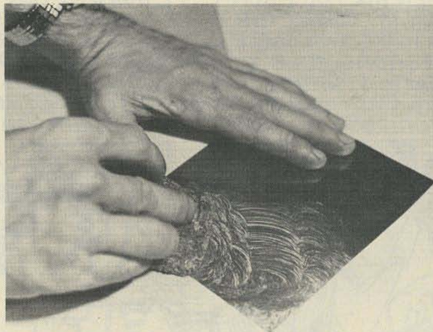
Fig. 2. Use the soap pad to thoroughly clean the surfaces of both the copper and the phenolic.
