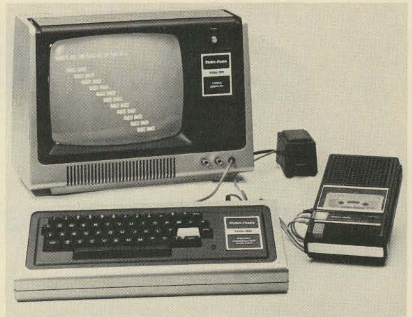
Radio Shack's complete TRS-80 Microcomputer System, consisting of a 53-key professional-type keyboard and microcomputer plus regulated power supply, computer-controlled data cassette recorder, and 12" video display monitor, is suitable for business, educational, and home applications. Available exclusively from Radio Shack stores and dealers, nationwide, for $599.95.
