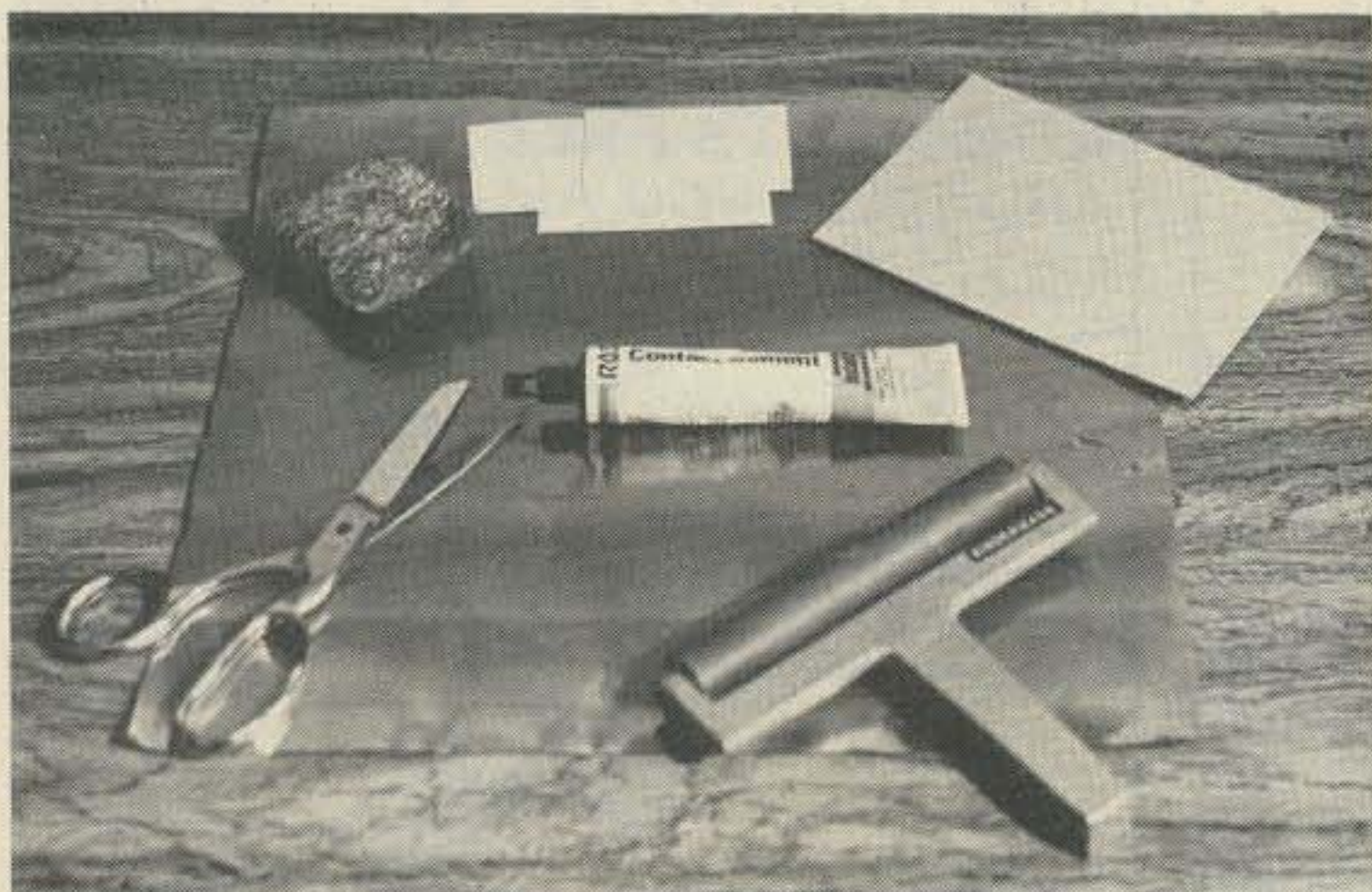
Fig. 1. Tools and materials needed are a pair of scissors, a steel wool soap pad, small pieces of cardboard cut from a filing card, contact cement, a sheet of copper and a phenolic board. The photographic roller is optional.
