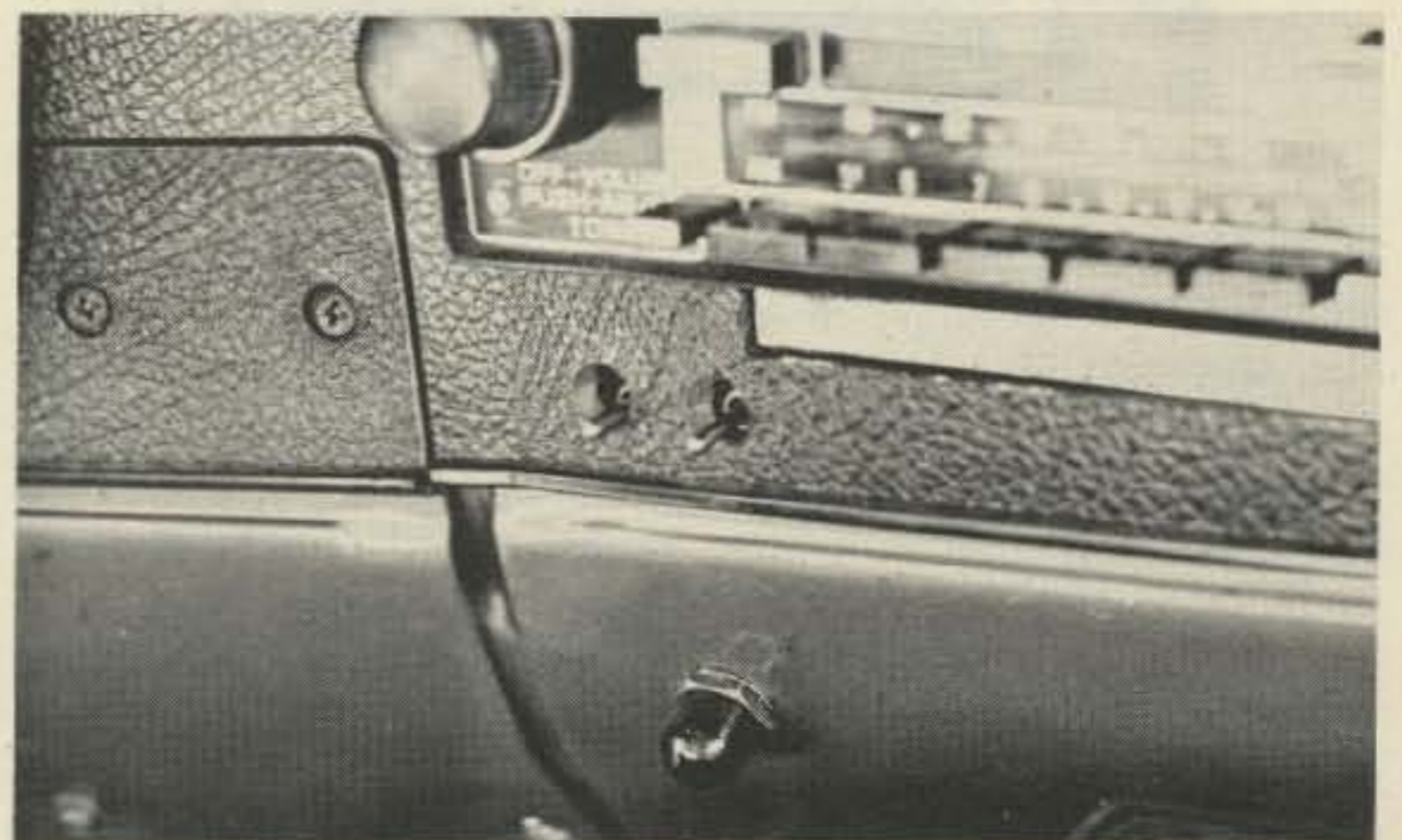
The automobile installation. The light is "on" when the alarm is not set. Of the two switches, the left, when pushed down, sets the tamper delay. When in the up position, the tamper alarm is on. The switch on the right controls another circuit in the car.
