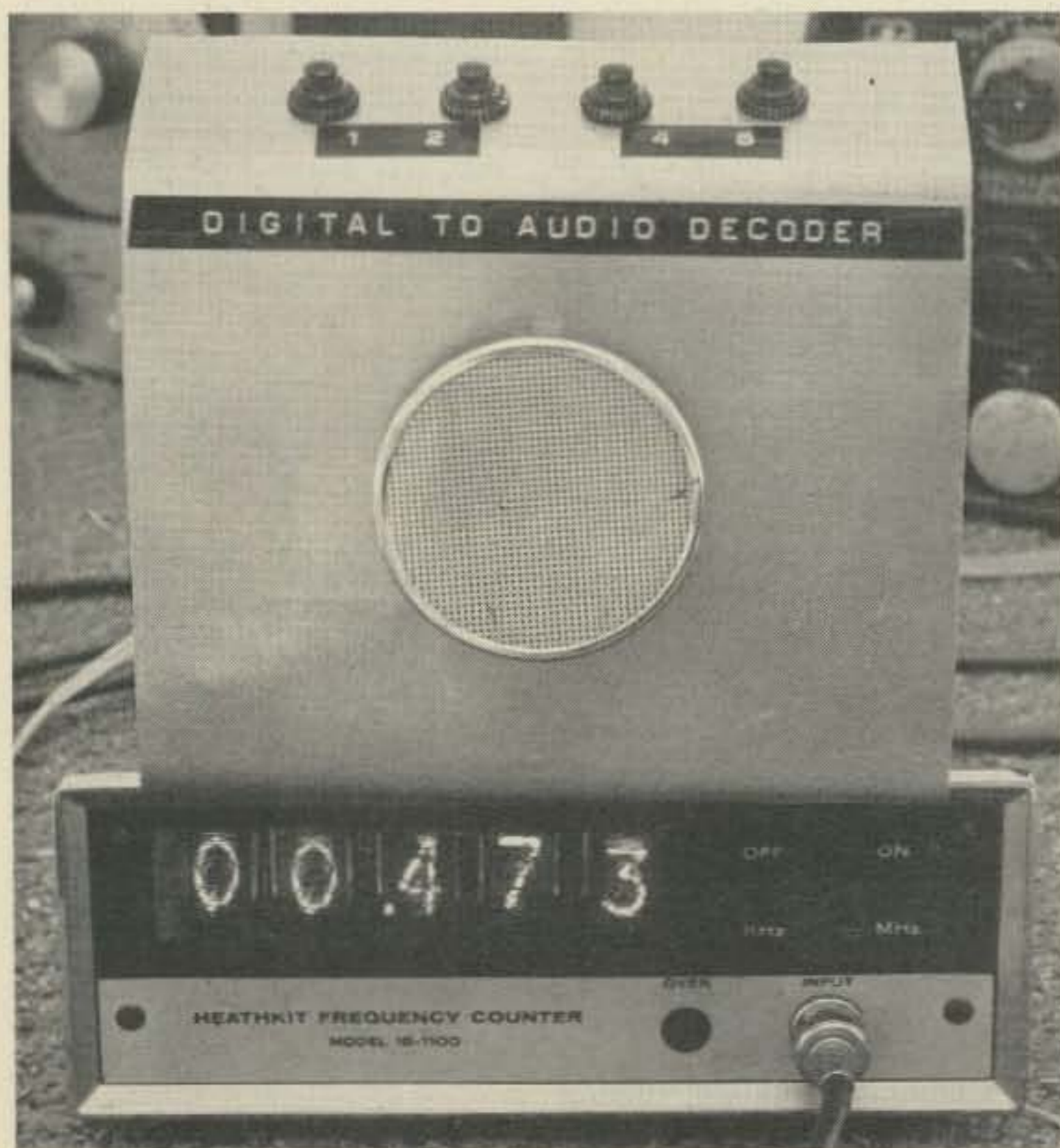
Photo 1. Digital to audio decoder and Heathkit IB1100 frequency counter.
