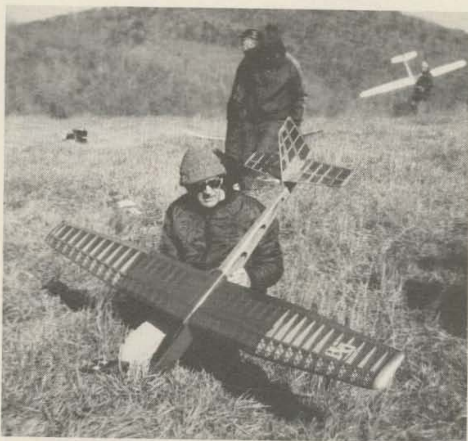
A modified Windrifter sailplane with transparent yellow plastic covering to show off internal craftsmanship. Span is 99 inches.
