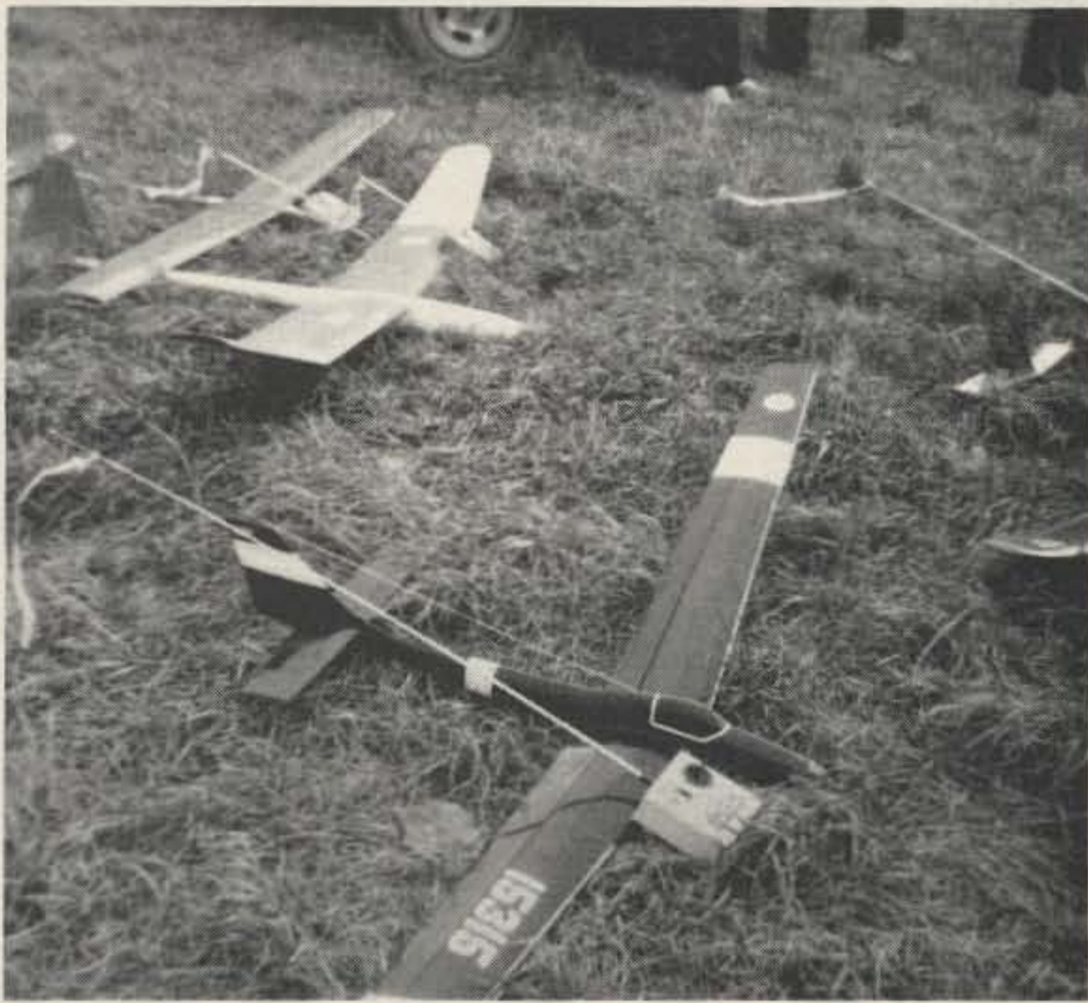
A "Hi-Pro" sailplane with molded fuselage and rudder. Wings have large movable flaps to change the airfoil and aircraft speed.
