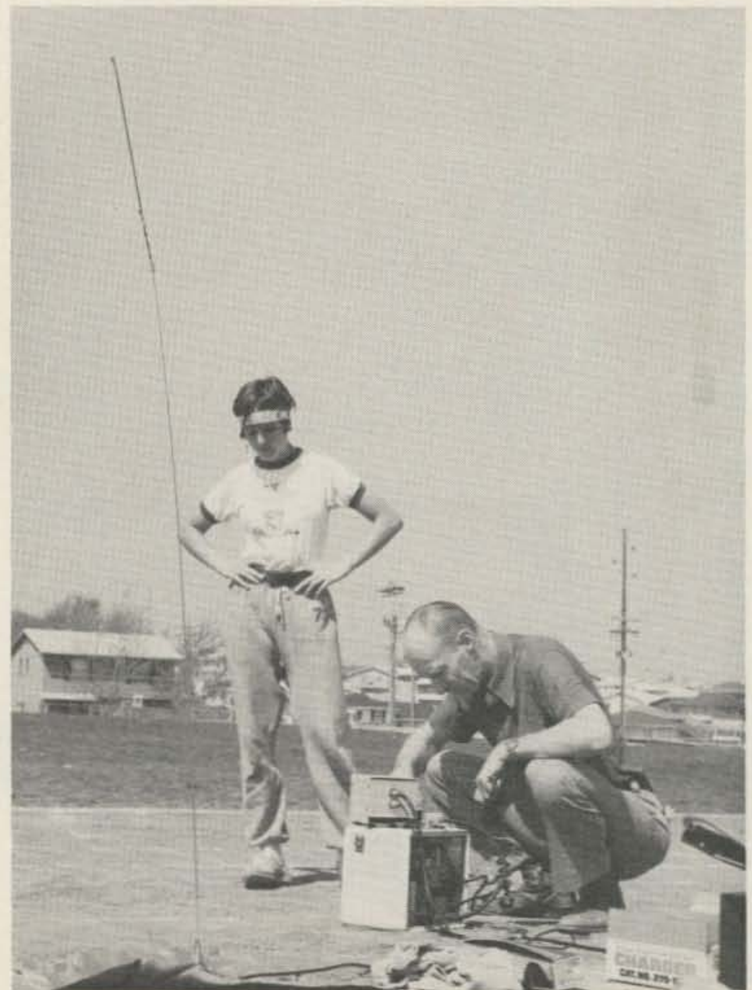
Ron Kinton WB0MBZ making some adjustments on the Gonset Communicator III during a practice session, with Sheila standing next to him. The antenna is a 5/8 wave on 2m extended to 1/4 plane on 6m using aluminum foil for a ground plane. Works FB, 1:1 swr.
