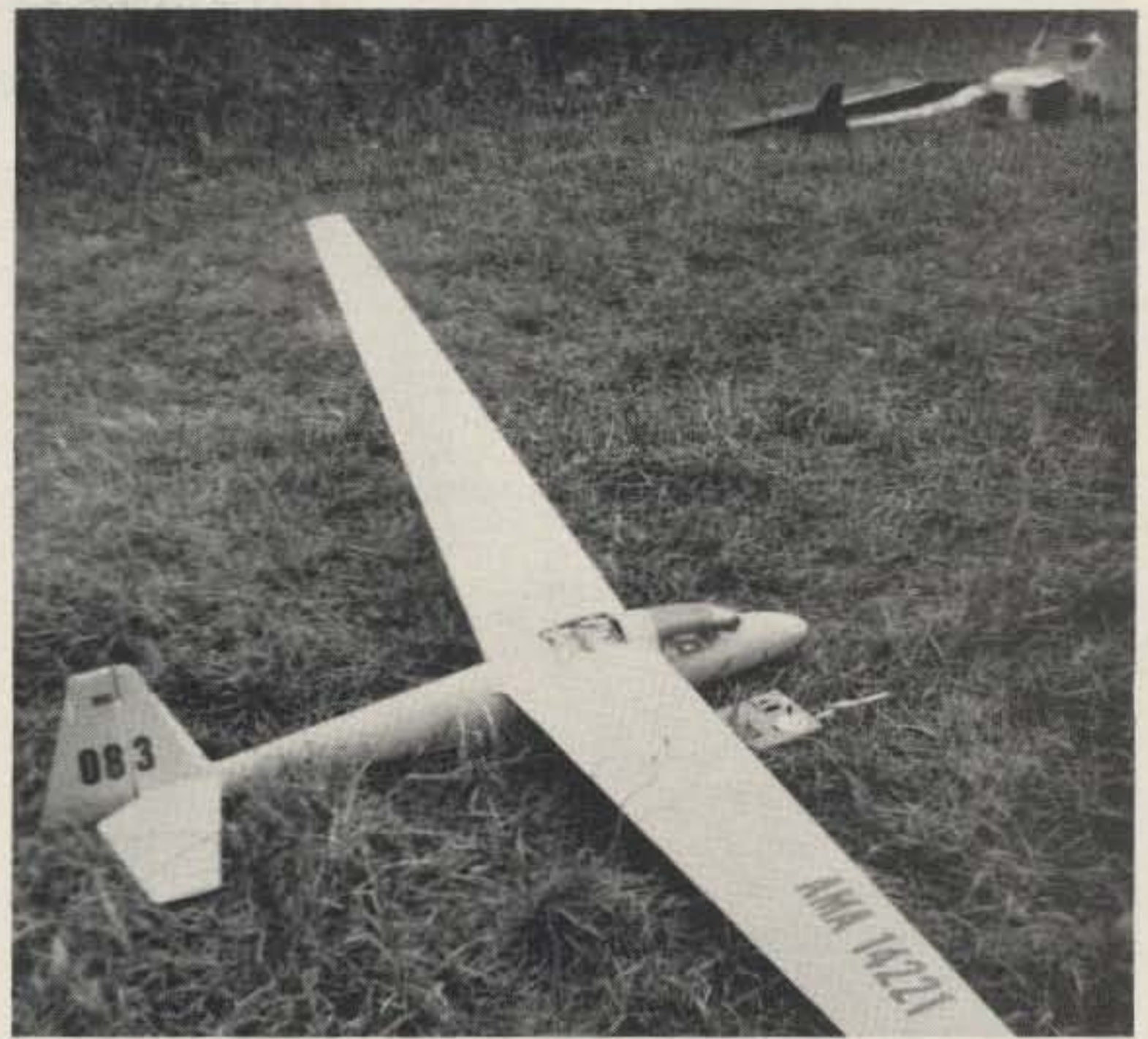
An all molded plastic and fiberglass model of a KA-6 sailplane. Span is 10½ feet, weight is nearly 12 pounds — ready to fly.
