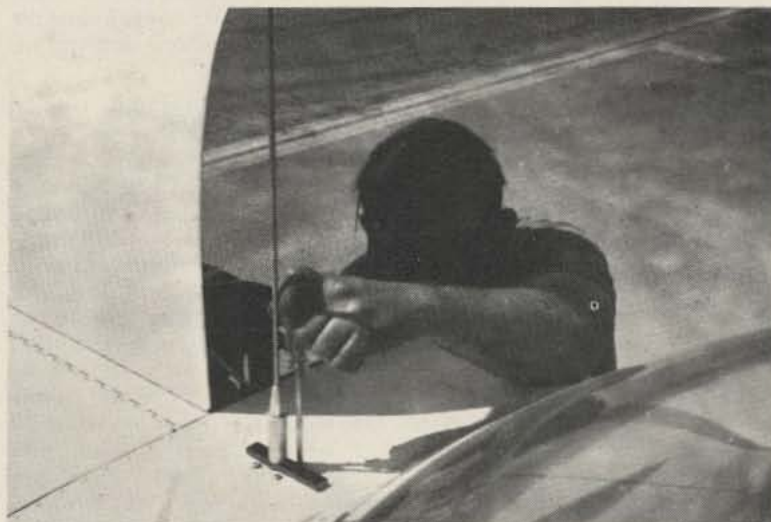
Dick Ulrich K6KCY puts finishing touches on the 10 meter whip for the OSCAR 7 test flight in 1973. Dick will participate in the flight test of the AMSAT/JAMSAT spacecraft in December.
