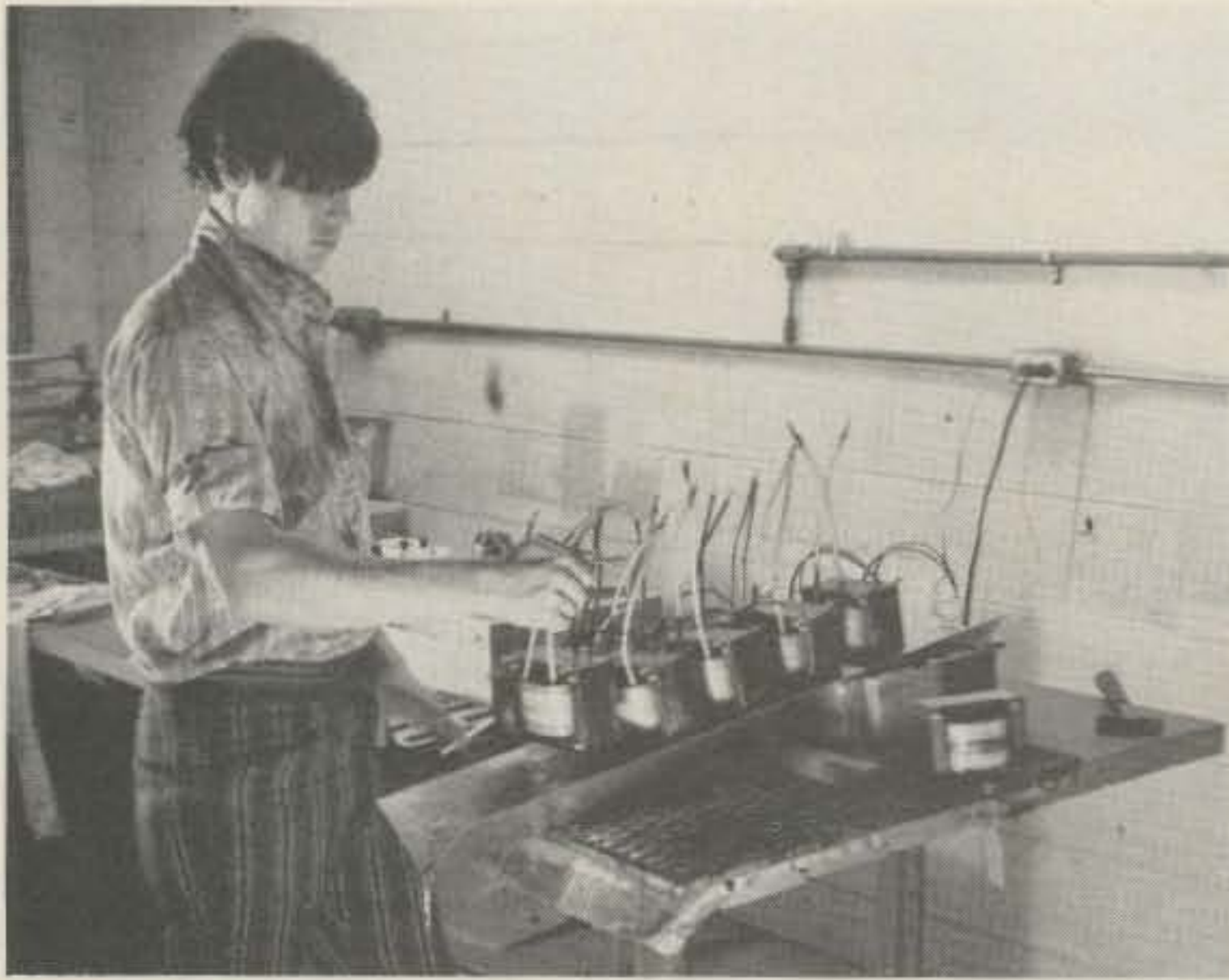
Even the power transformers for Ten-Tec equipment are wound at the Sevierville TN plant. A machine automatically inserts laminations in the transformer windings, then the whole affair is dipped in a sealant and put on a rack to harden.
