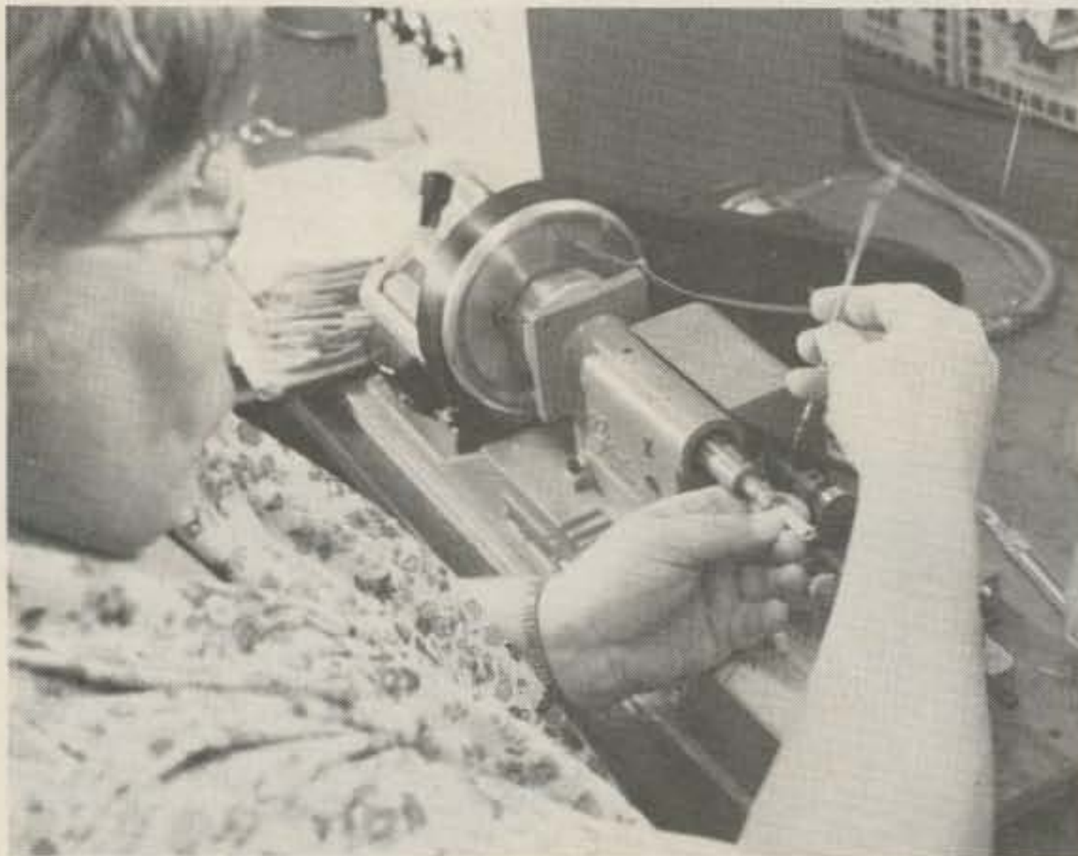
This coil winder is a Ten-Tec innovation. The machine is attached to a digital turns-counter, which also is programmed to stop the winder after the proper number of turns has been applied to the form. It saves time and cuts down on errors.
