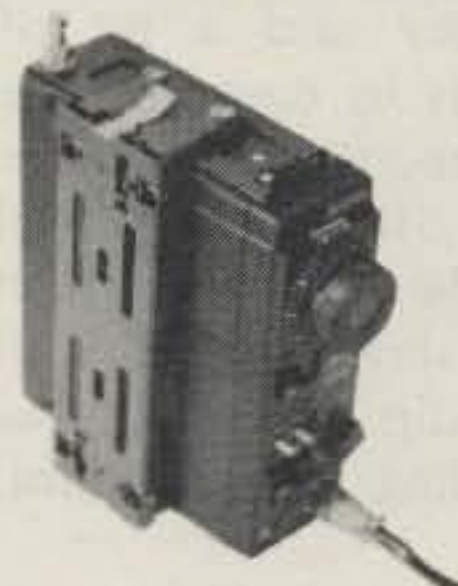
This new mobile mount is now available for your IC-215 . Fast insertion and removal is a snap, and the mount is collapsible when not in use.
