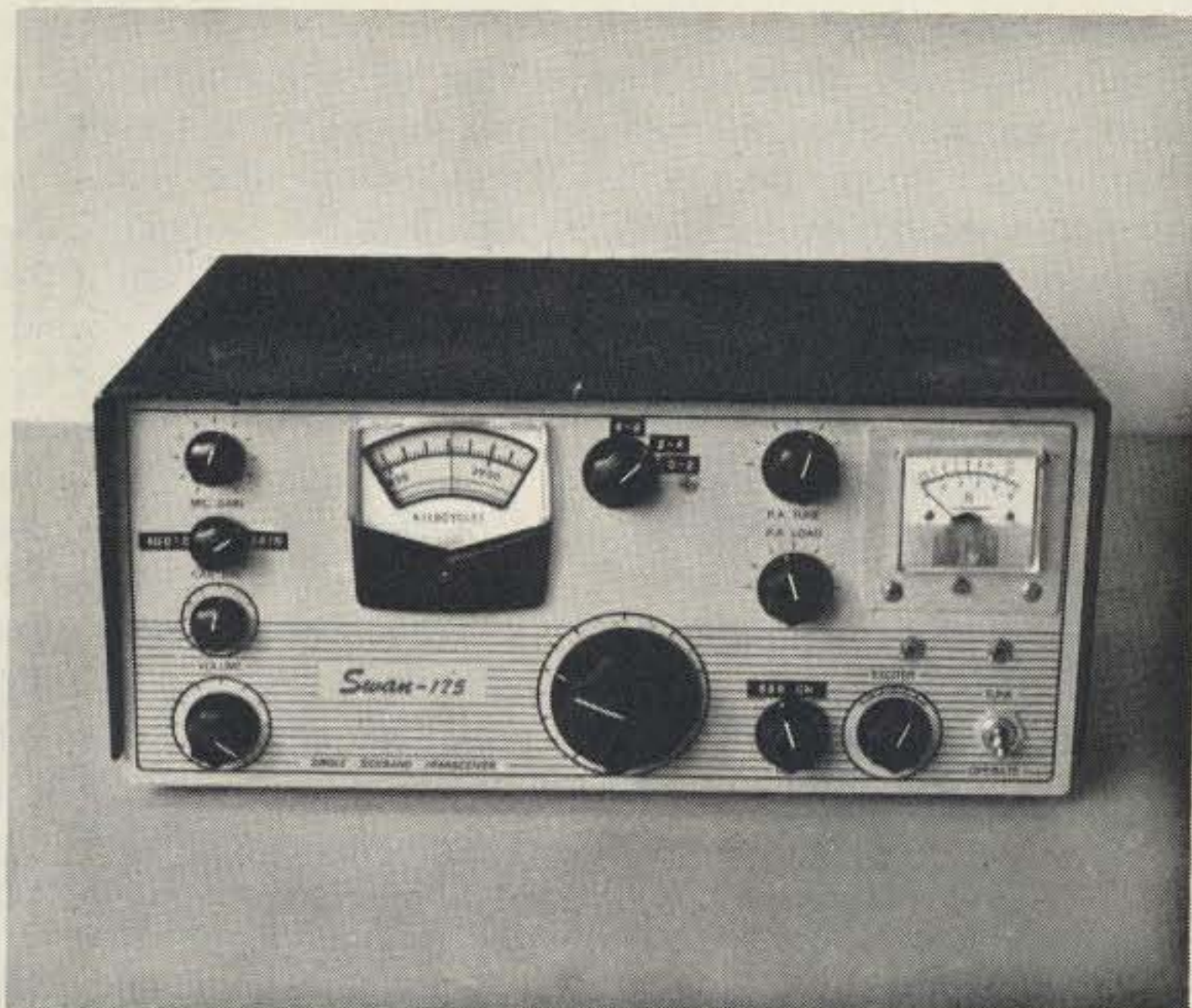
The front panel of the modified Swan retains much of its original appearance. The S-meter is mounted on an aluminum plate which covers the large hole left from removal of the original meter.
