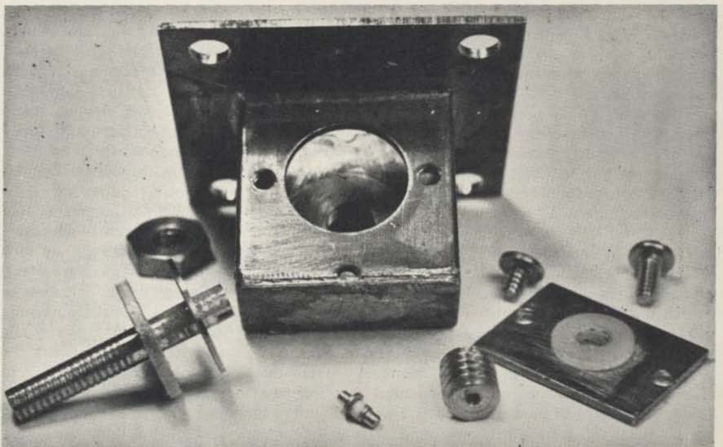
Photo B. Gunn effect oscillator assembly parts. Not shown is the cover iris to the waveguide flange.
