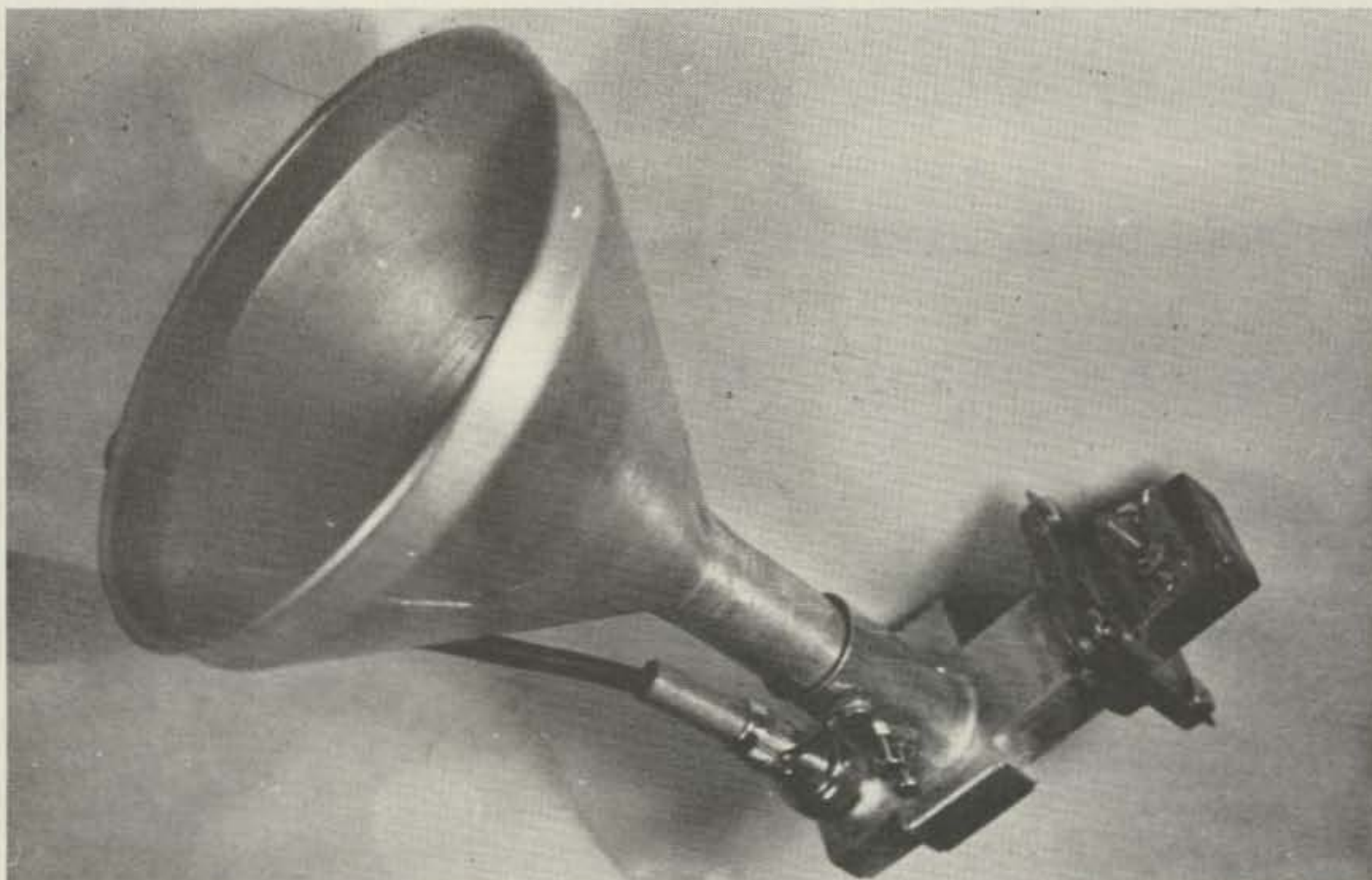
Photo A. The tuning screws and modulator diode are shown in a different position from that described in the text. These components may be located in either position, but the detector diode must be fed as shown to allow access to the tuning screws.
