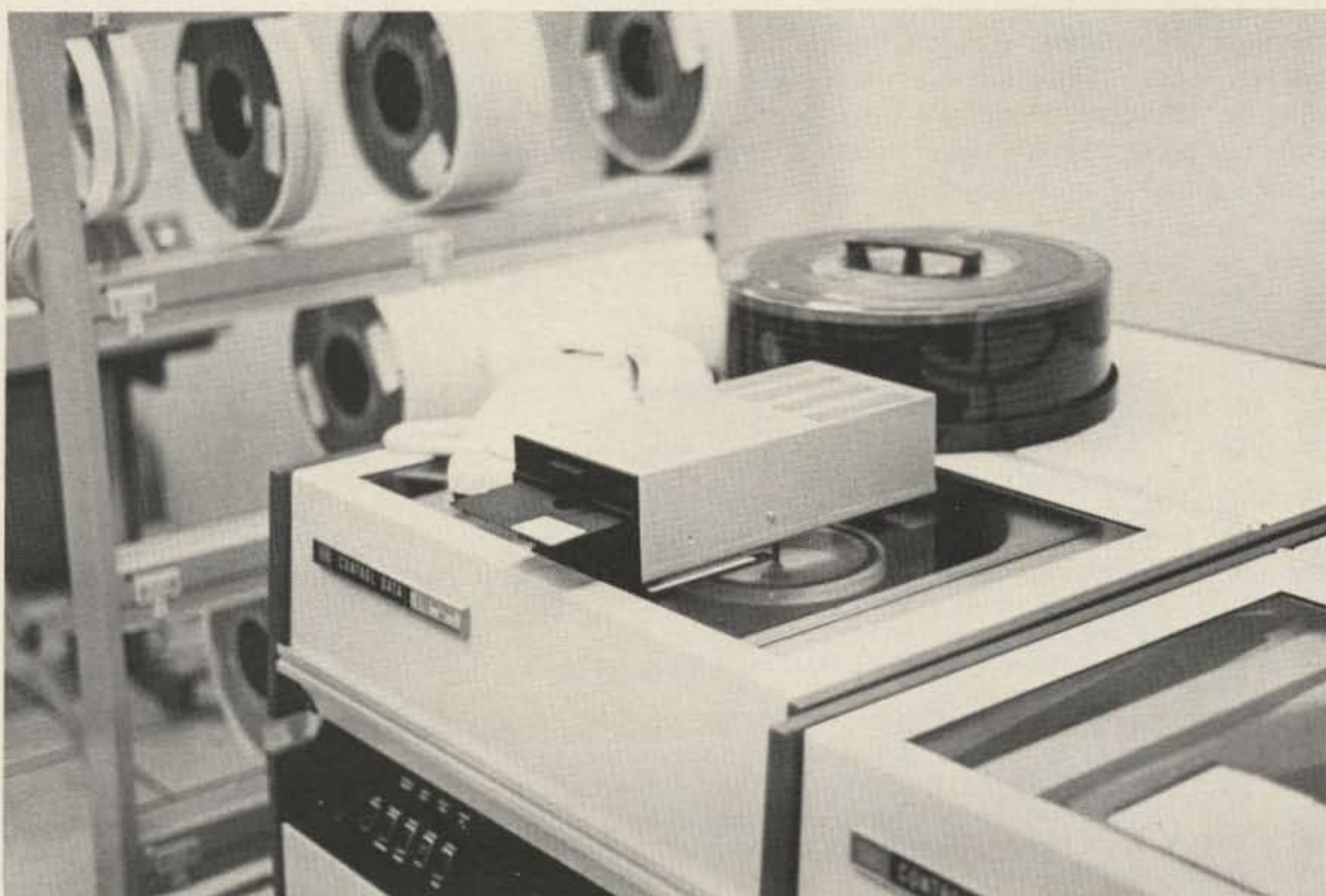
Photo B. It is interesting to compare the minidrive with a giant rigid disk system. This photo illustrates the relative sizes. Ball-park ratios for data capacity are 300 to 1. For price, the ratio is 1 to 18, and the large drive transfers data about 20 times as fast as the mini.
