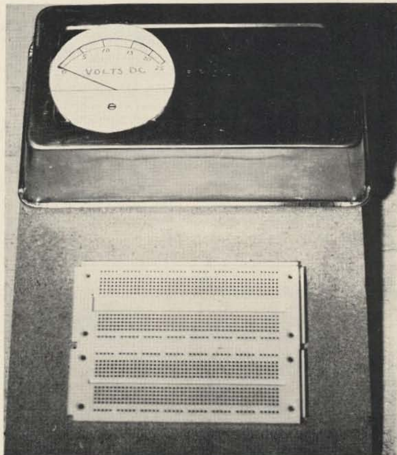
Photo D. Every breadboard needs a bread pan. Here is a bread pan used instead of a metal chassis. The bread pan is cheaper and easier to work with.
