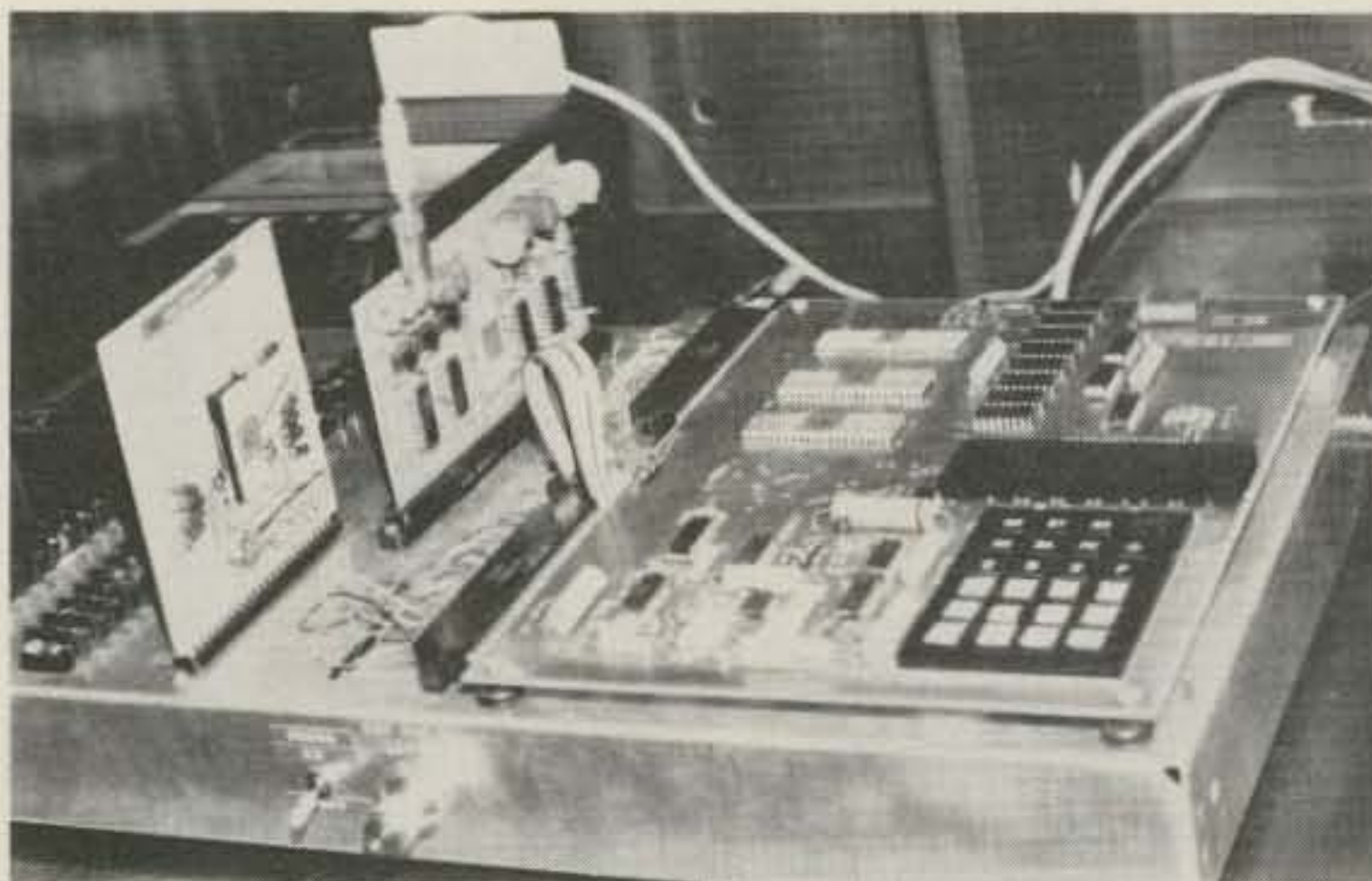
KIM mounted on aluminum chassis box with Lancaster TVT6-L and calculator interface.
