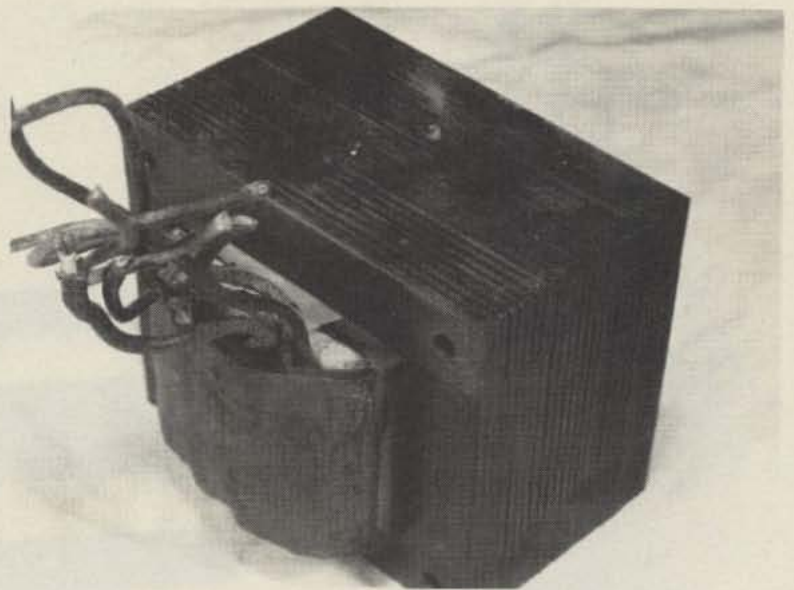
Photo B. Covers and static shield removed.
