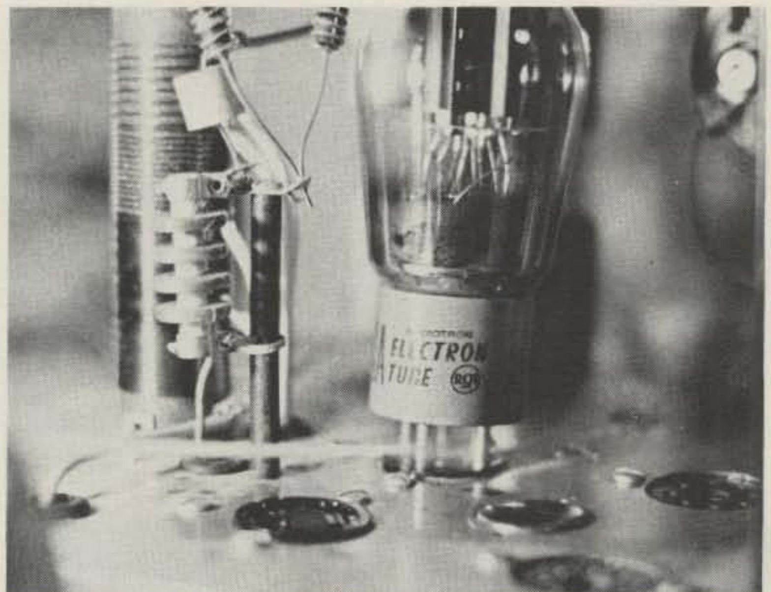
Photo E. Spray the tube and socket contacts and insert/remove the tube to clean mating contact surfaces.
