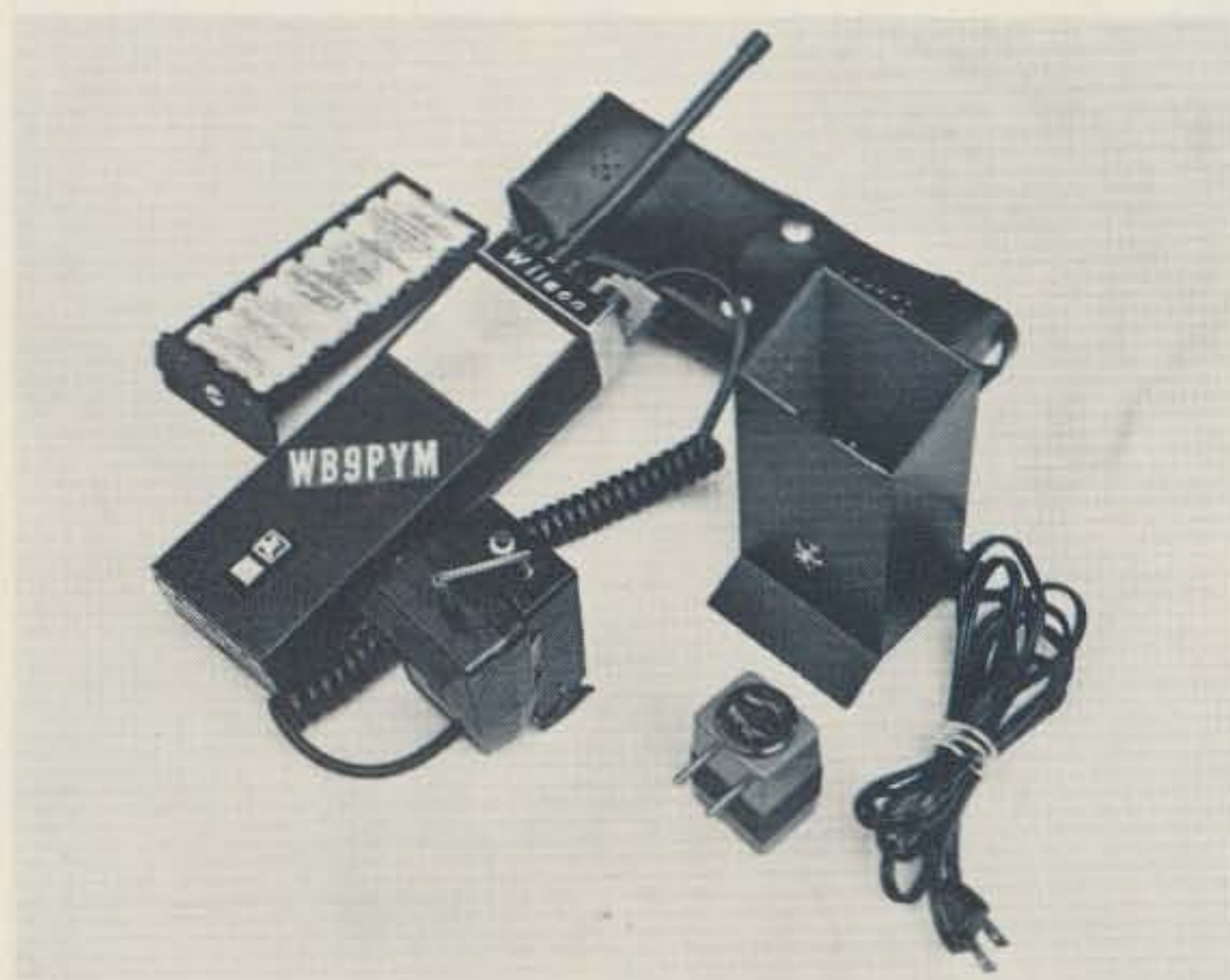
Photo A. A minimum of equipment is needed for 2m FM operation in Europe. In addition to a transceiver, take your external microphone fitted with a piggyback tone burst, charger for the nicads, 220/110 V ac converter, and an extra set of nicads.
