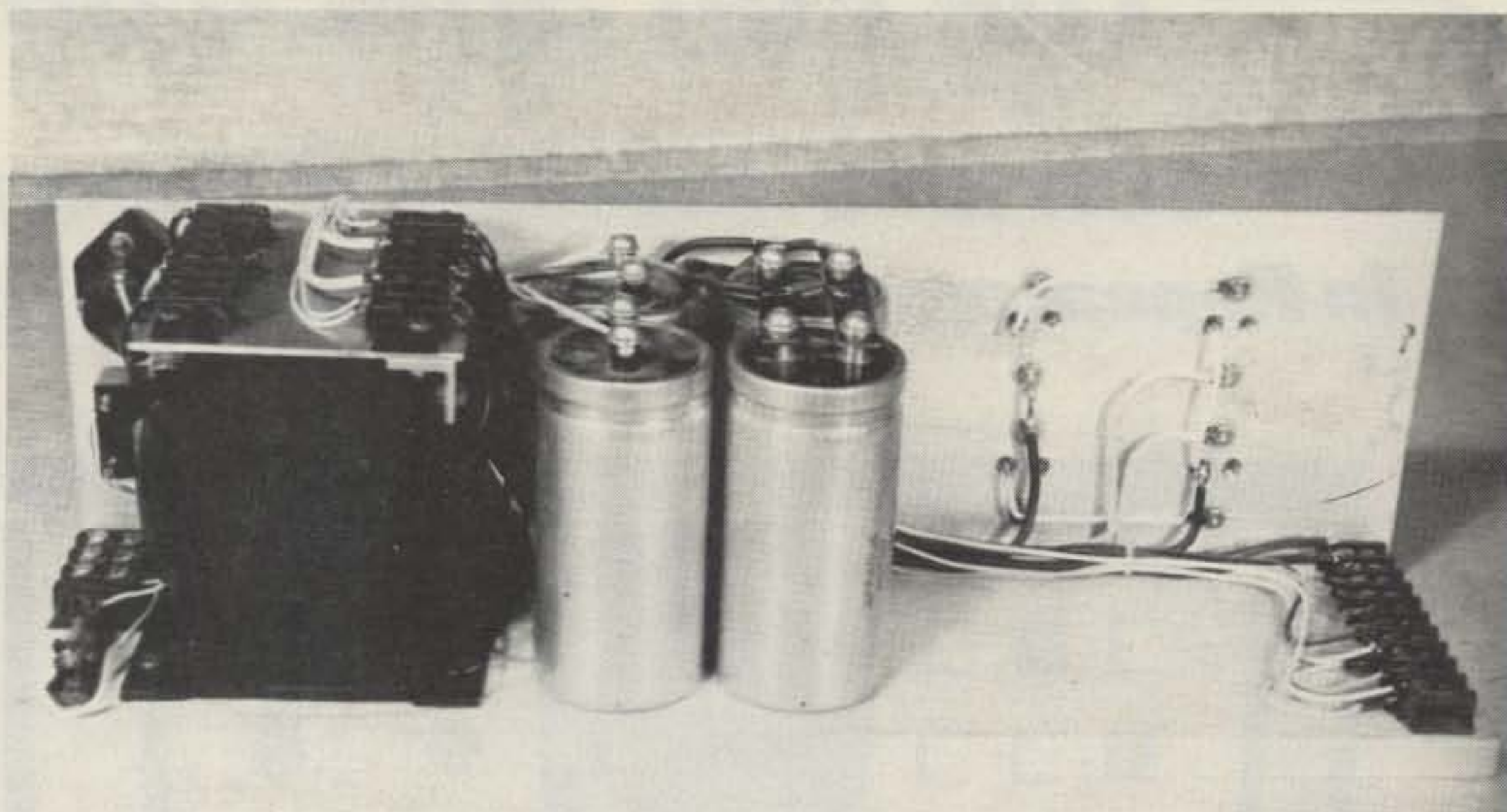
Photo G. The beauty. Possible output from regulators: 45 Amps @ 5 V; 10 Amps @ 12 V. Weight — 21 pounds!
