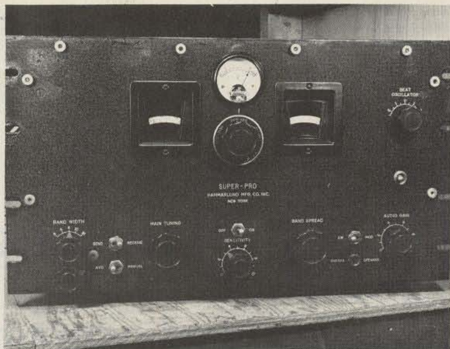
Photo L. Baby-oil treatment restores the wrinkle finish of this beautiful old 1937-vintage SP-100.
