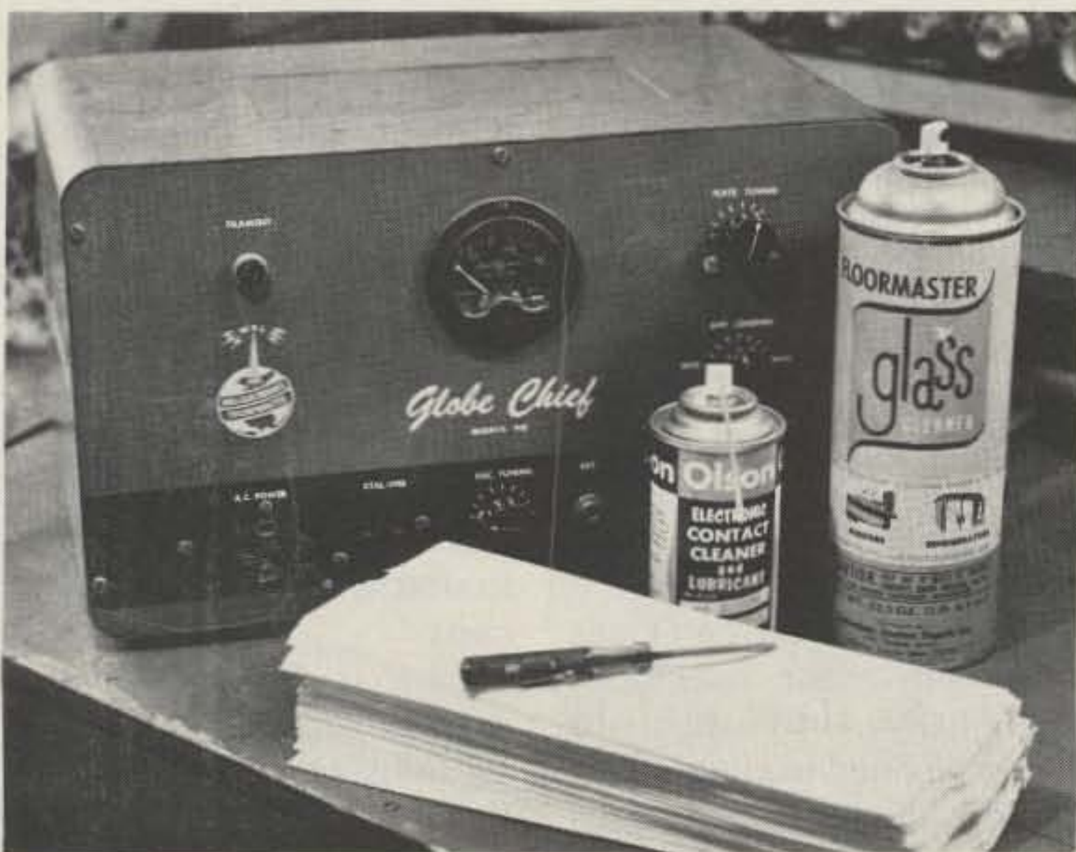
Photo C. Globe Chief transmitter with cleaning materials.
