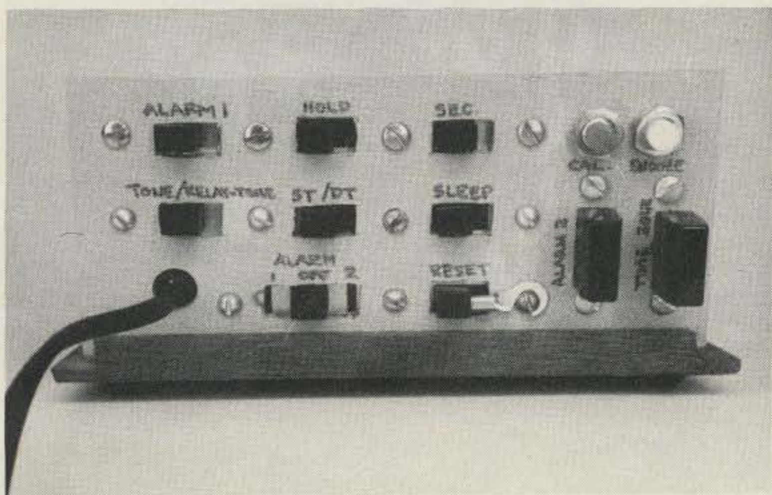
The rectangular cutouts for the switches were cut with a hot knife in the plastic rear panel. A solder lug blocks the reset switch to prevent accidental closure.
