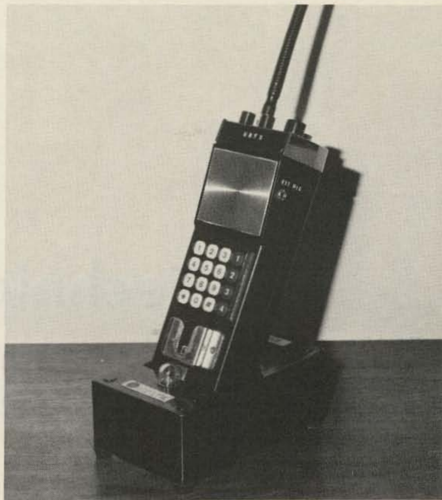
Photo B. HT is shown in the non-charging reclining position. Once charging is complete, the unit can be disconnected from the charger and is ready to operate portable or fixed-base as shown in the photo.
