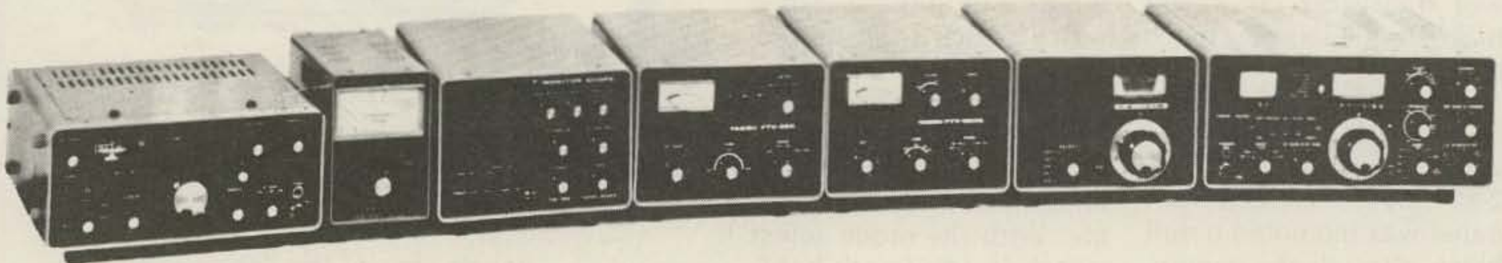
Left to right — FT-620B, 6 Meter Transceiver • YP-150, Dummy Load Wattmeter • YO-101, Monitor Scope • FTV-250, 2 Meter Transverter • FTV-650, 6 Meter Transverter • FV-101B, External VFO • FT-101F 160-10M Transceiver
