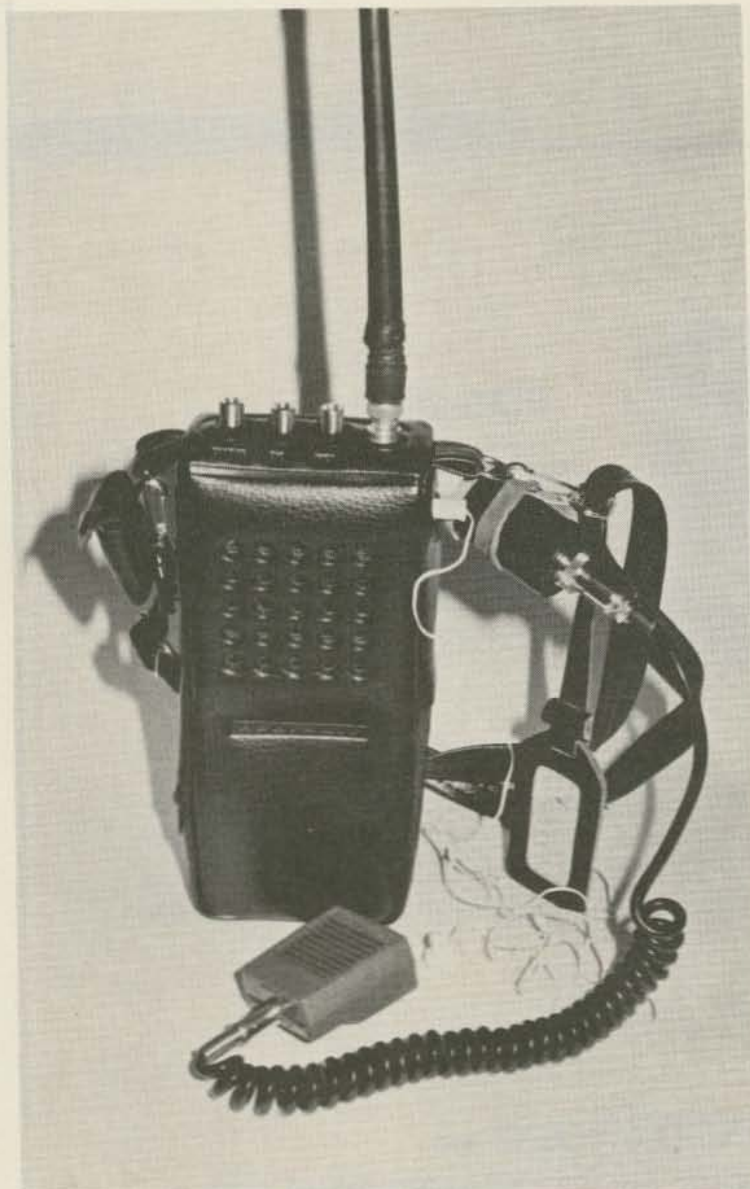
Unit ready for external PTT and private listening. Heath microphone element had been installed in the Motorola housing to keep the system matched.
