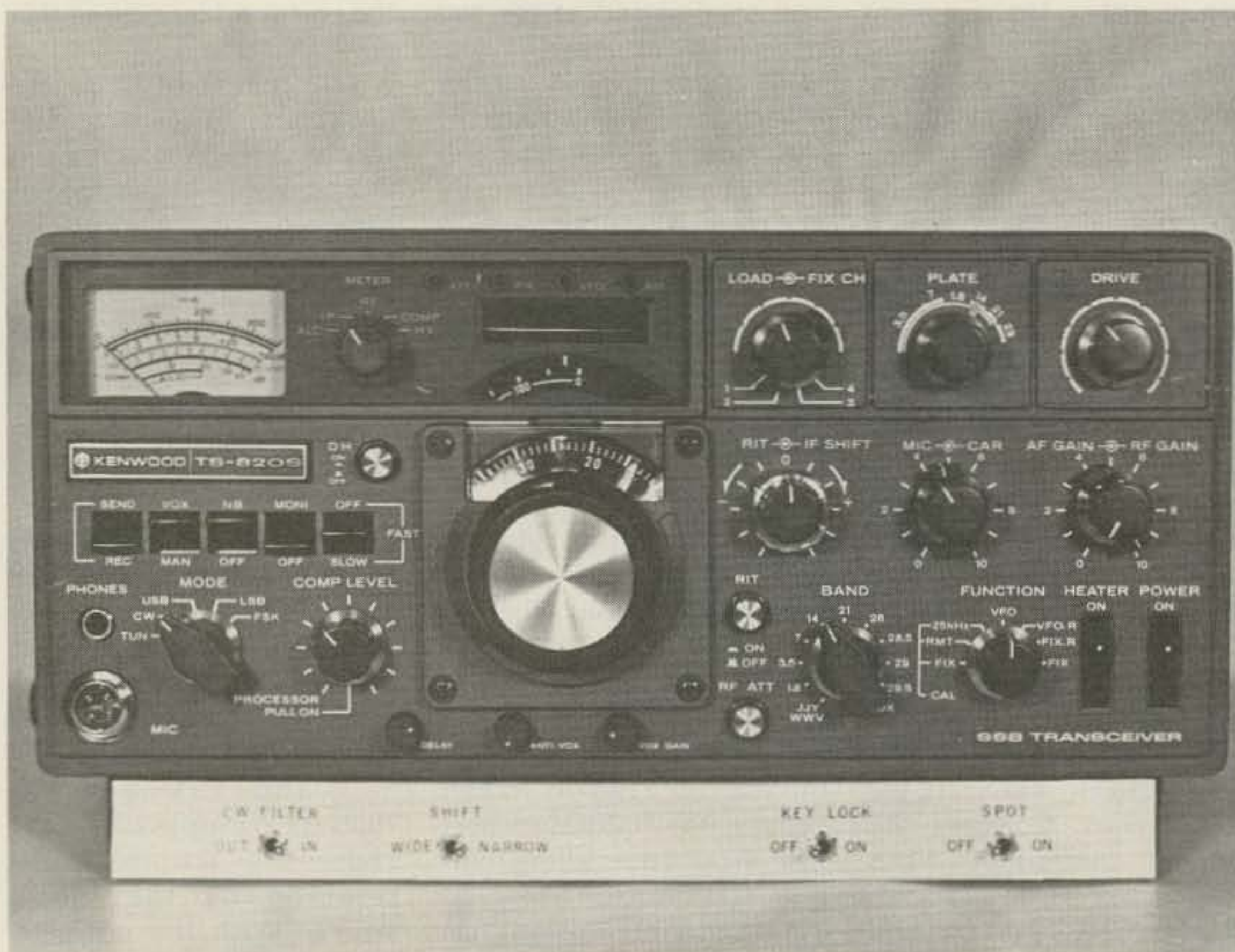
This prototype control panel was silver with black lettering. Future versions will be black-anodized, with white photoengraved lettering.
