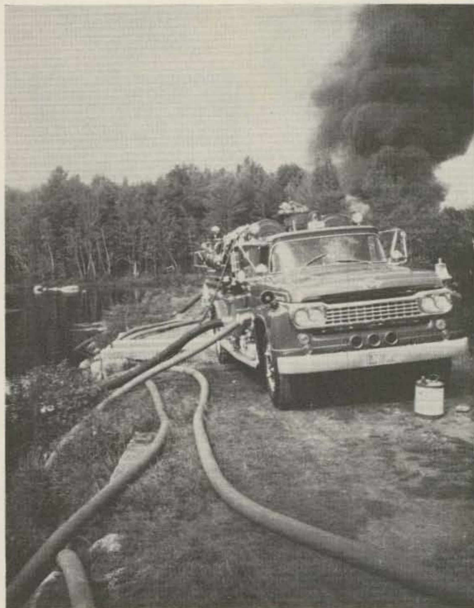
Pumpers at Meadowood (Bowker Pond) supplying water for the practical sessions.
