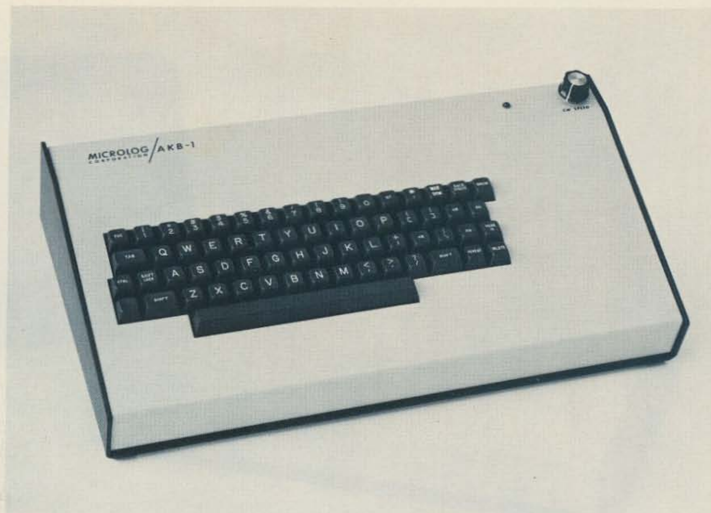
Microlog AKB-1 keyboard. Although there are many options available for the keyboard, only one is visible from the exterior. In the upper row, third key from the right, a special key-cap is installed with the owner's call when the ID option is ordered. All other options are internal.
