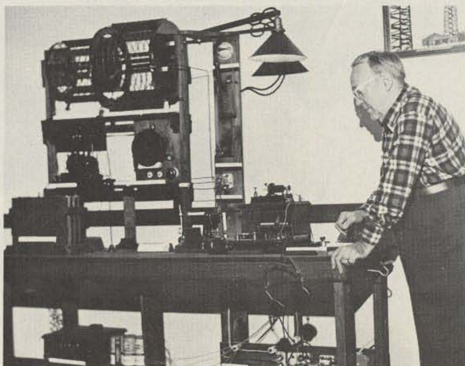
Frank Caswell W1ALT mans the "ole pump handle" of this working model of the rotary spark-gap transmitter which Marconi used. Caswell built it in his spare time, and it is housed in the National Seashore Visitor's Center.
