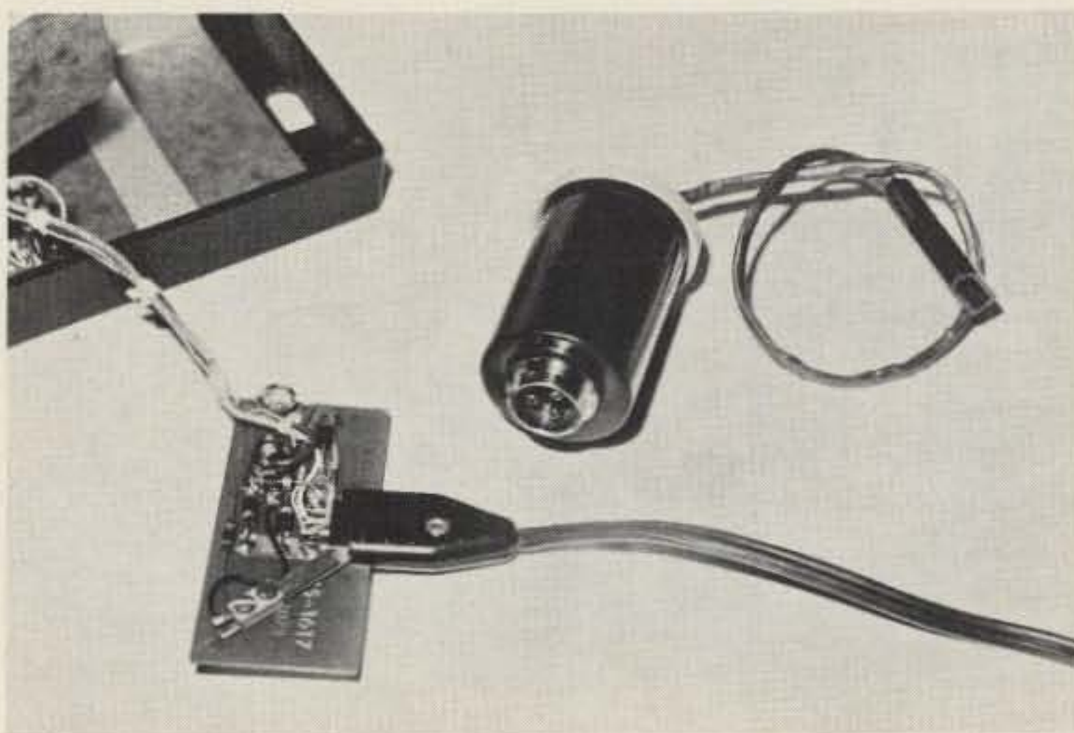
The external microphone adapter mentioned in the text and the SPST switch added to the battery charger board. The notched battery charger connector is plugged in, showing how the notch keeps the switch from functioning during battery charging.
