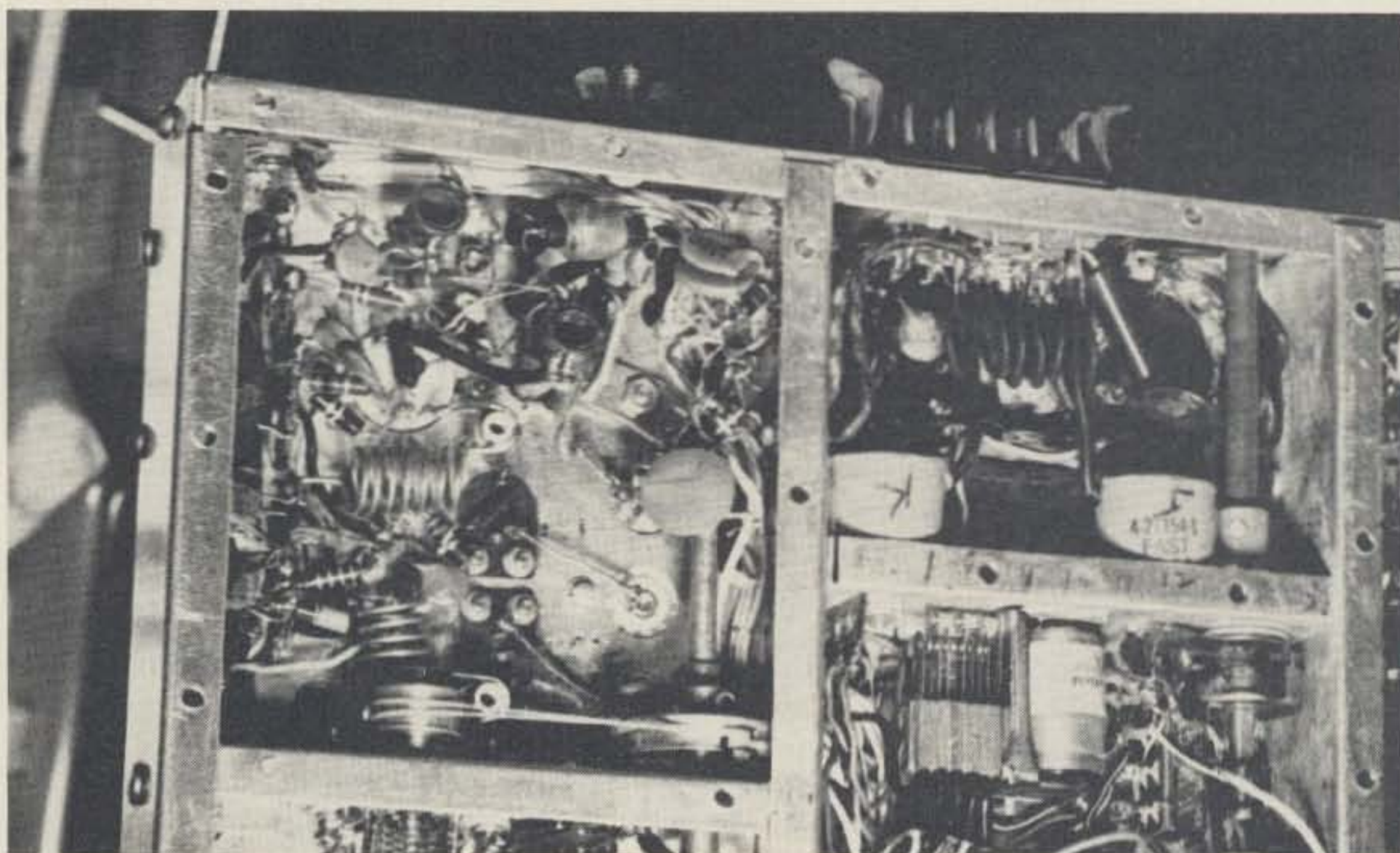
A close inspection of the compartment in the upper-left quadrant shows the phase modulator tube socket and two terminal strips that were added to modify the Pawnee transmitter.
