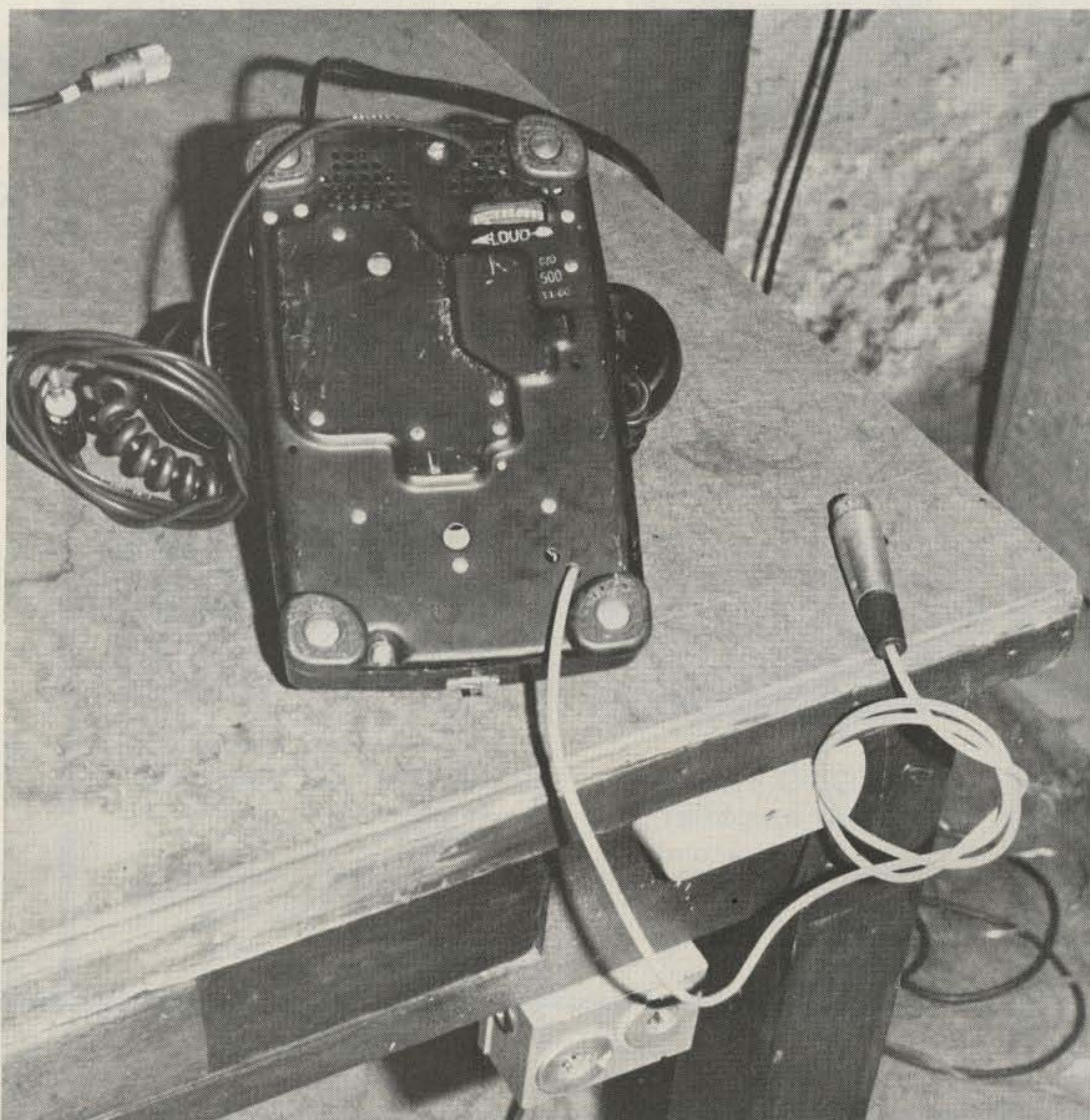
Underside view of phone with patch inside. The wire coming out of the uppermost part plugs into the Drake's mic input. The lower wire plugs into the Cannon box below the electrical outlet (bottom of picture). The PTT switch is centered in the bottom of the front of the phone.
