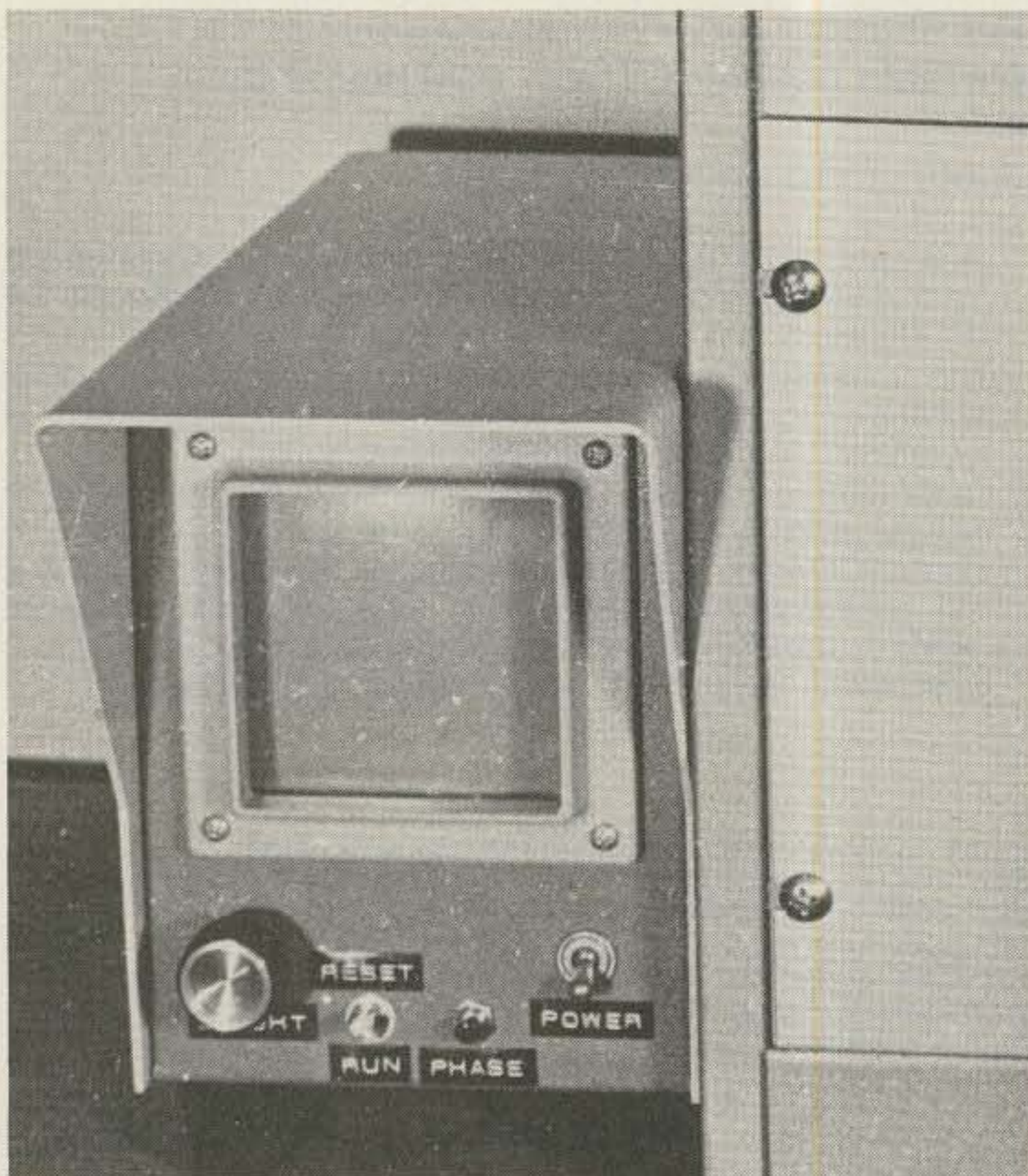
Photo A. The remote display terminal in the author's prototype. This used the cabinet, bezel, CRT, HV module, and yoke from a Robot fast-scan viewfinder. The cabinet contains these components and the relevant CRT circuits.
