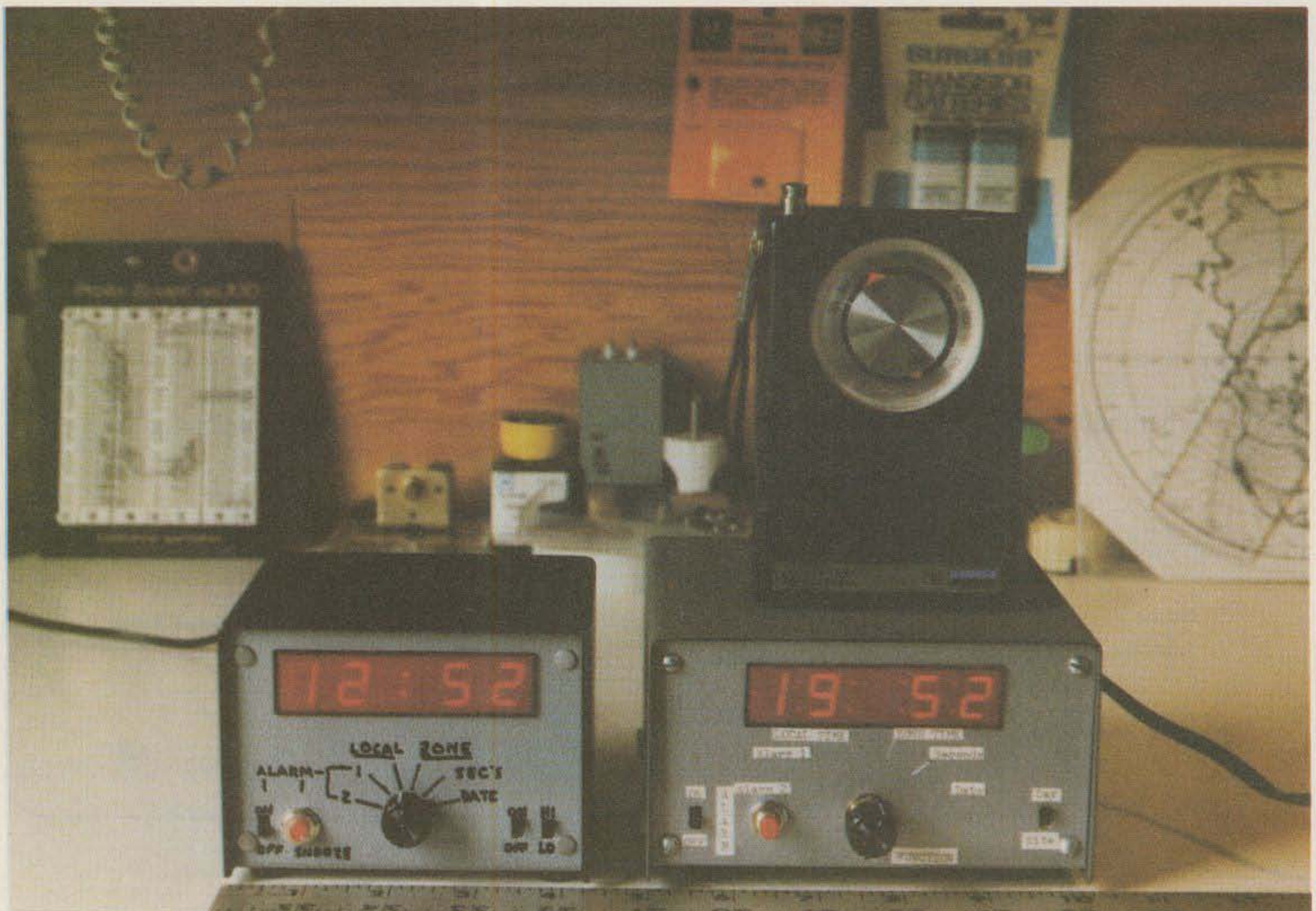
Both clocks set up and operating. The small clock is on GMT, the other on local time. The radio is connected to the alarm output of the larger clock.
