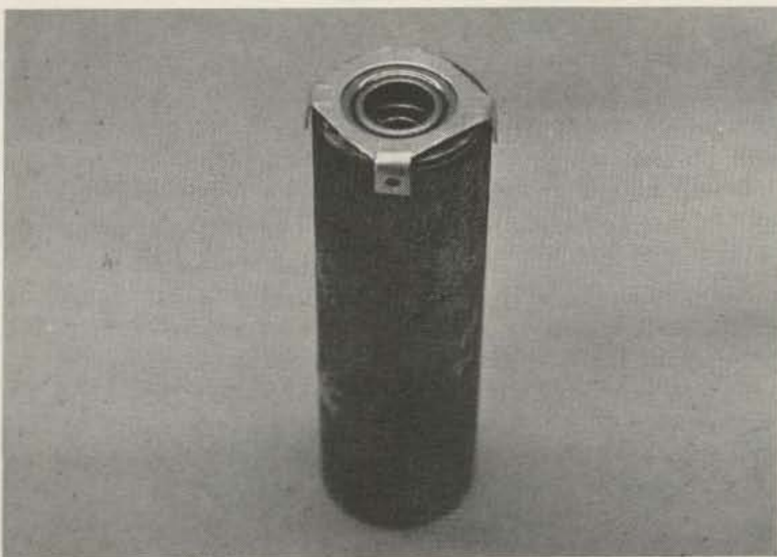
Photo D. Bicycle axle held in tubing by use of aluminum retainer.
