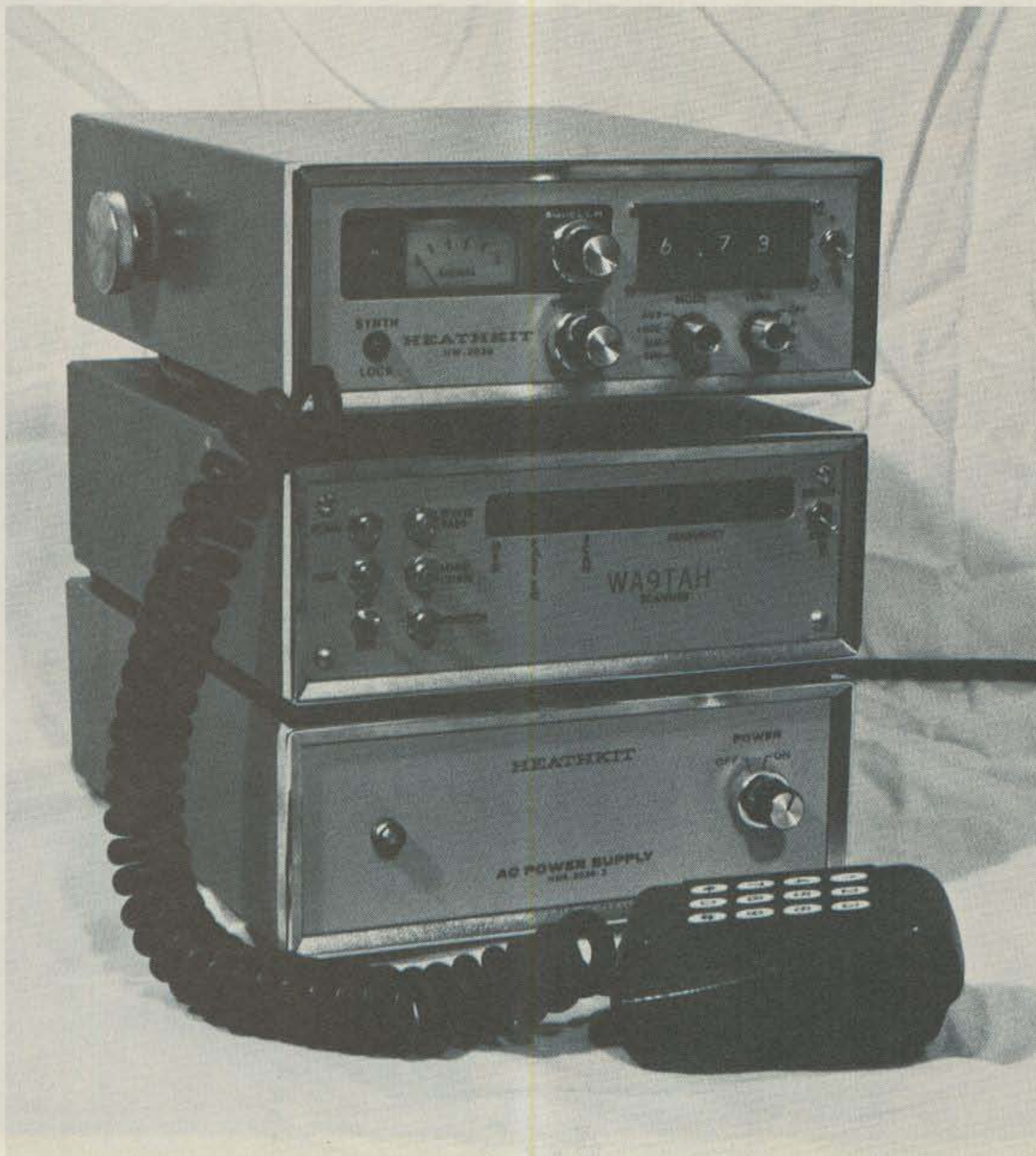
Overall view of the author's 2 meter FM setup with Heath power supply, WA9TAH scanner, and HW-2036 transceiver.
