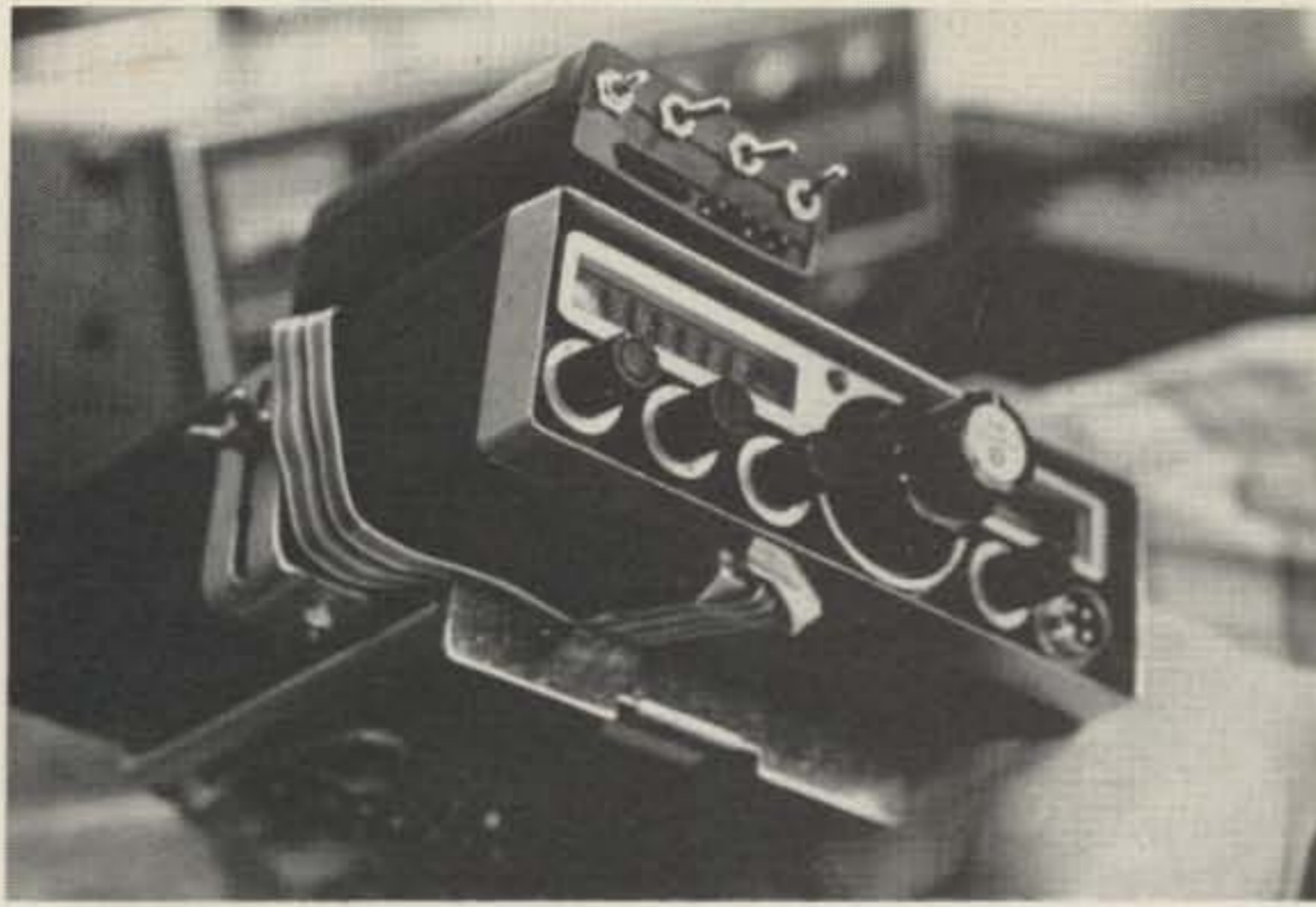
The 16-conductor flat cable was routed around the side and through the case at the front molding. The light object at the point of entrance is a folded-over business card used to protect the cable from being pinched.
