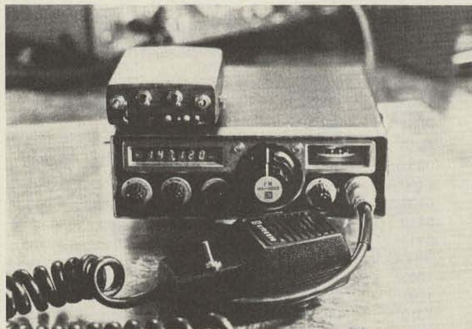
View of the scanner on top of the KDK. Velcro™ is used to hold it in place.
