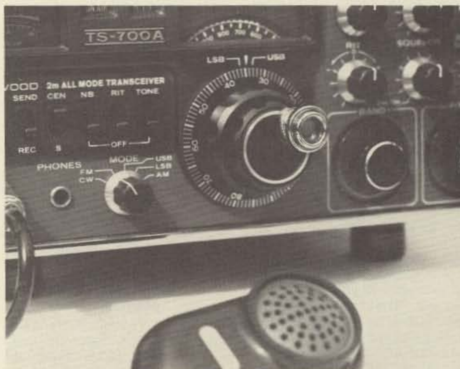
Photo B. Spinner knob on the TS-700A.
