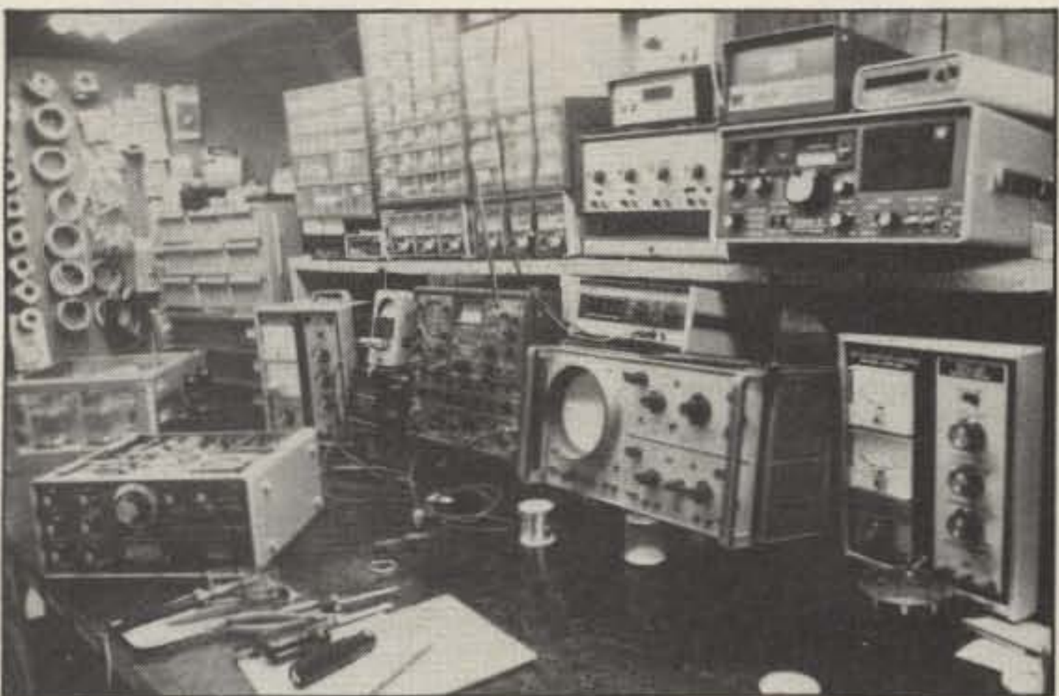
Service Shop — You've probably heard of our fine service reputation — using Cushman CE4B signal generators, Hewlett Packard oscilloscopes, Bird wattmeters — we fix it right!
