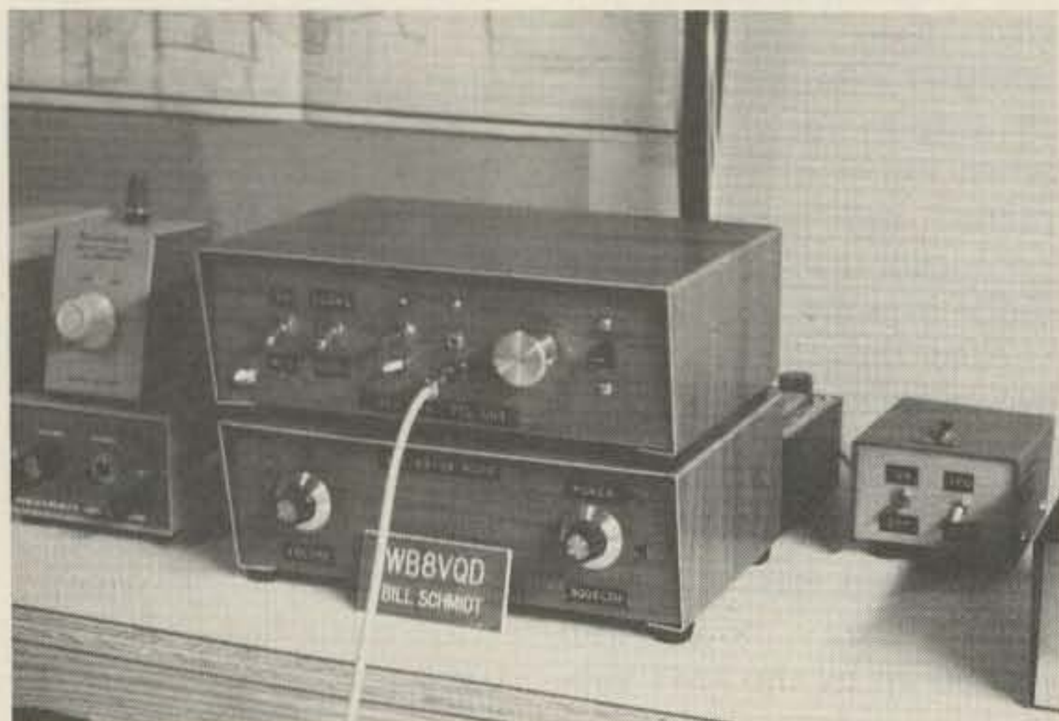
Terminal unit provides both 60 mA loop for mechanical machine when we want hard copy and TTL level signals for the computer.
