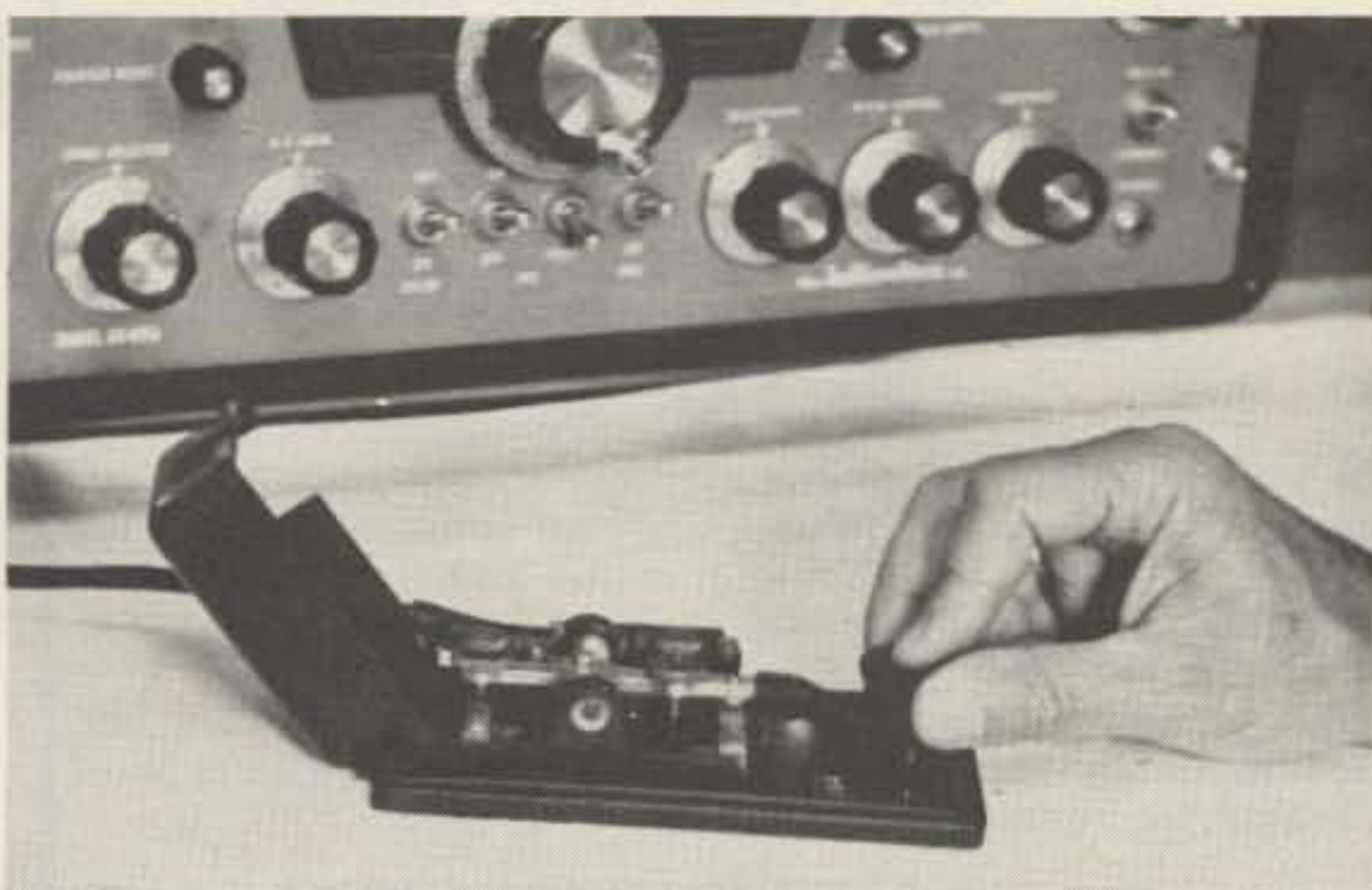
Here is a German Baumuster T1 military key of the 1930s. "This is my favorite hand key because the adjustments are precise and the concave knob gives it a good feel," says John Elwood, who purchased the key from Louise Moreau W3WRE. In the background is John's Hallicrafters SX-101A receiver. That's John's precise fist in action.
