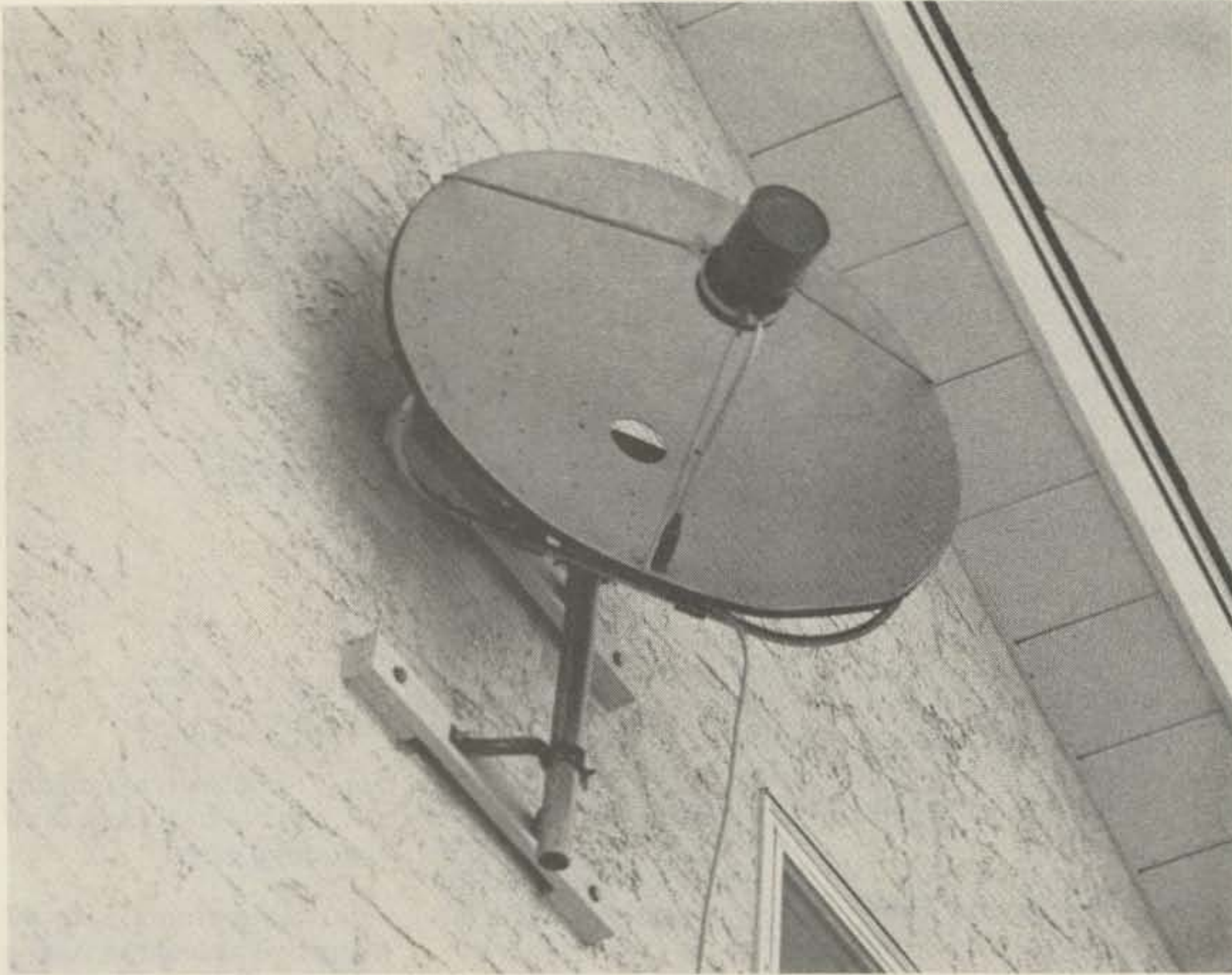
Photo 1. This is a 74-cm (29-inch) commercial reflector using a WA9HUV coffee can feedhorn. Located 4.5 meters (15 feet) high, this antenna pulls in snowfree color MDS TV signals over a distance of 32 kilometers (20 miles).
