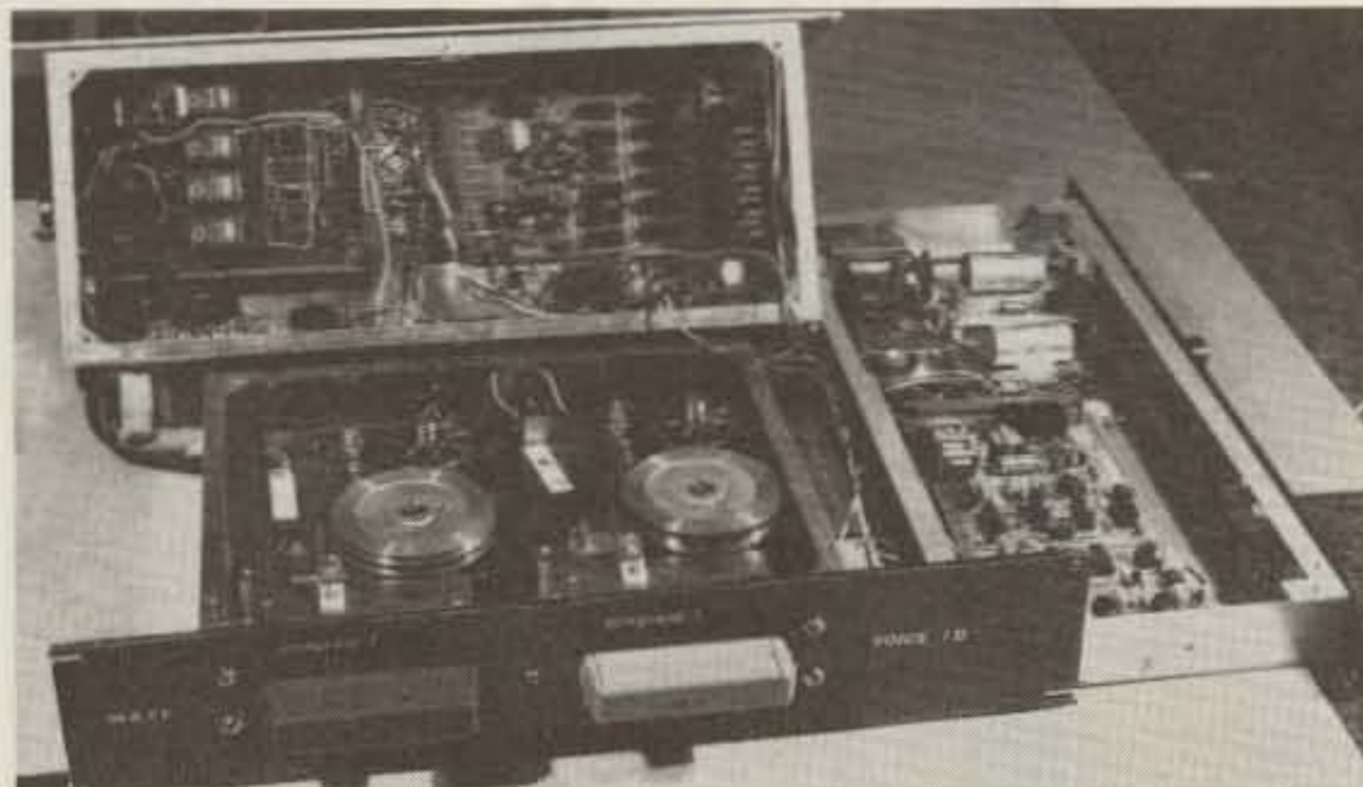
This is the M.A.R.C. voice ID system. Two of the four tape decks are shown, mounting into one chassis with access to the tapes from the front. The underneath view of the electronics shows the function decoder board on the right and the address field-motor switching on the left. The audio patch is on the extreme right of the picture.
