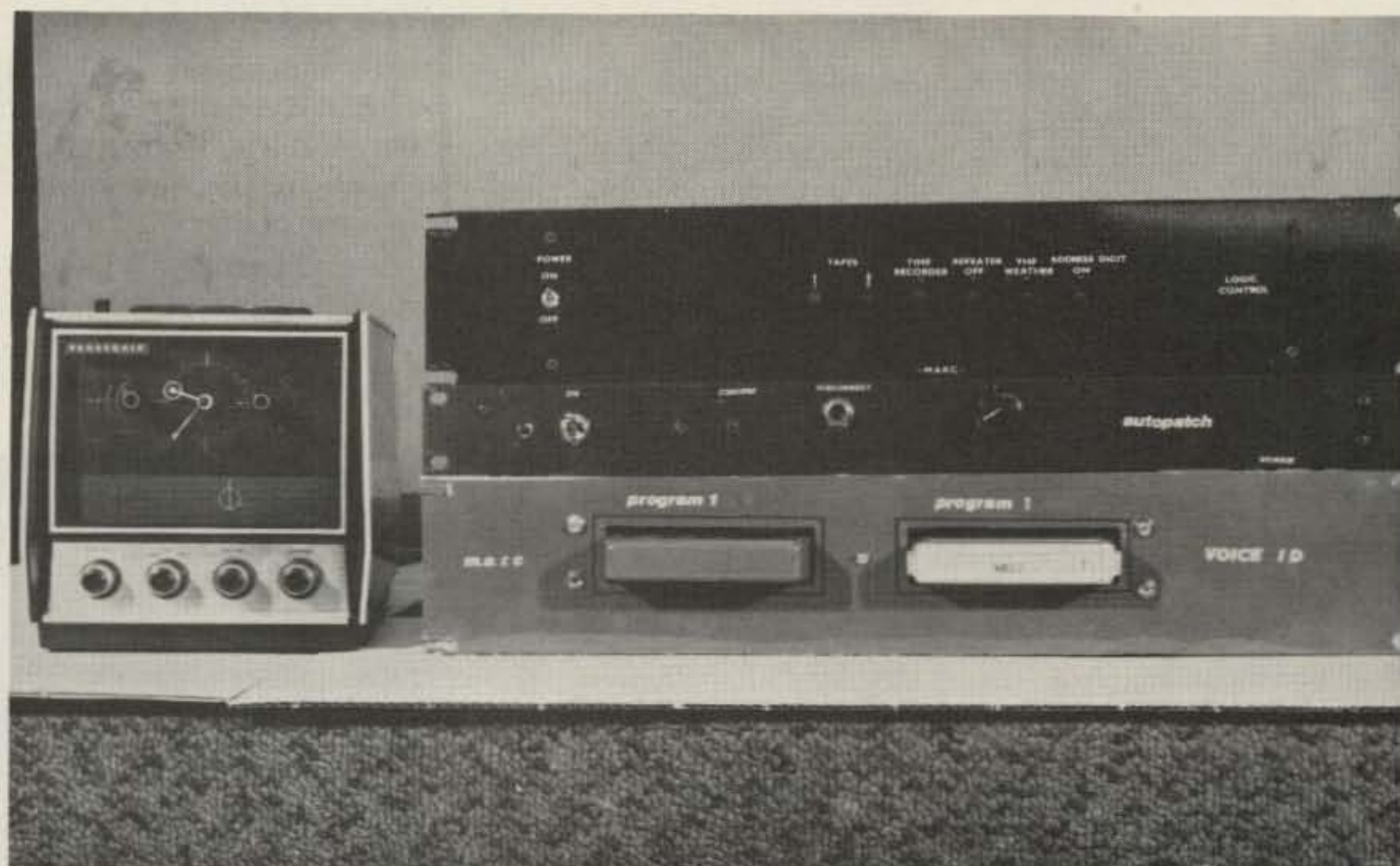
The front view before rack-mounting shows the Panasonic RC 6800 Talking Clock Radio used as the time machine. The stack on the right consists of the logic control, autopatch, and two of the four tape machines.
