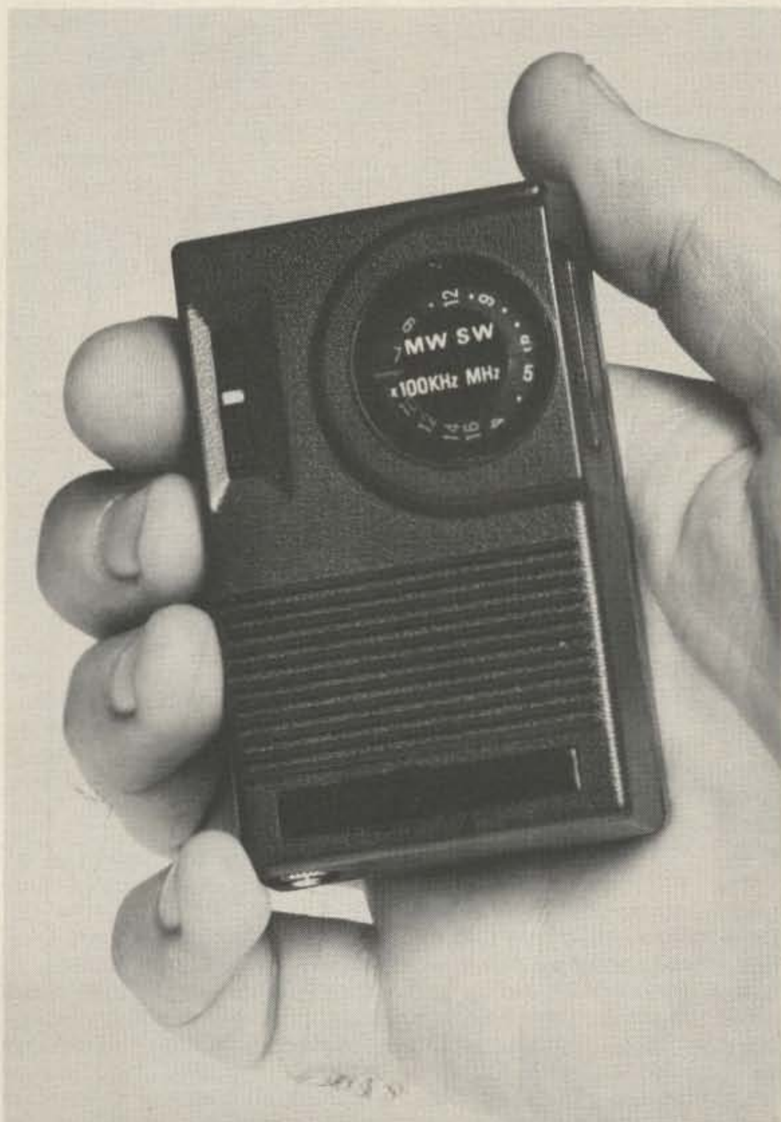
Radios International's EP-8 shortwave receiver.
