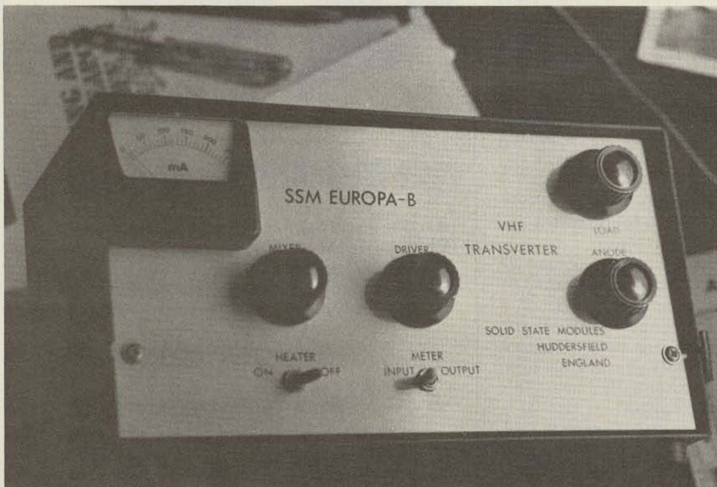
The Europa-B two meter transverter.
