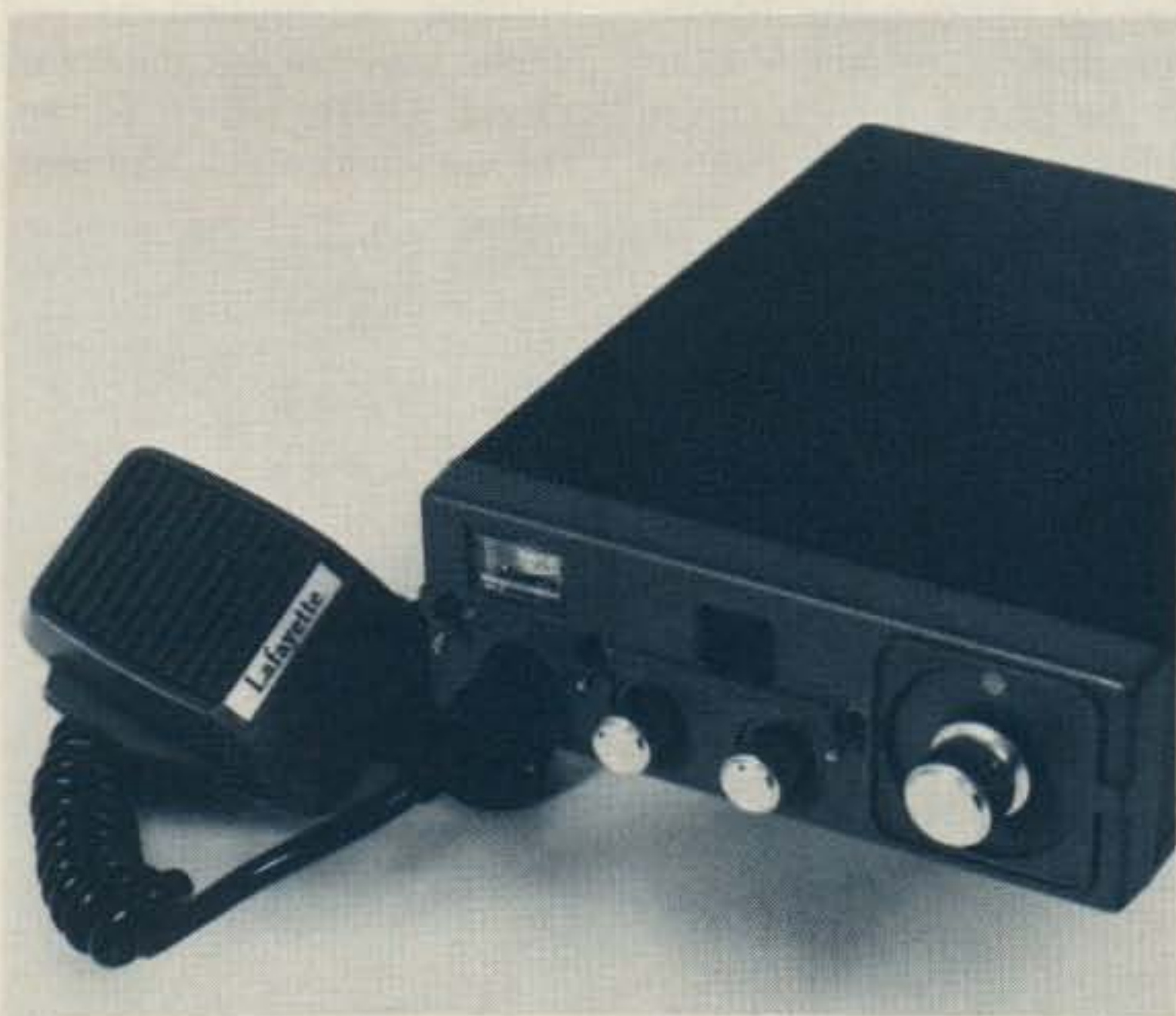
Front view of converted Lafayette rig. The CB channel switch has been replaced with a 10-position rotary. A pair of 7-segment LEDs have been added for direct frequency read-out. Three toggle switches provide display on/off, simplex/repeat, and add 10-kHz to operating frequency.
