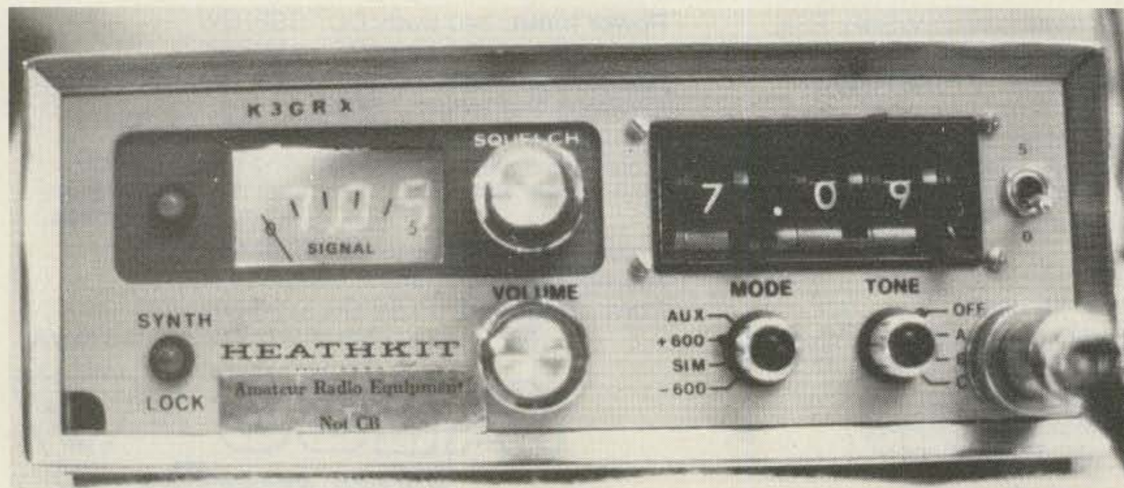
Photo A. Complete installation of frequency display superimposed on S-meter.
