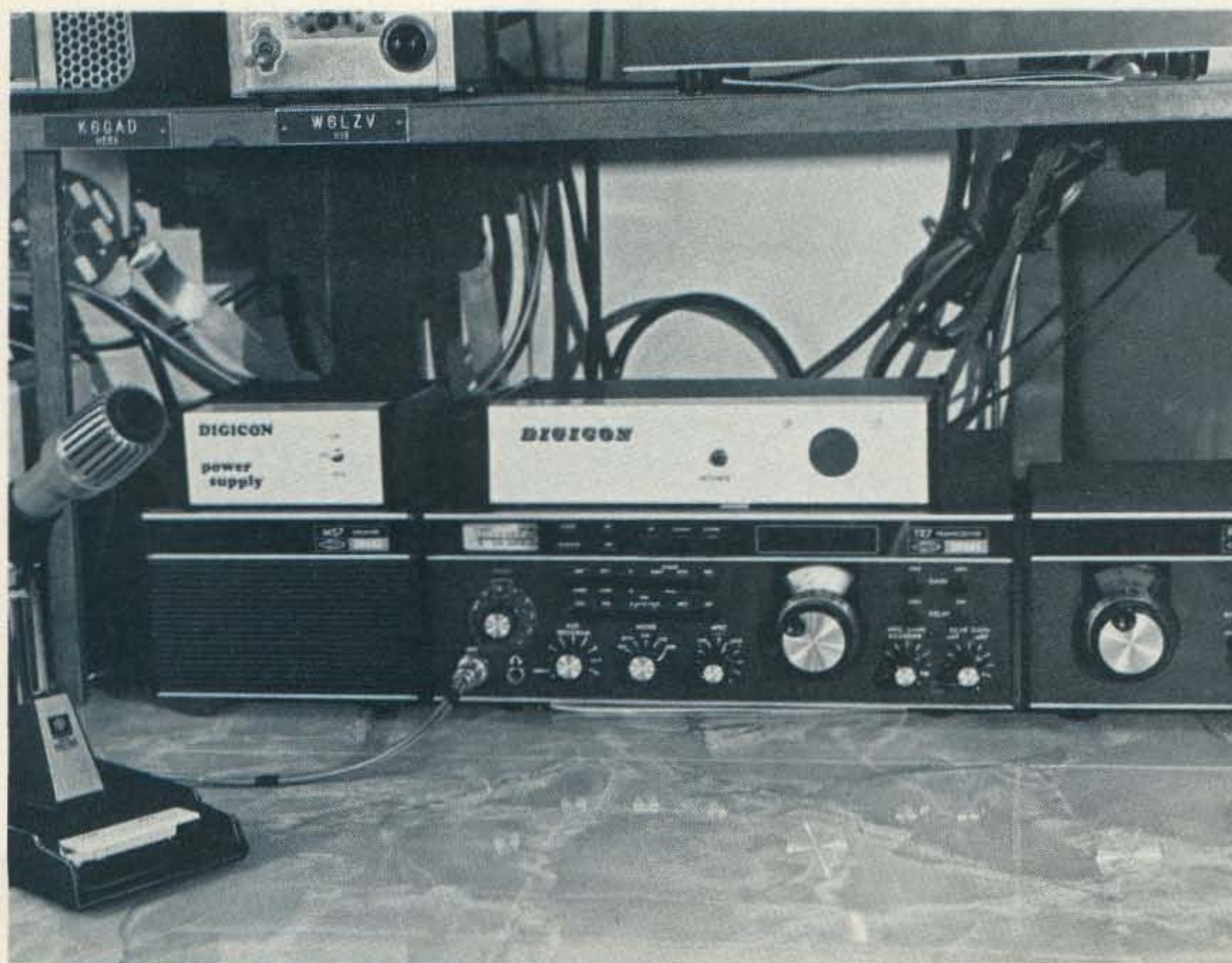
Photo A. The Digital Frequency Display-to-Morse Code Converter (DFD-MCC). The name DIGICON (Digital Converter) was given to my project by W6LZV.
