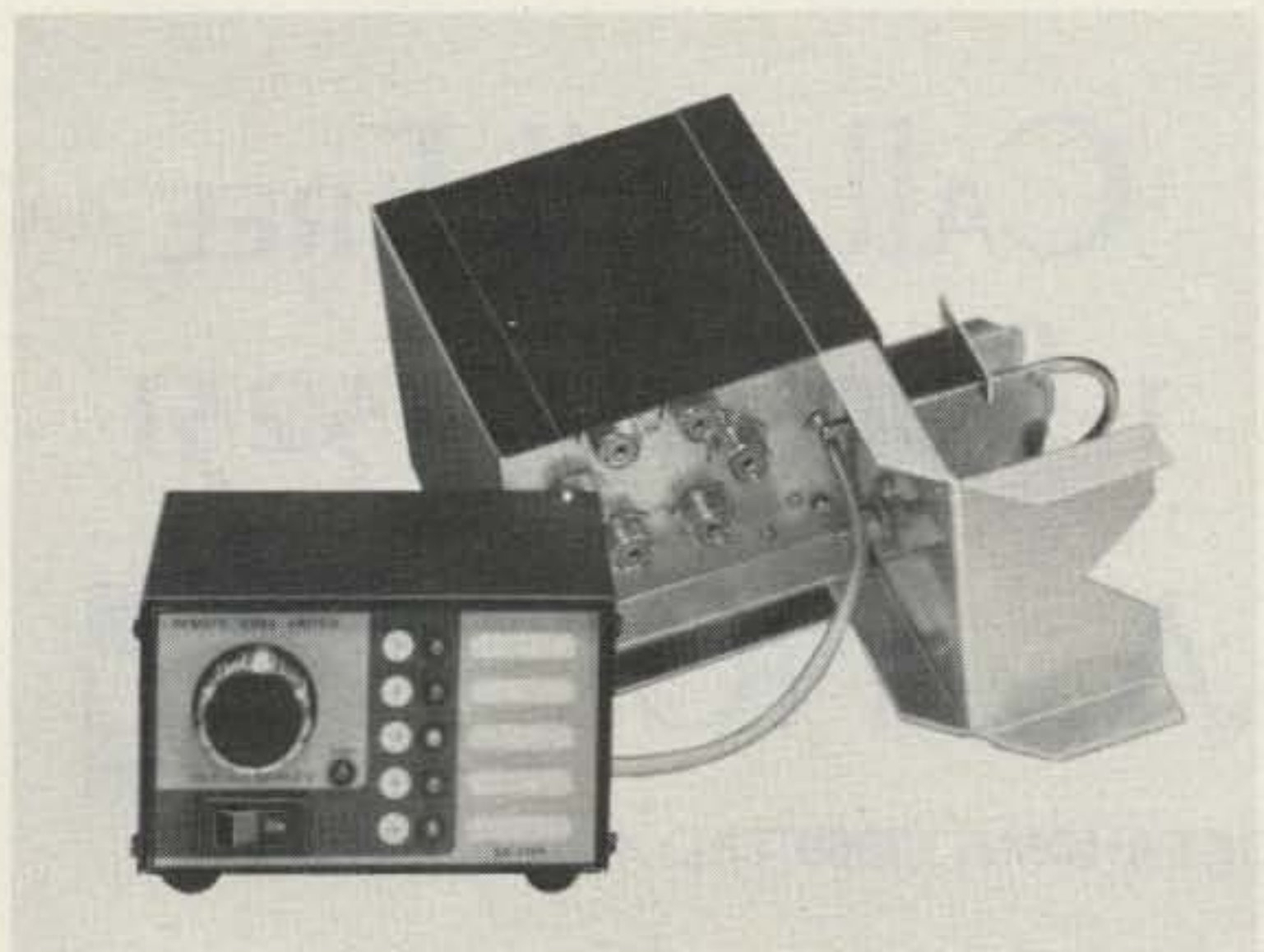
The Heathkit SA-1480 Remote Coax Switch.
