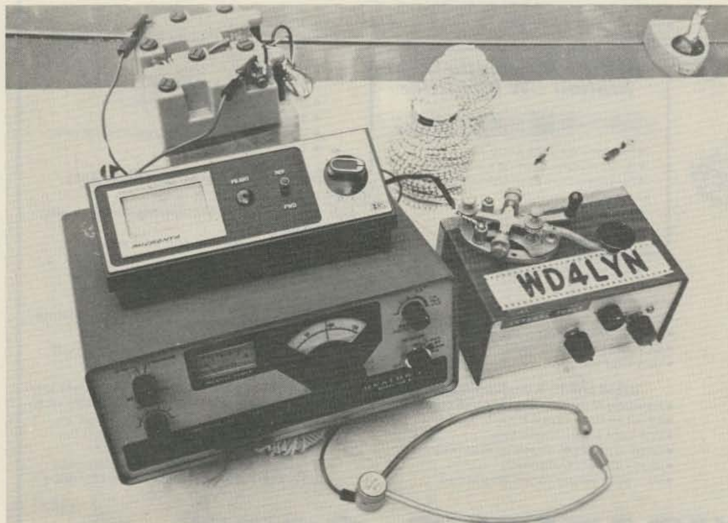
Photo A. The QRP station assembled and ready for packing. Note the antenna and counterpoise (plastic-covered hookup wire) wound on empty vitamin bottles, just behind the key and antenna tuner.
