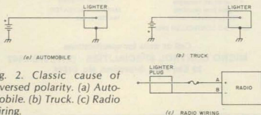
Fig. 2. Classic cause of reversed polarity. (a) Automobile. (b) Truck. (c) Radio wiring.
