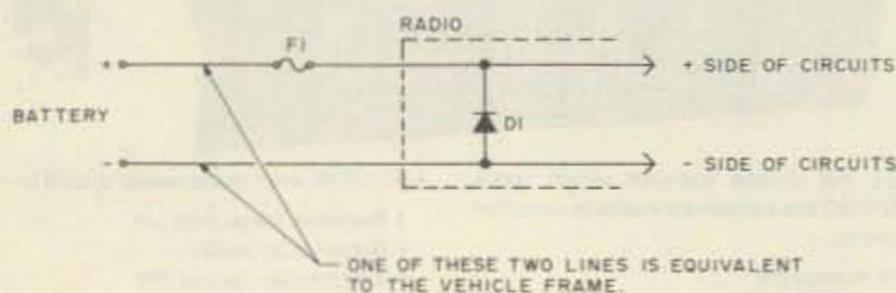
Fig. 1. Typical primary power circuit.
