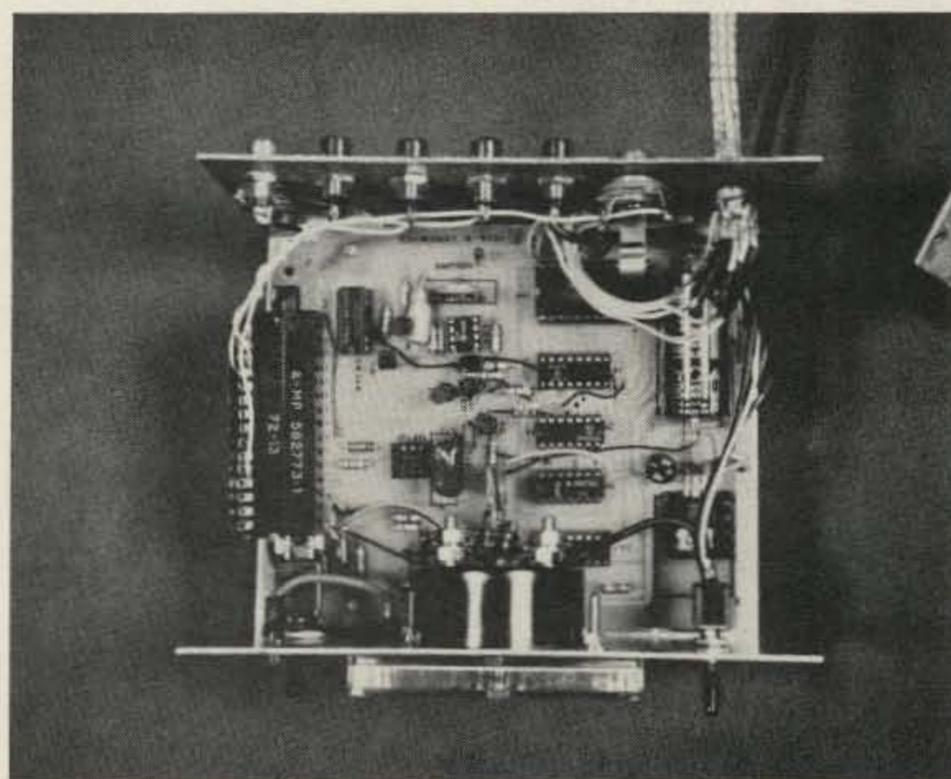
Fig. 5. CW/RTTY converter with the cover removed.
