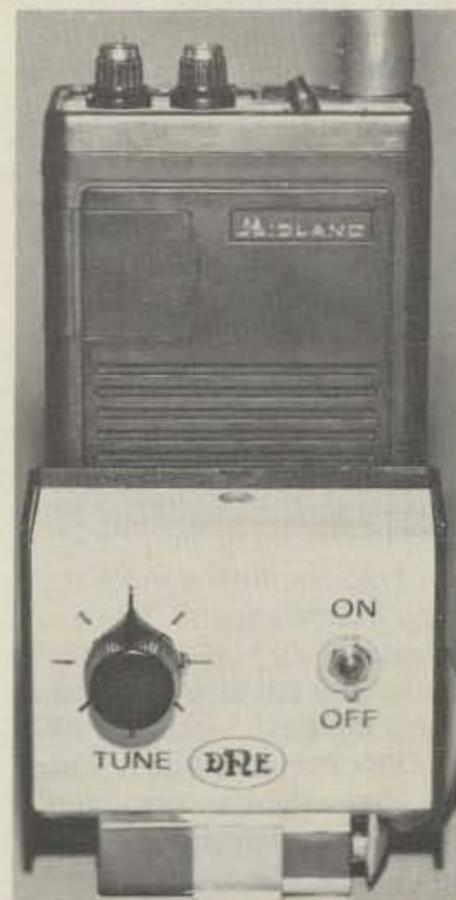
Photo B. The tiny P-20 is designed to fit against a pocket scanner like this Midland.
