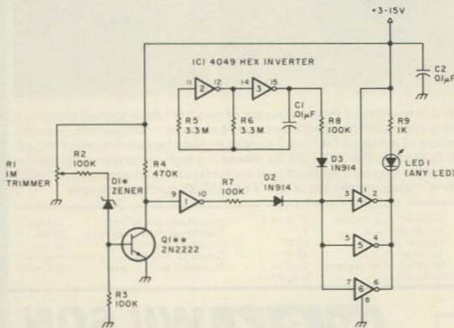
Fig. 2. Pilot light/voltage monitor.
