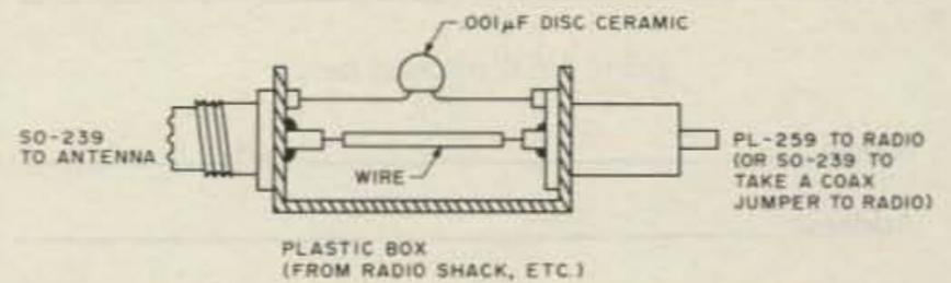
Fig. 6. Dc-isolation in antenna line.
