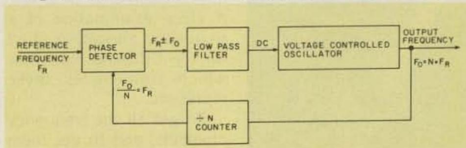
Fig. 2. Block diagram of a more versatile phase-locked loop.
