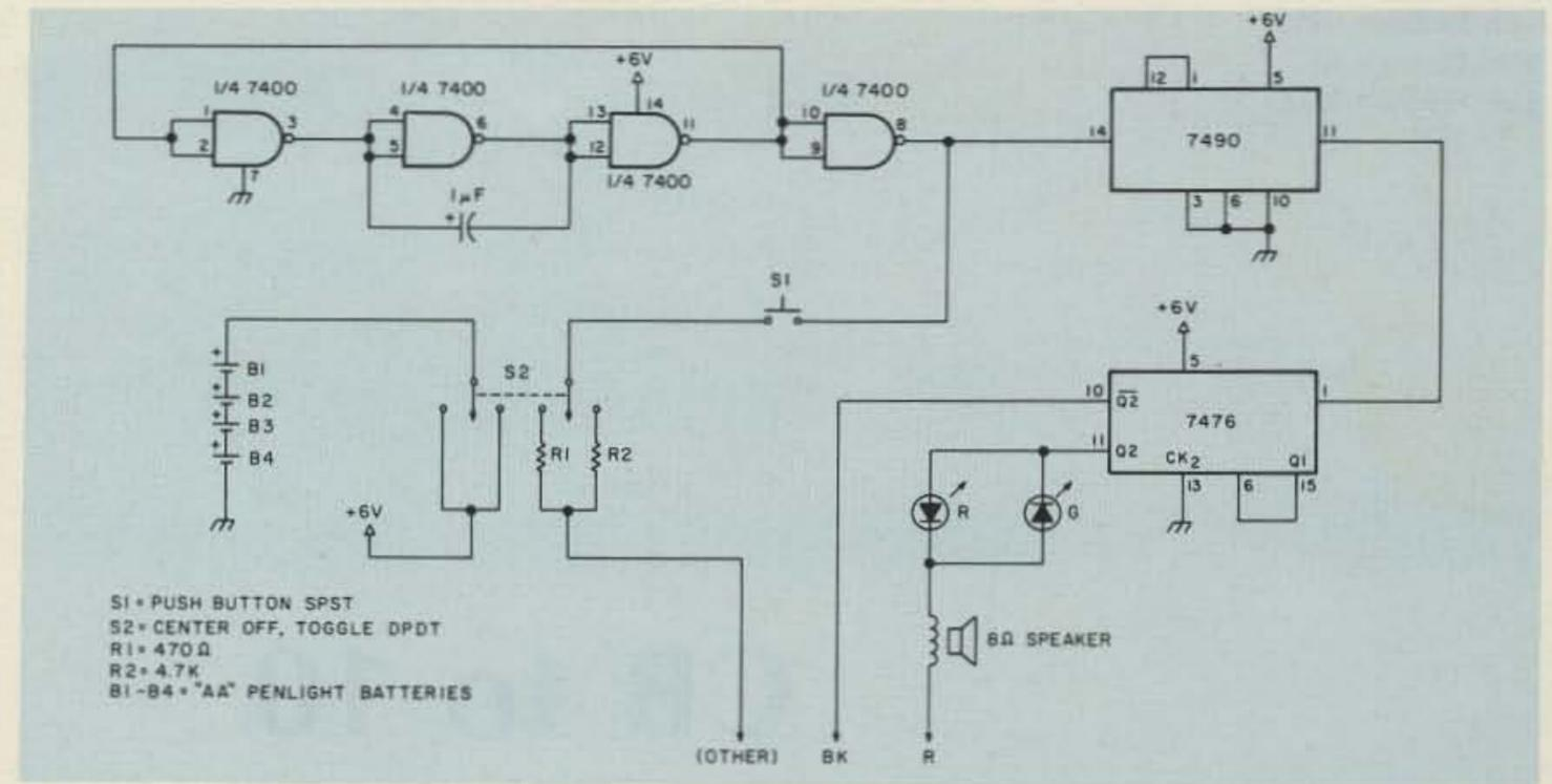
Fig. 1. Transistor tester schematic diagram.
