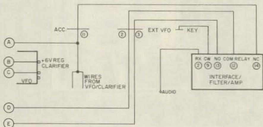
Fig. 8. Interchassis wiring.
