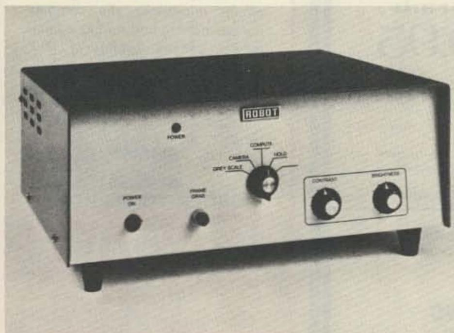
Robot Research's Model 650 scan converter.
