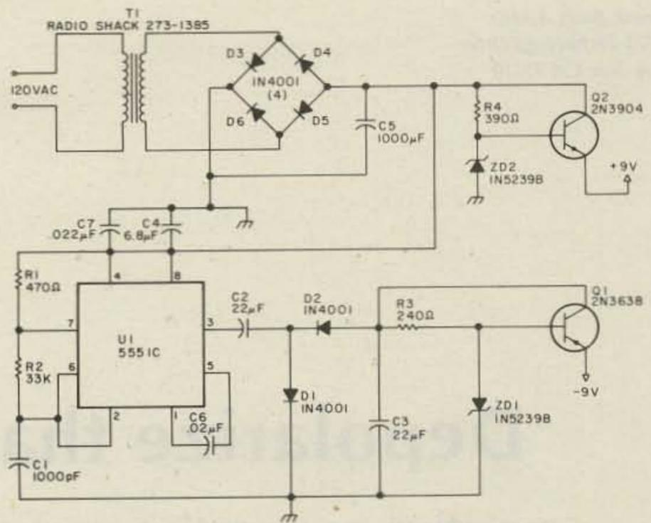
Fig. 4. Complete plus and minus 9-volt power supply.
