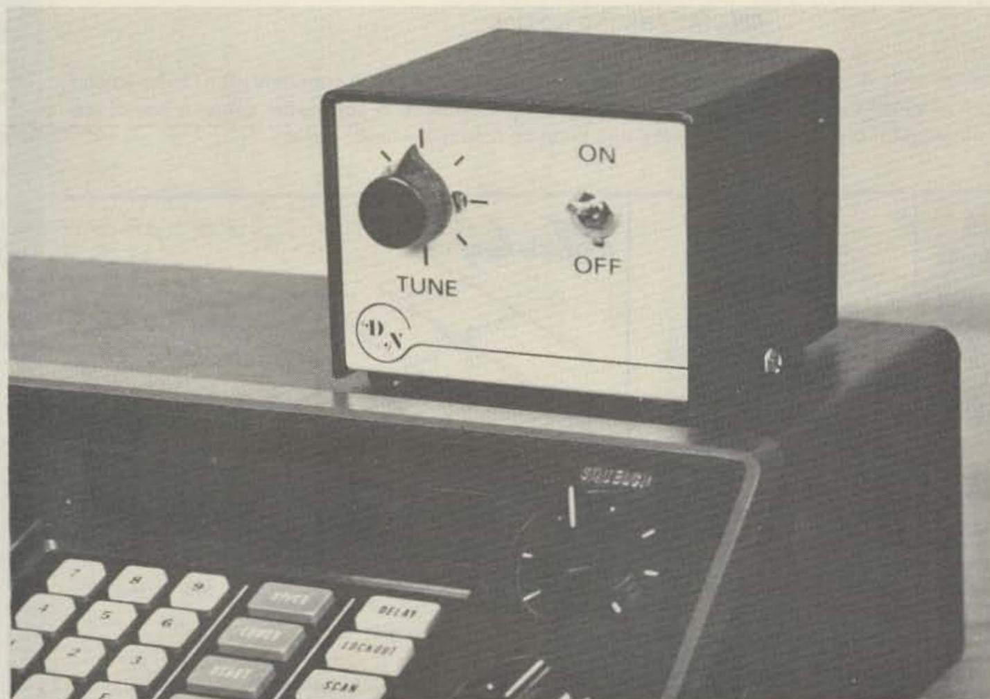
Photo A. The D-12 scramble decoder shown working here with a Bearcat 210 scanner.
