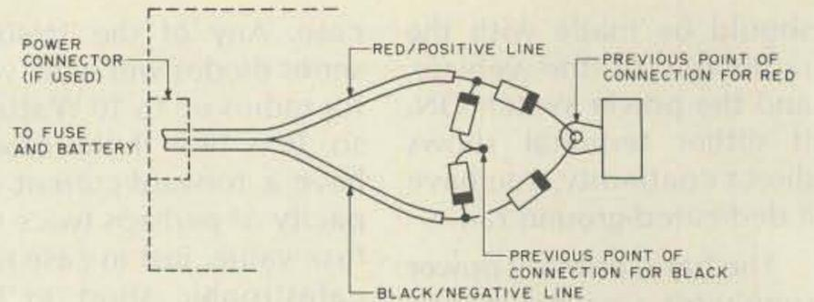
Fig. 7. How to add the bridge inside the radio.
