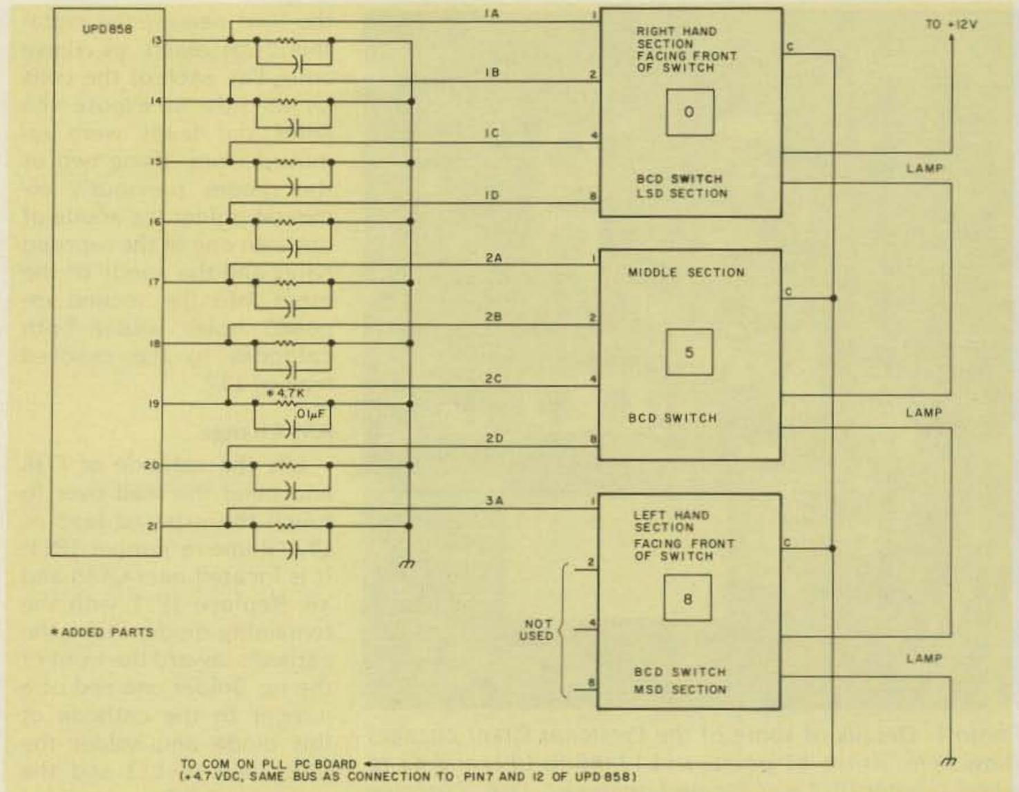
Fig. 8. PLL-to-BCD switch wiring.
