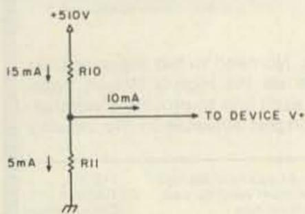
Fig. 1.  $510\text{ V}/15\text{ mA} = R10 + R11 = 34\text{k}$ .  $R10 = (510\text{ volts} - 10\text{ volts})/15\text{ mA} \approx 33\text{k}$ ;  $R11 = 34\text{k} - 33\text{k} = 1\text{k}$ . Therefore,  $R10 = 33\text{k}$  and  $R11 = 1\text{k}$ .
