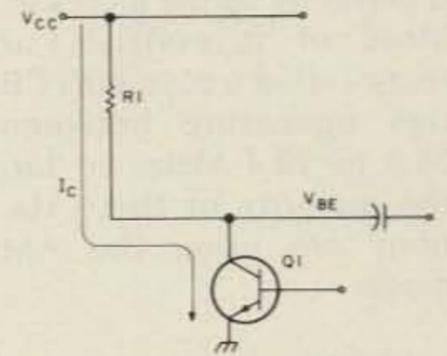
Fig. 6. Too much current through R1 when Q1 is conducting will blow Q1.
