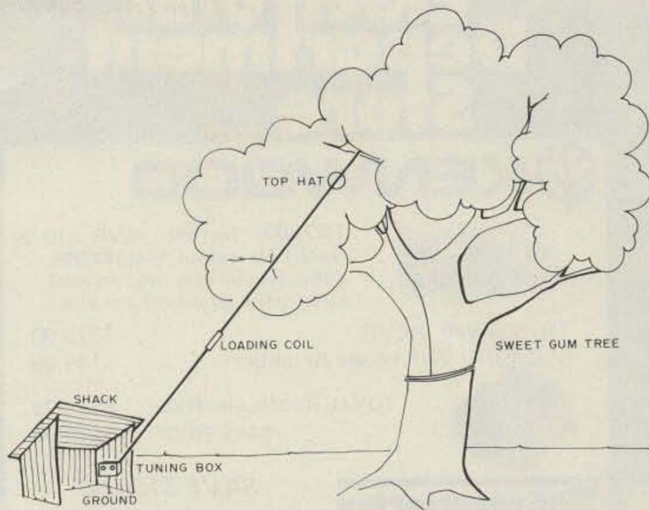
Fig. 3. The AB5S installation.
