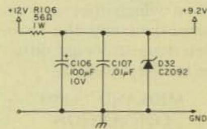
Fig. 6(a). Original regulator circuit.
