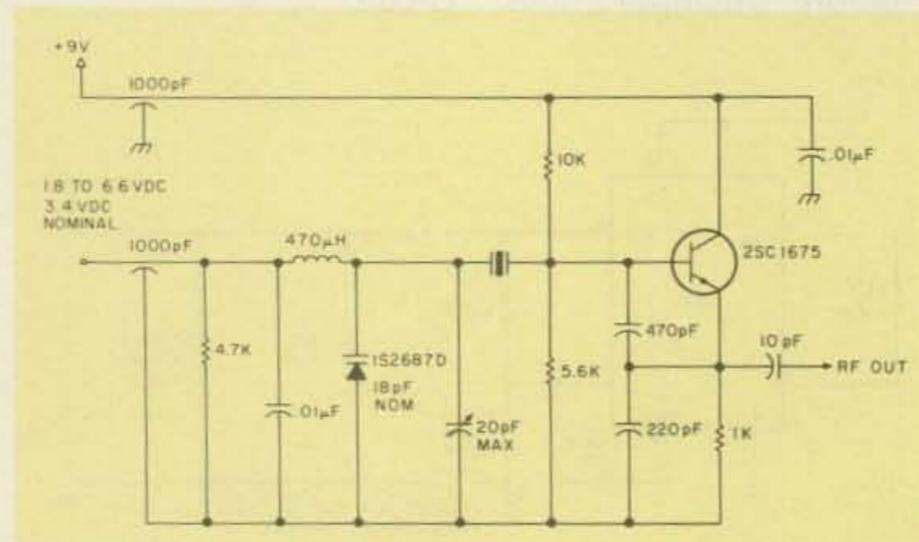
Fig. 7. Crystal-oscillator schematic.
