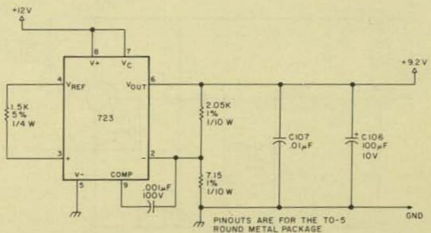
Fig. 6(b). The 723 regulator circuit.
