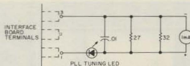
Fig. 4. M-80 board modification for tuning meter.
