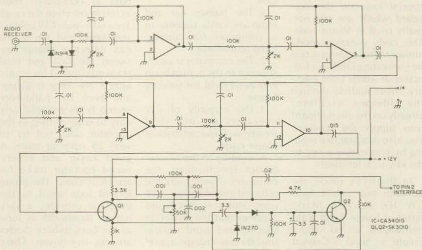
Fig. 3. Filter/amp schematic.
