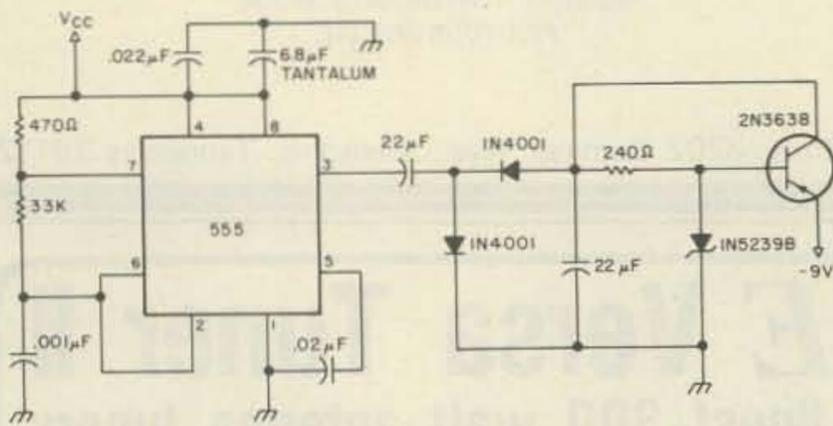
Fig. 1. Original -9-volt power supply.
