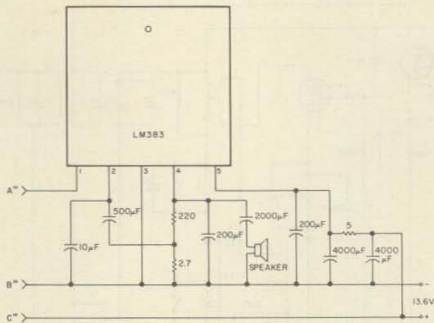
Fig. 4. Audio power amplifier uses Radio Shack LM383.
