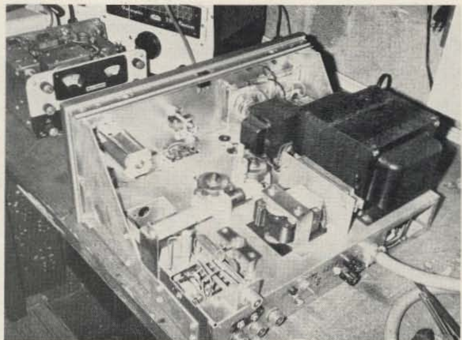
Photo C. The new plate-tune and -load capacitors and modified choke L2 are installed.
