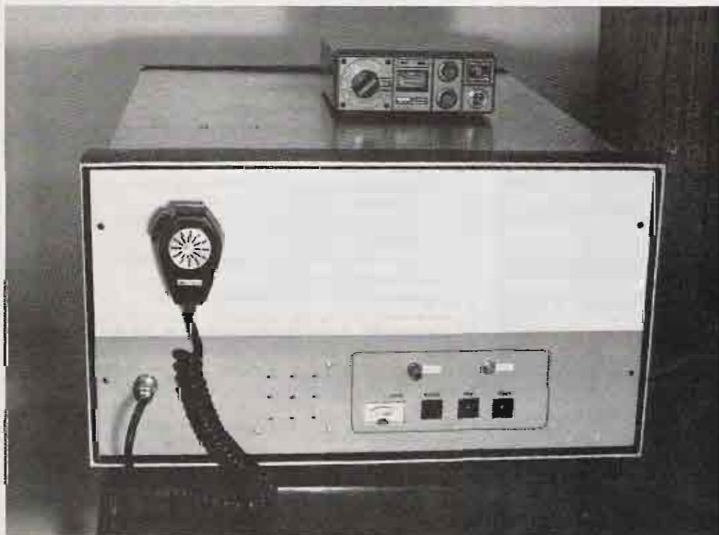
Photo A. Repeater is self-contained inside a 19"-wide cabinet, with the exception of IC-22S two-meter remote base and audio tape cartridge machine (not shown).
