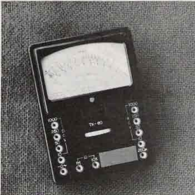
Photo A. The front of the VOM as it originally appeared. It still looks good, but electrically it was falling apart.
