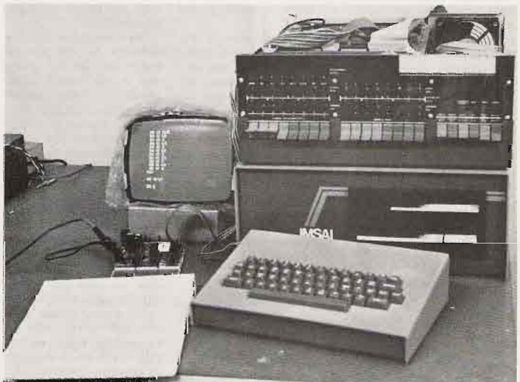
Photo D. Development system consisting of IMSAI 8080, dual floppies, keyboard, and 9" CRT. ROM-simulator boards connect to small dedicated application microcomputers for in-circuit emulation-type software debug.
