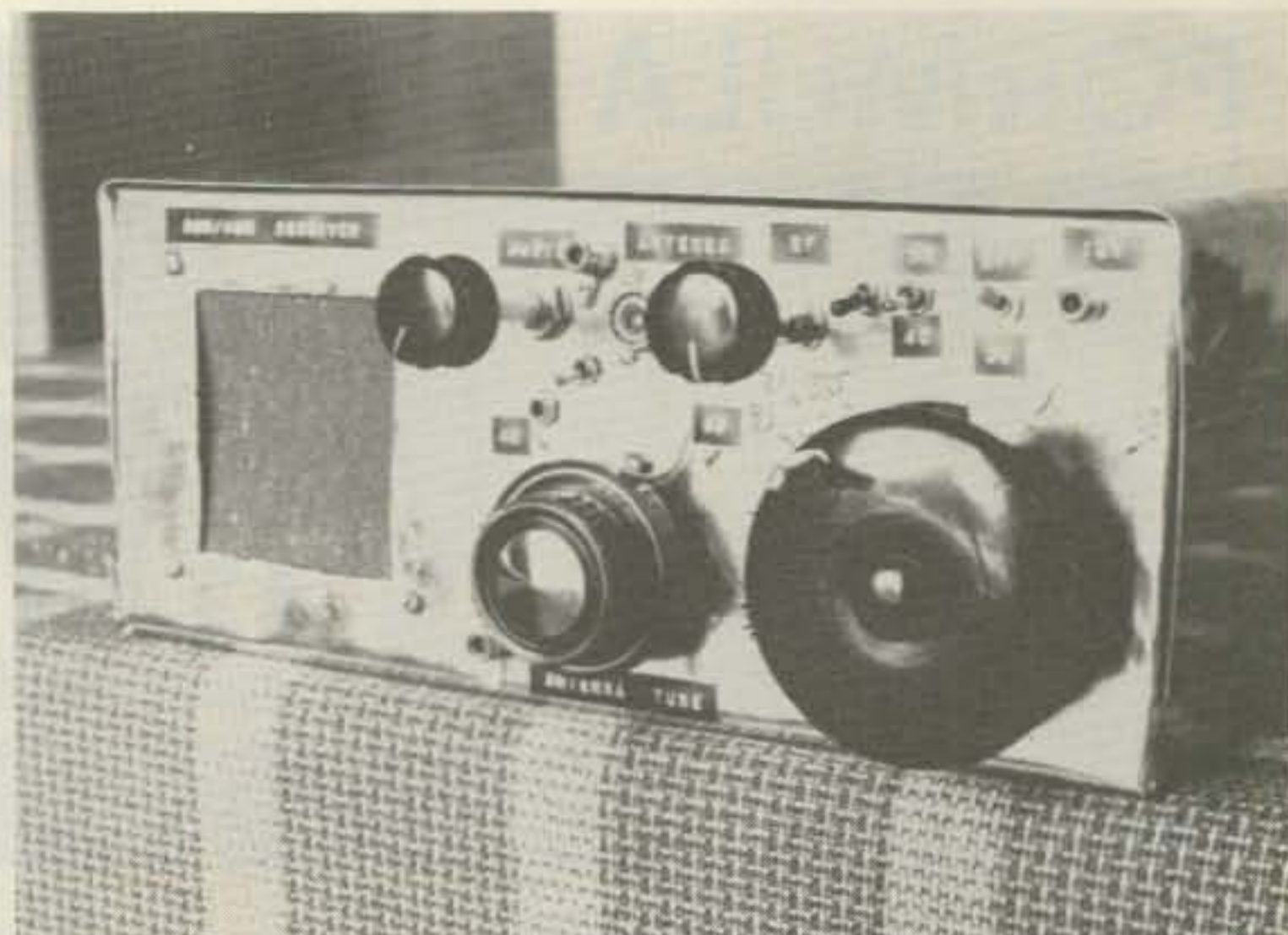
Photo D. Front part of the receiver. The extra switches and sockets are for interfacing with a 5-Watt DSB transmitter.
