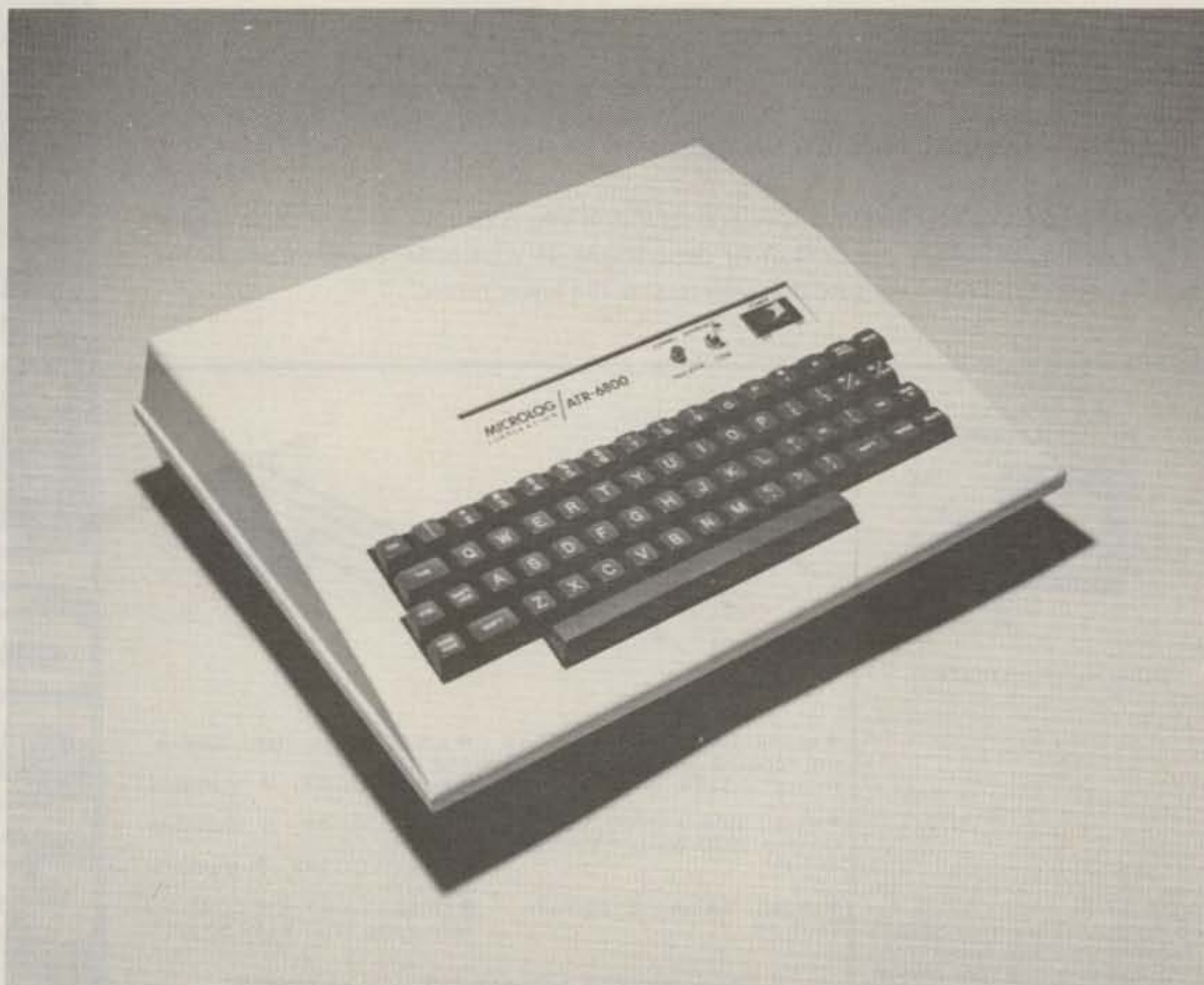
Photo A. The Microlog ATR-6800. On the recessed strip above the keys are (r to l) power switch with integral indicator, reference tone switch, and LED indicator.
