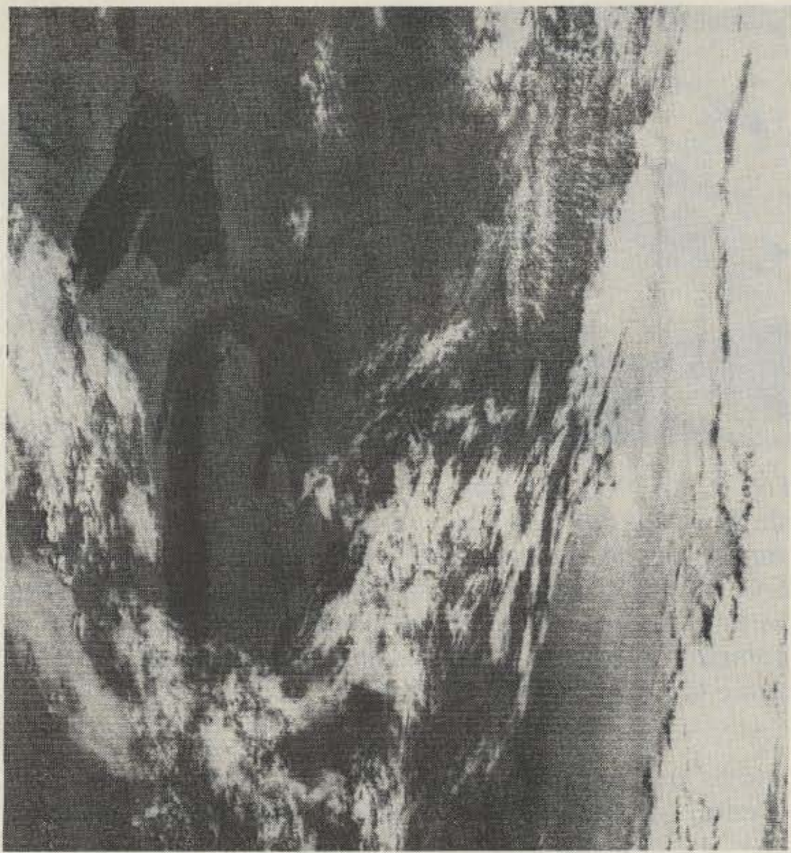
Fig. 7. An NOAA pass displayed on the WB8DQT direct-printing GOES facsimile recorder without changing the 40-rpm carriage drive motor. Note the vertical "stretching" of the display. The use of a 20-rpm motor will provide the proper aspect ratio with this machine (see Fig. 1).
