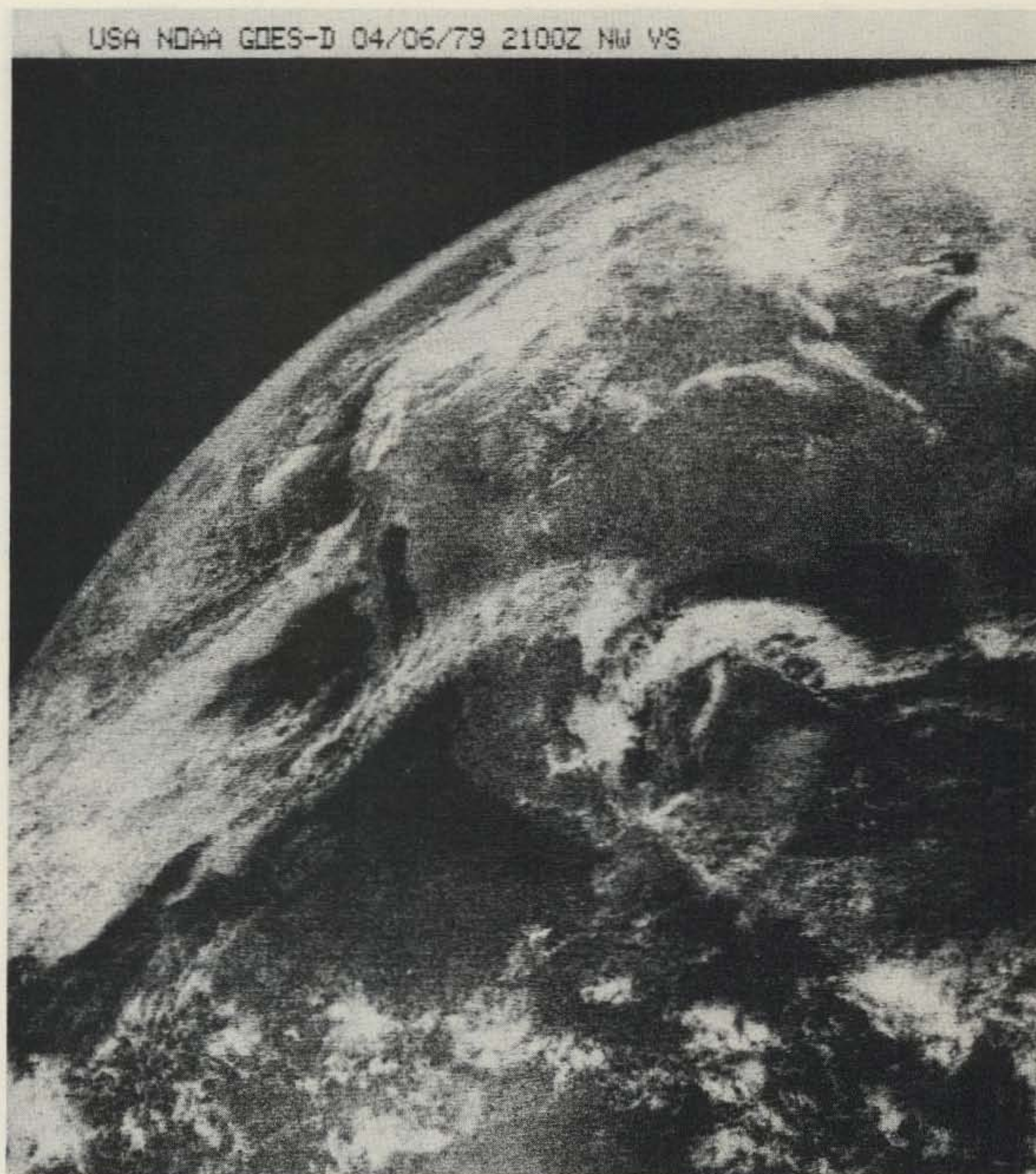
Fig. 2. An example of visible light imagery (GOES D, a replacement for GOES E) printed on the FX-2E direct-printing fax recorder. GOES D had drifted several degrees north of the equator when this picture was acquired and the downlink signal was noticeably noisy. Despite this, the machine printed a quite acceptable picture.
