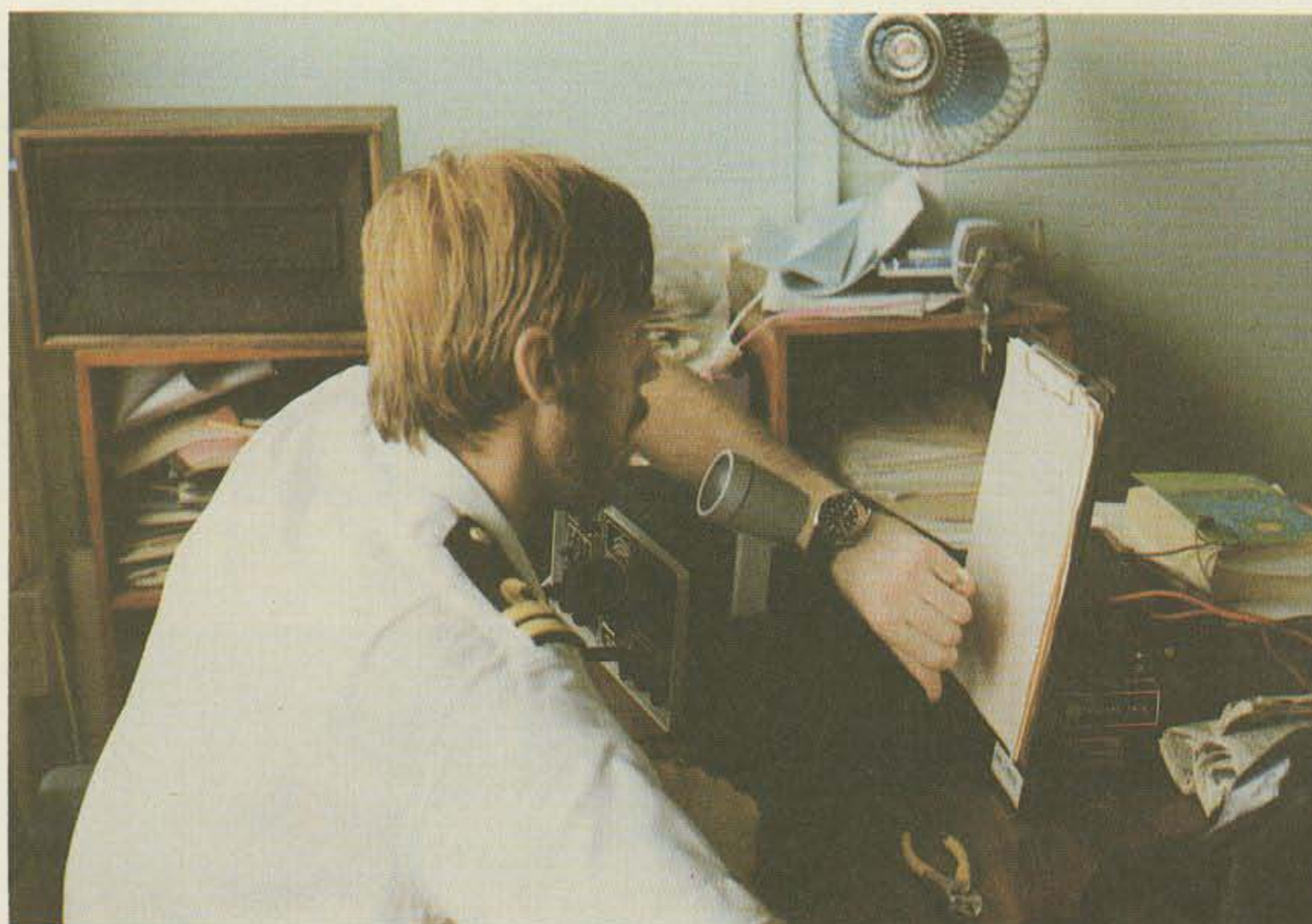
This British naval officer from the Glasgow used ham radio to keep in touch with his ship. St. Lucia's hilly terrain made a VHF link impossible, so 40 meters was used.
