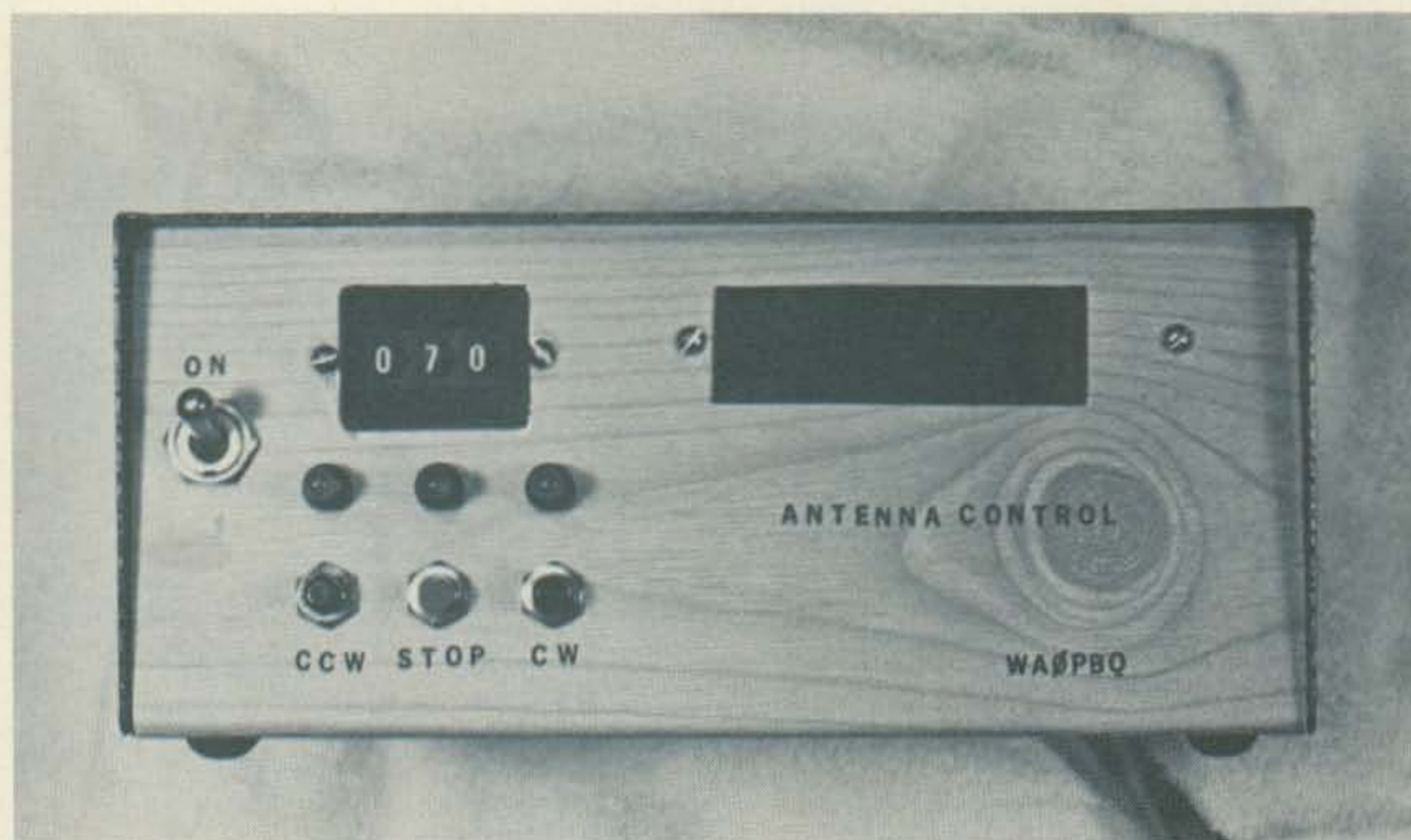
Photo A. Front view of the digital rotator control. Thumbwheel switches for selecting the desired heading are at upper left. LED readouts are behind a red plastic filter at upper right. At lower left are three push-buttons for ccw and cw rotation manually. Discrete LEDs above each push-button indicate the status of the control.
