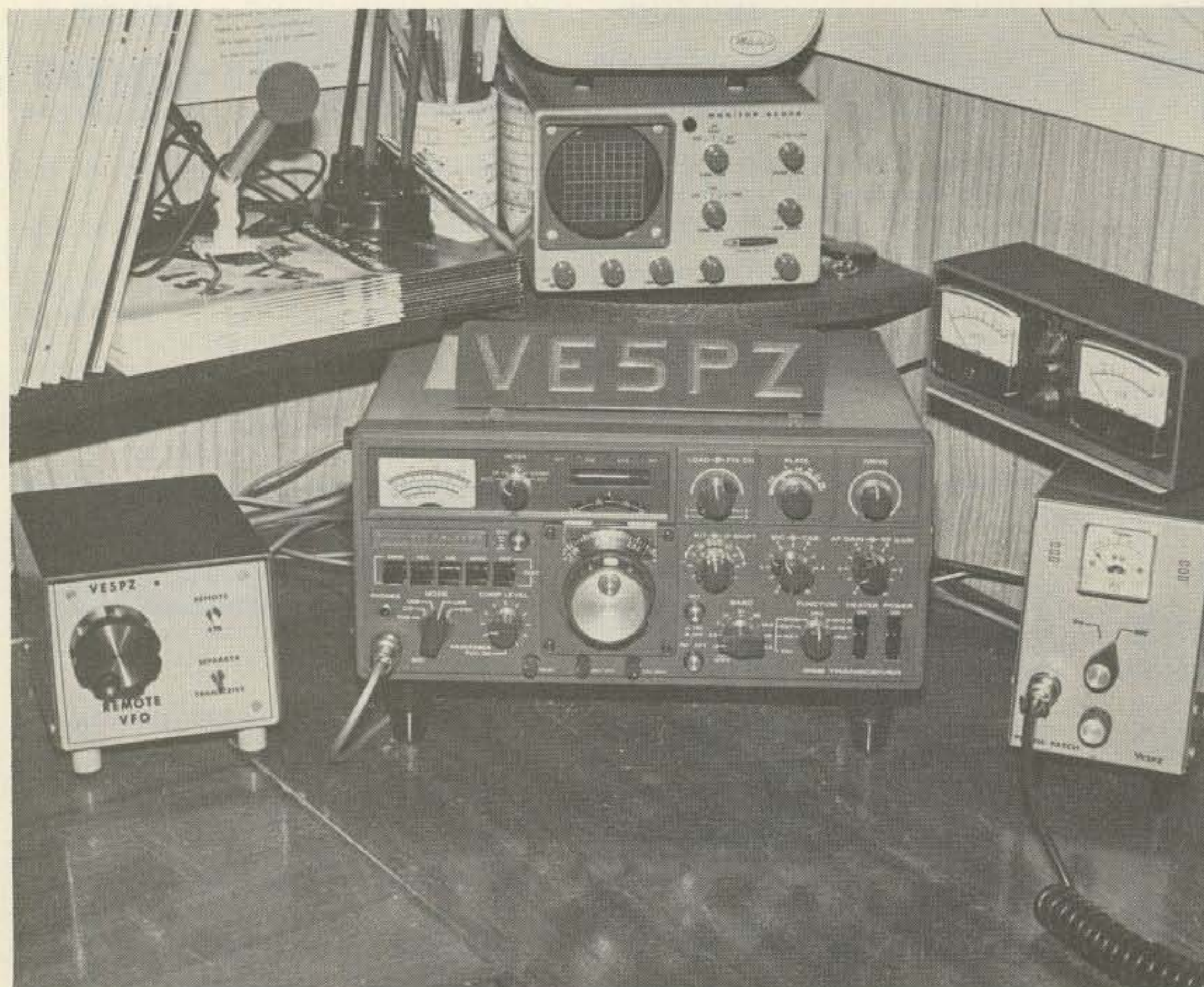
Photo A. The completed remote vfo.
