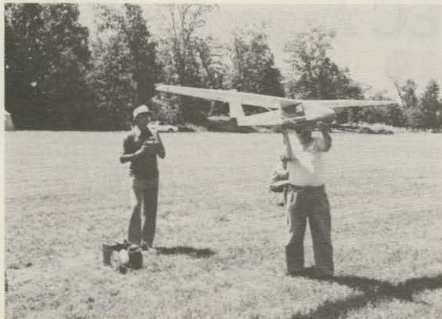
Gene Shelkey from Scottdale, Pennsylvania, gets some help to launch his scale-model Schweitzer sailplane. It is an 11-foot span, 6½-pound flying weight craft complete with pilot figure and full interior.
