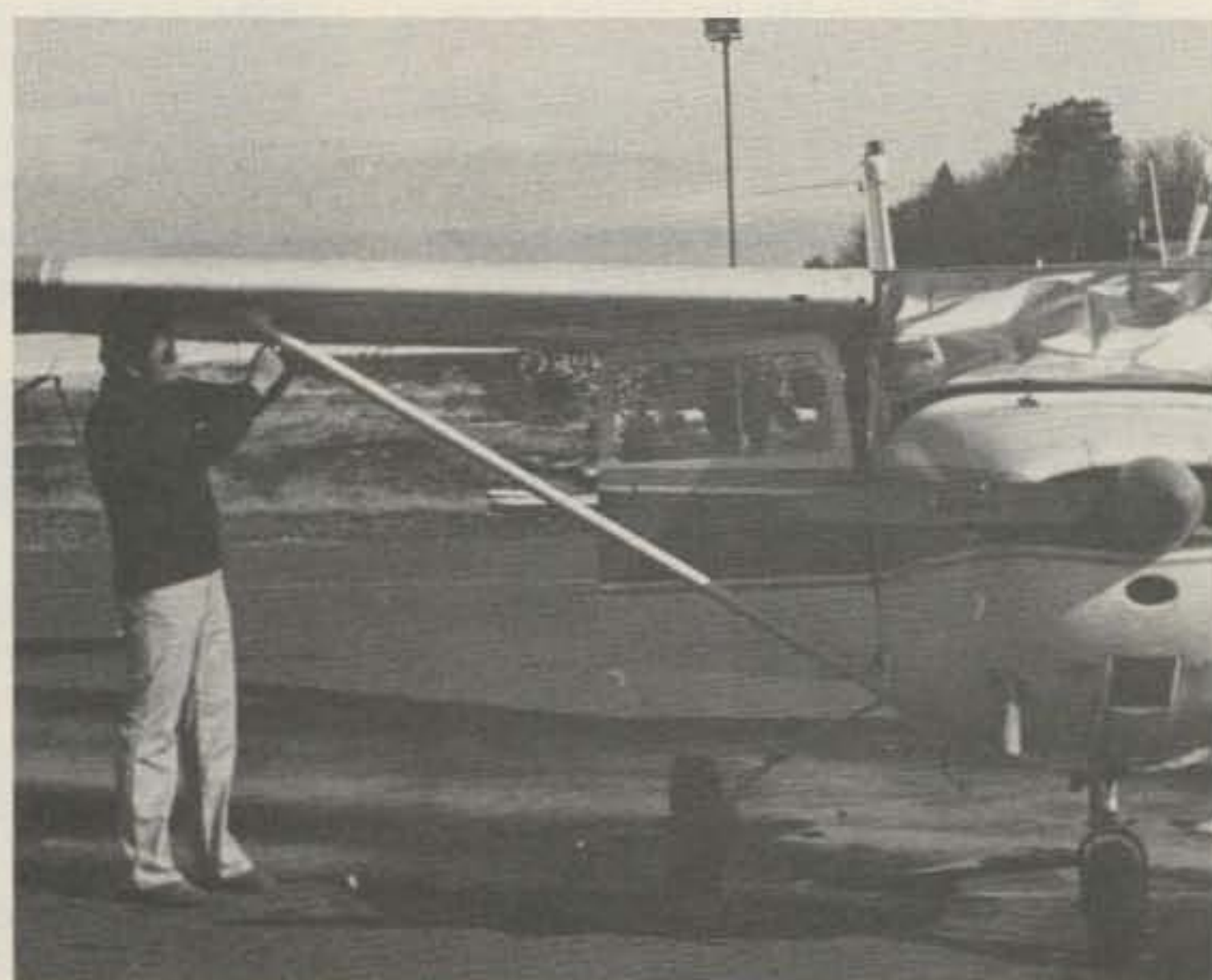
Photo B. Installing a temporary antenna mount onto the tie-down ring.
