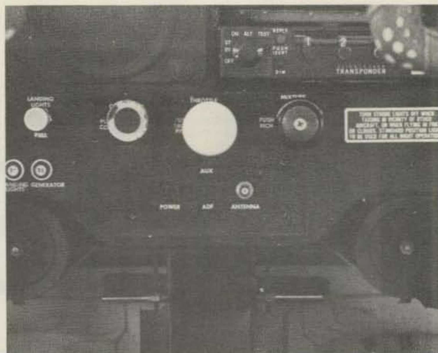
Photo G. A power and antenna patch panel mounted in a Cessna 172.
