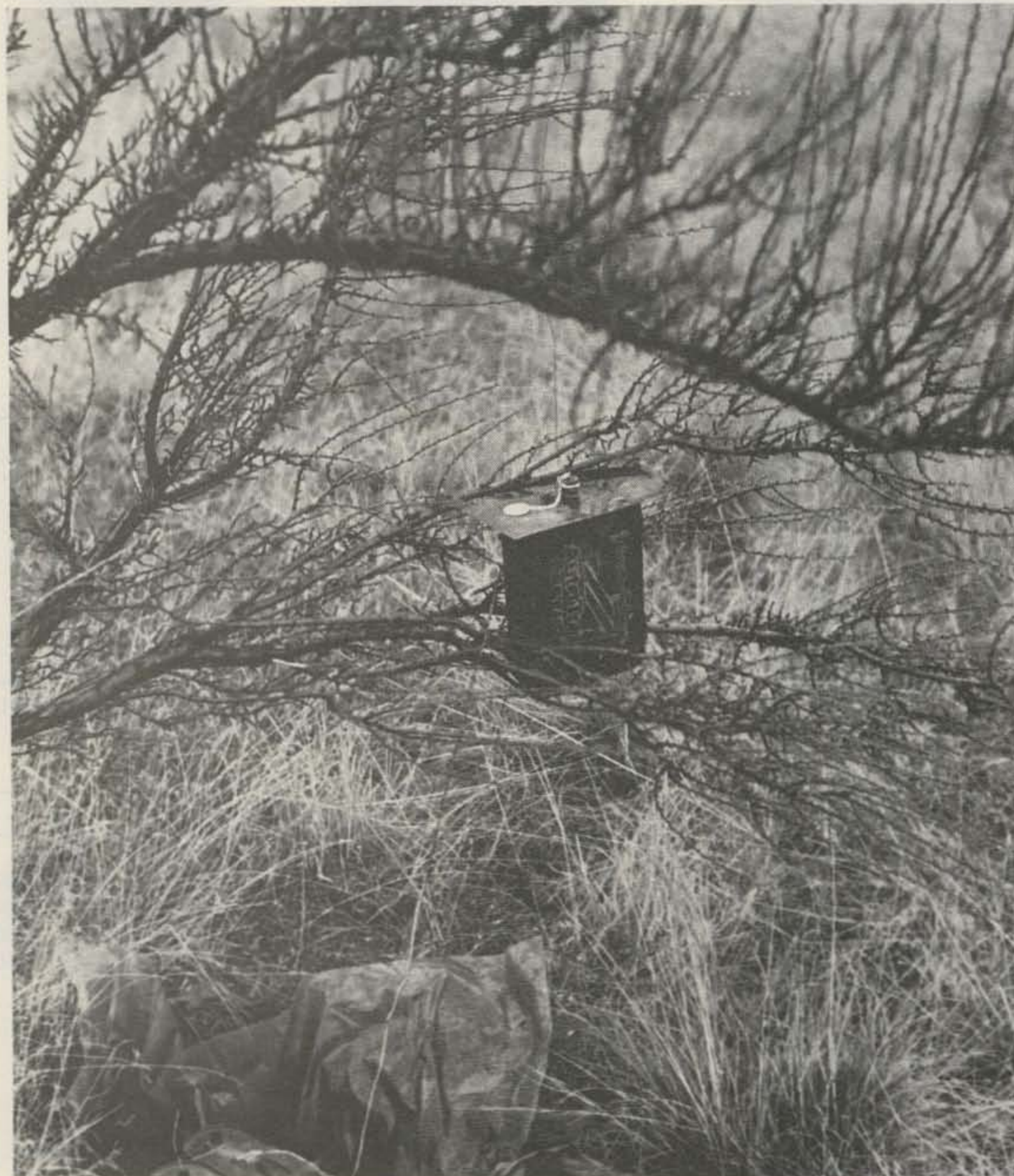
Photo A. The jamming transmitter in the sagebrush, enclosed in a black-painted first-aid box. Wires lead to the plastic-wrapped, buried batteries.
