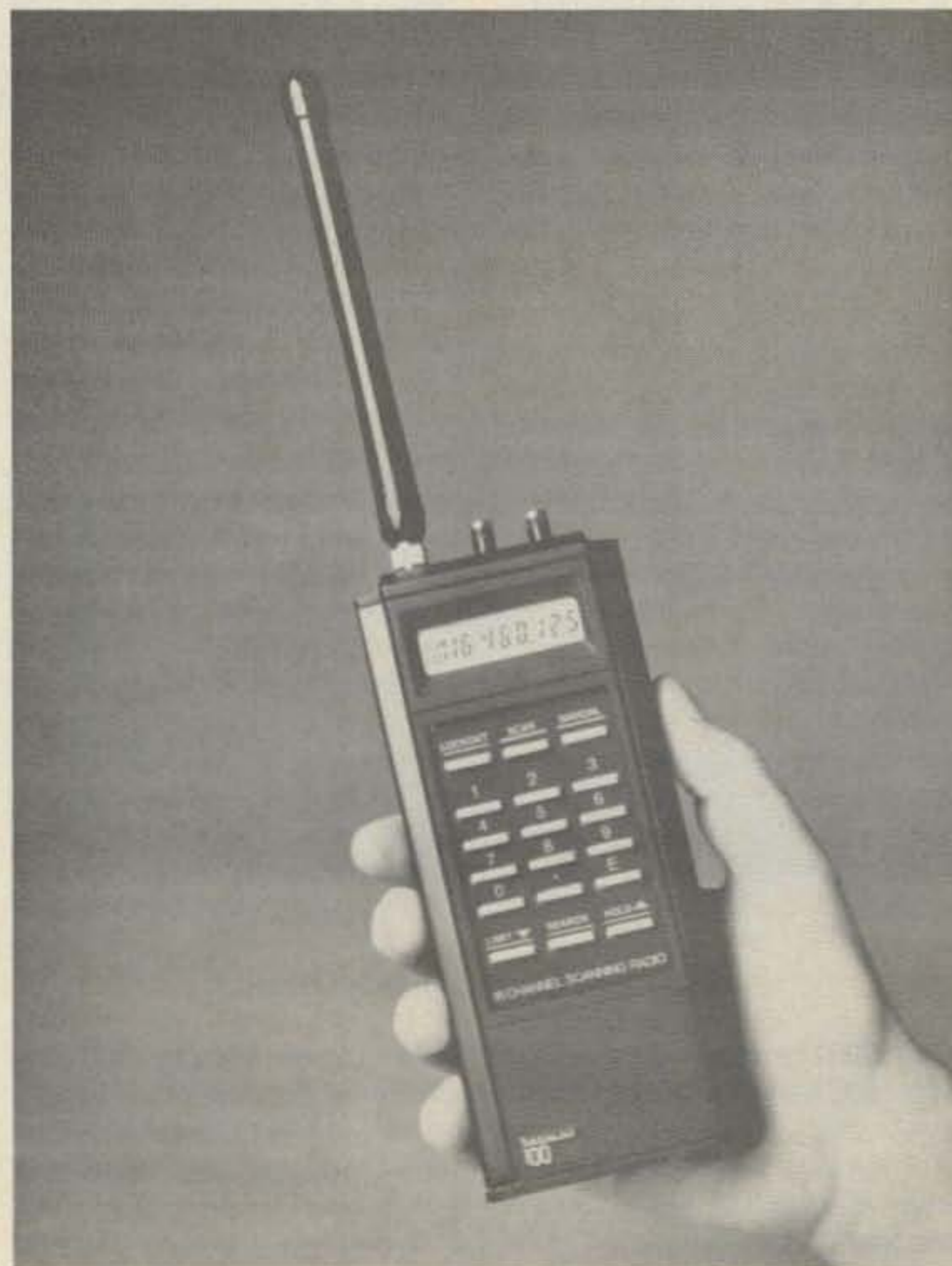
Bearcat's hand-held synthesized scanner.
