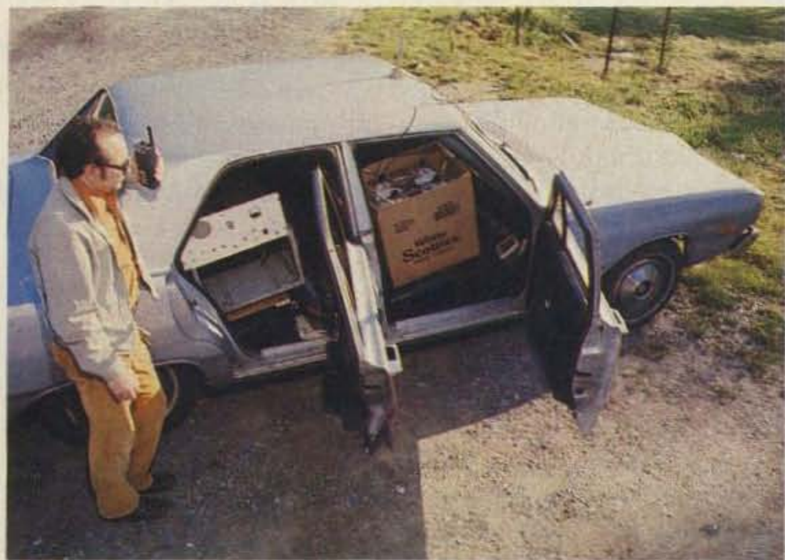
Frank N3RZ stands next to his portable repeater, a .70/.30 220 repeater linked to the main .40/.64 machine to extend coverage. The duplexer is in front seat, the machine and battery in the back, and the antenna is on the car roof.
