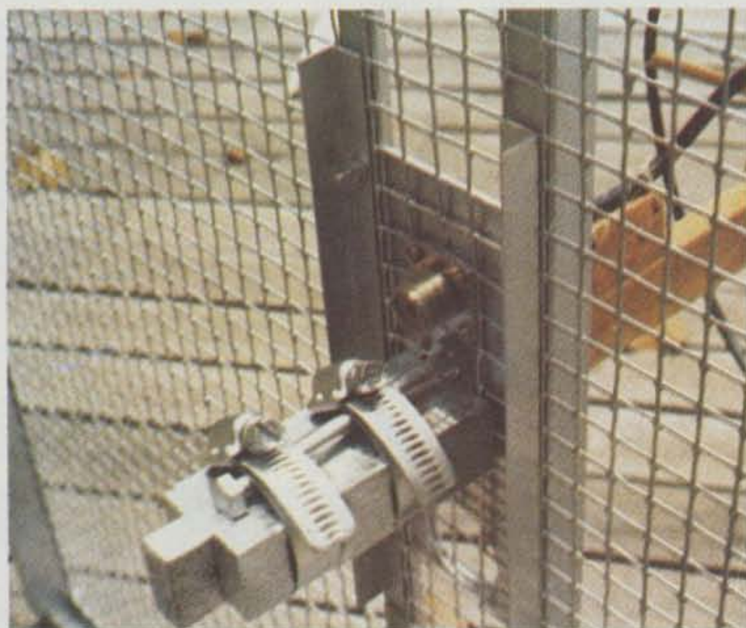
Securing the boom to the reflector.
