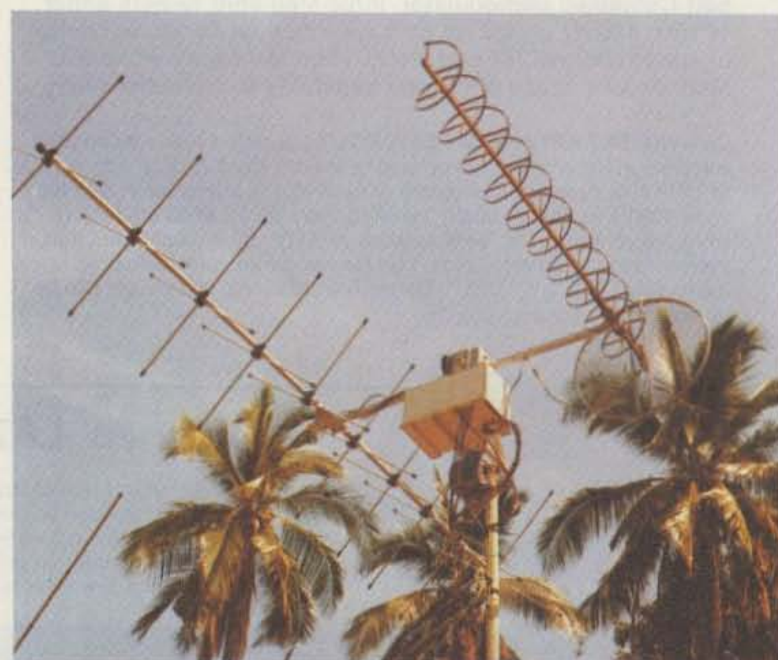
The helical at work—note that the reflector frame is now a lightweight bicycle wheel rim, which is "neater, lighter, and better looking."
