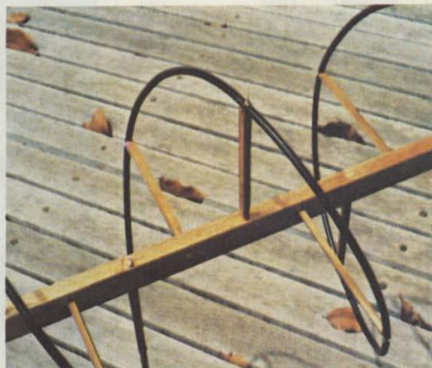
The helix attached to the "chopstick" spacers.
