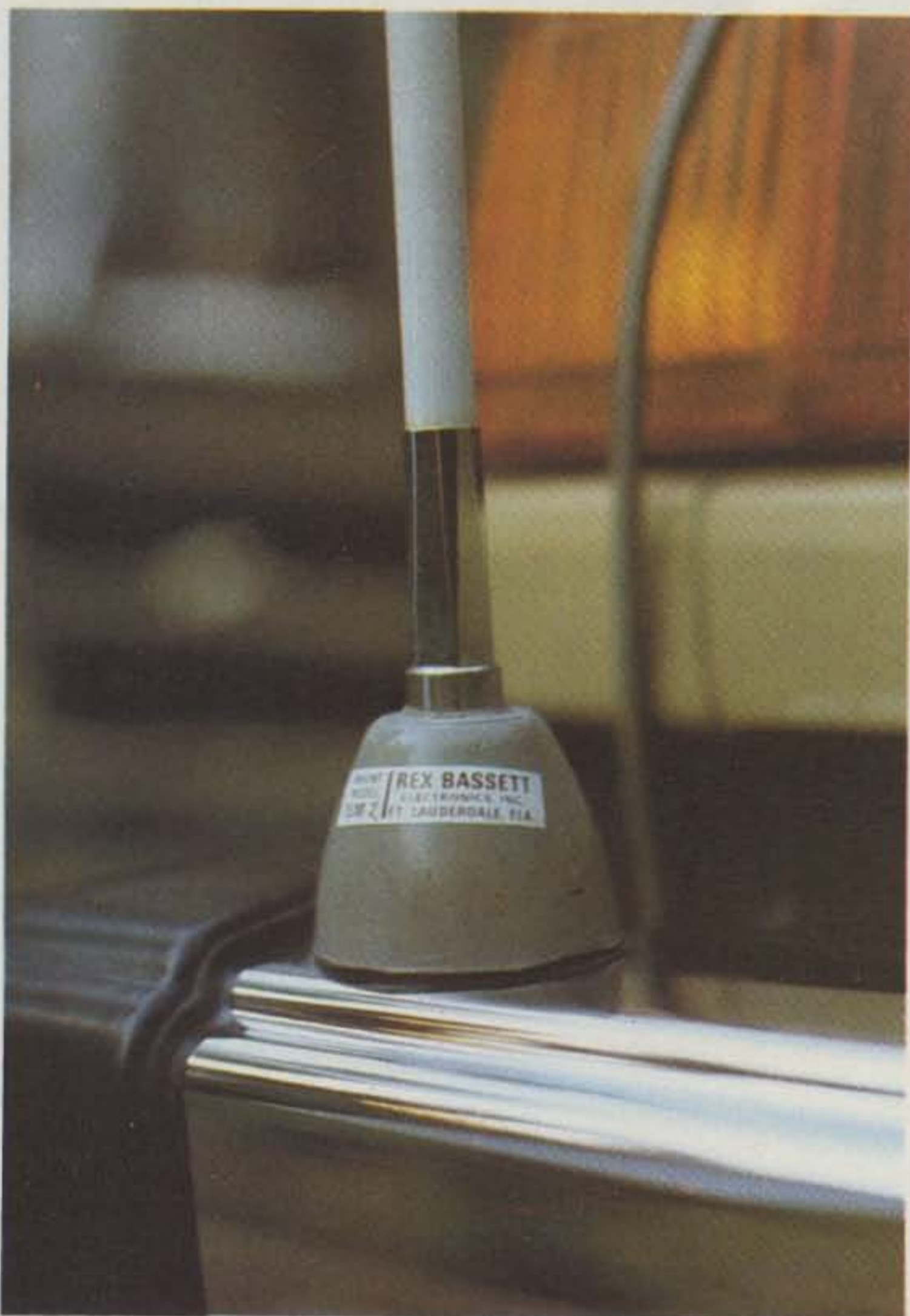
The Rex Bassett TLM-2 mobile mount, with a VAC-20 antenna.
