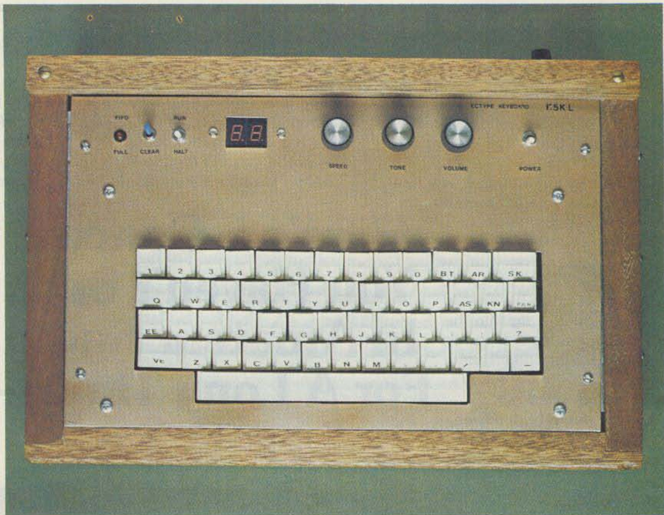
Photo A. Aluminum angle stock bolted to the sides supports aluminum top, bottom, and rear panels. The top was painted with epoxy spray enamel; clear epoxy protects the transfer lettering on the keys and controls. The digital display is for the QRR, QRS digital speed indicator. (See article by W7BBX, 73 Magazine, June, 1980, p. 50).
