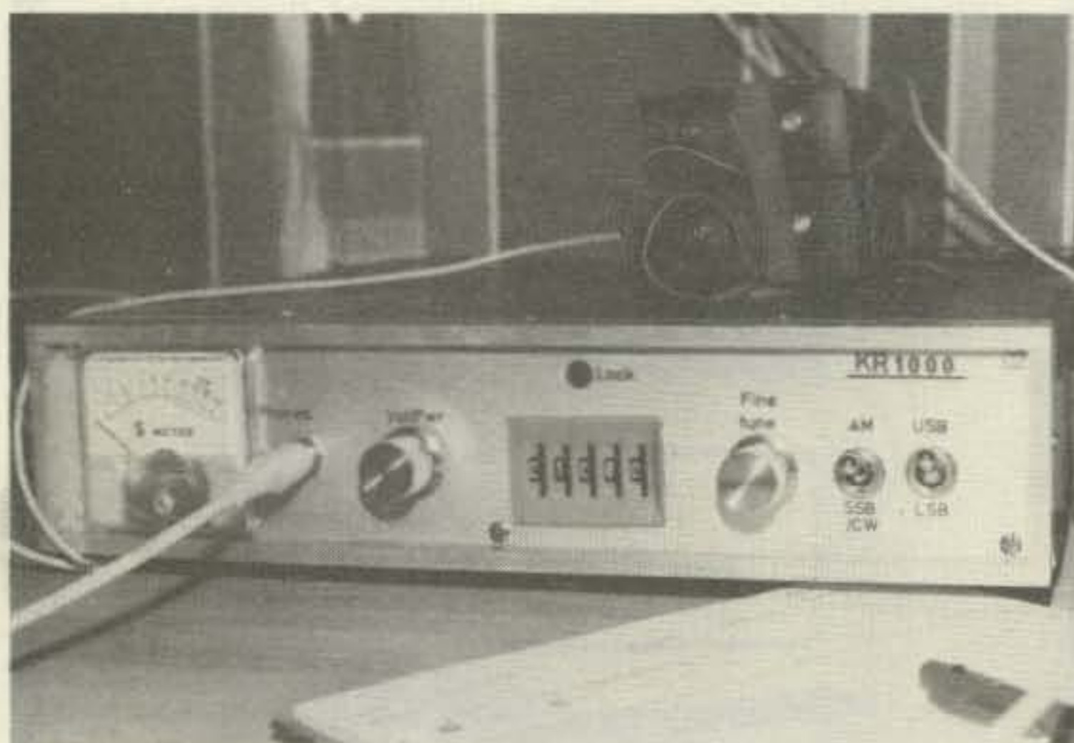
Photo A. Direct thumbwheel-switch readout on the prototype KR 1000. (Photo by ZL4LM)
