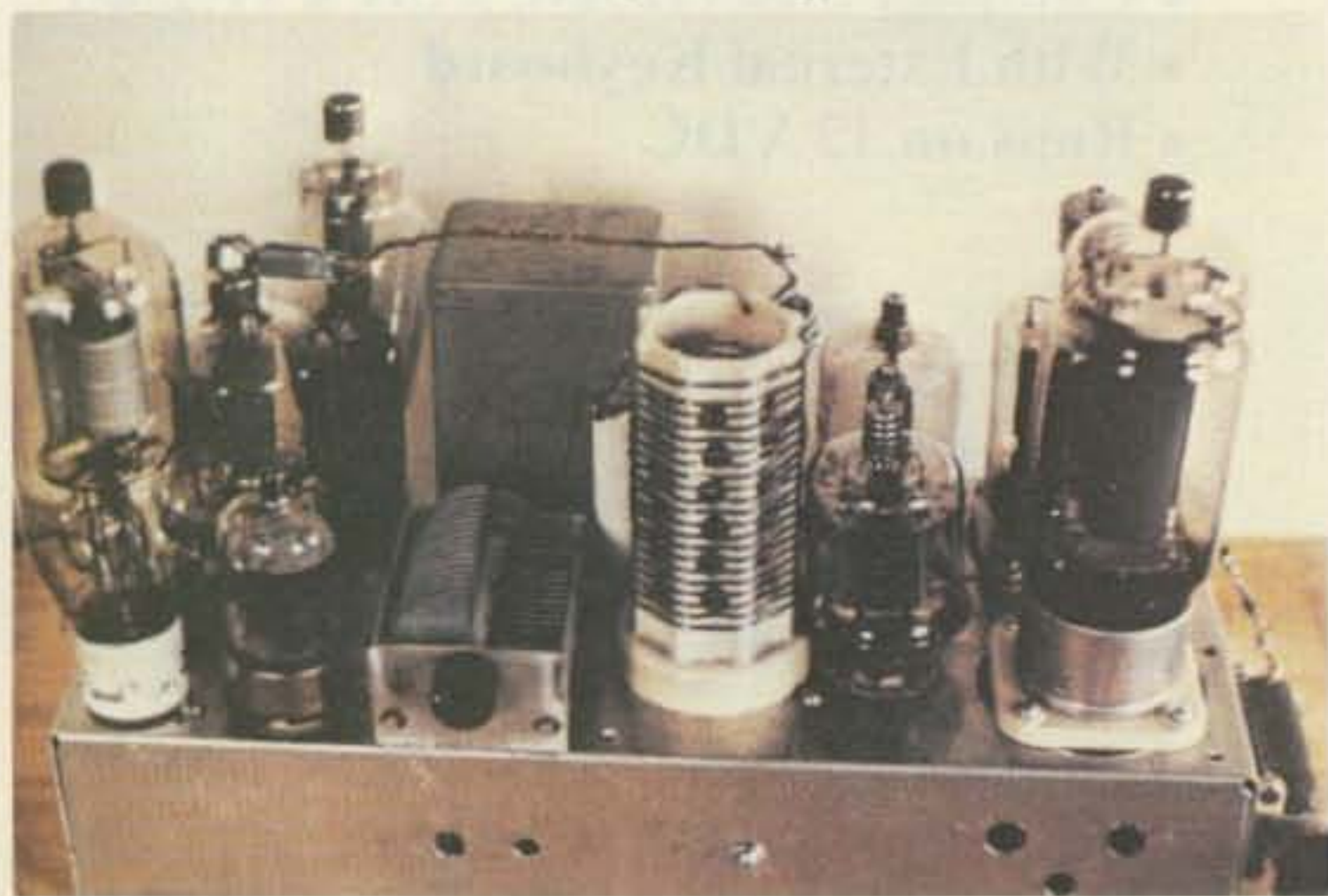
The amplifier test chassis! Only one tube is used at a time.
