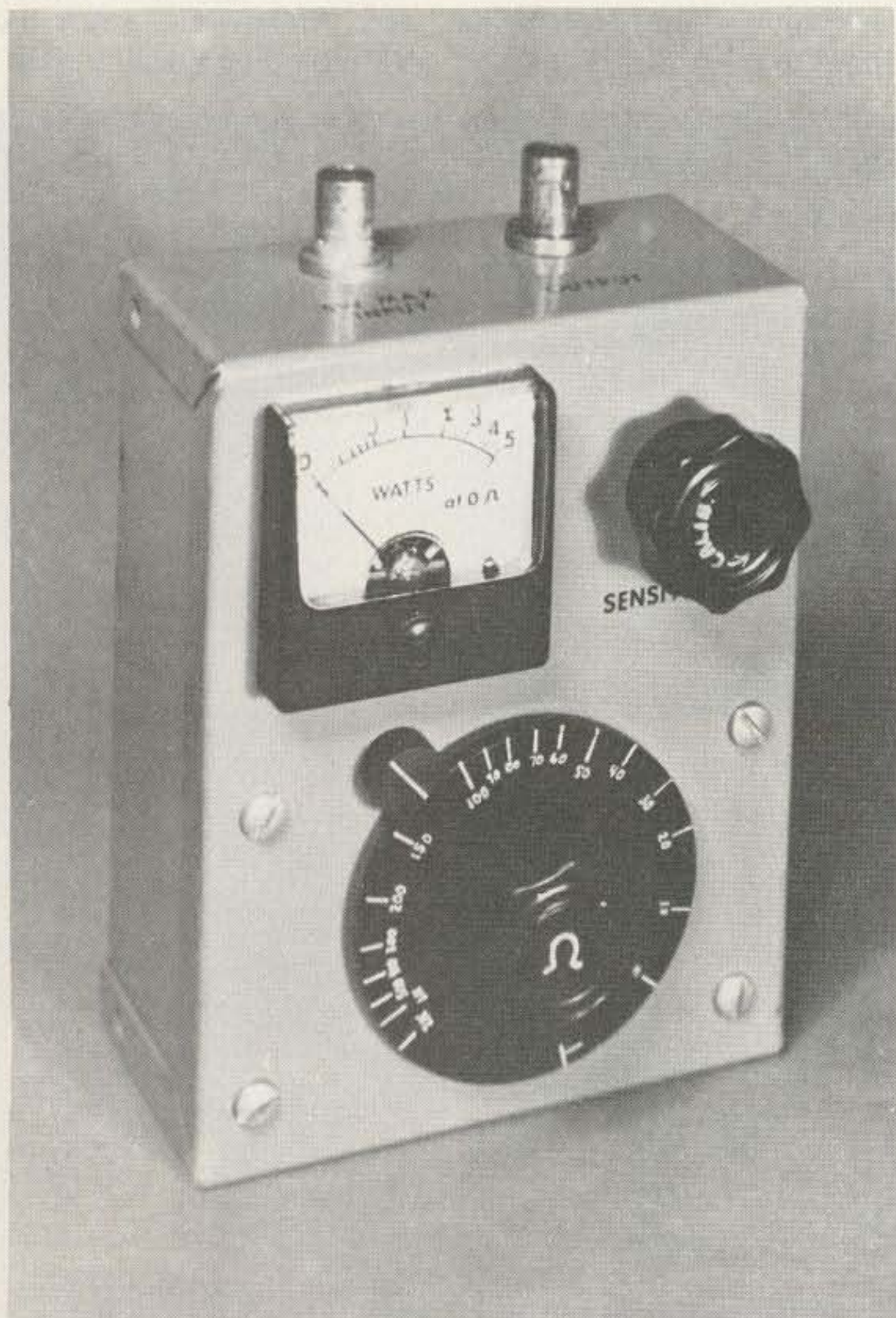
Photo A. Front view of the dummy load/wattmeter/RF bridge. The resistance dial is a 2-1/4" diameter plastic skirt attached to a standard knob.
