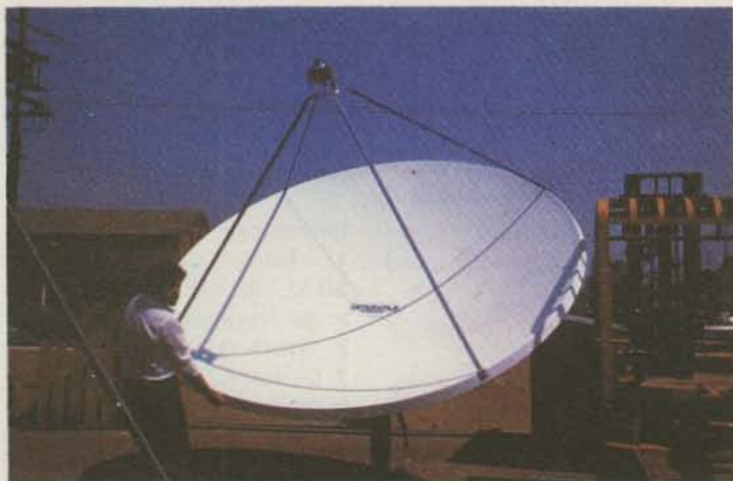
Fig. 1. The prime-focus design uses a parabolic reflector to concentrate the signal from the satellite into a small area known as the focus point. The accuracy of the dish surface to a true parabolic curve governs the size of the focus point and placement of the feedhorn.
