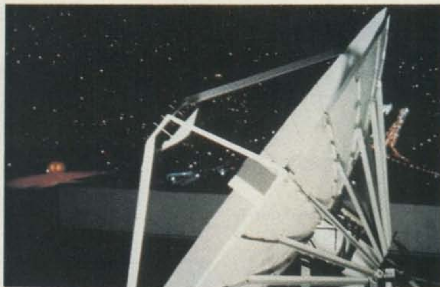
Fig. 2. The Cassegrain or twin-reflector design offers increased efficiency, but there are limits. As a rule, Cassegrains must be larger than ten feet before you can derive any benefit because the subreflector blocks a significant portion of the signal from ever reaching the dish.
