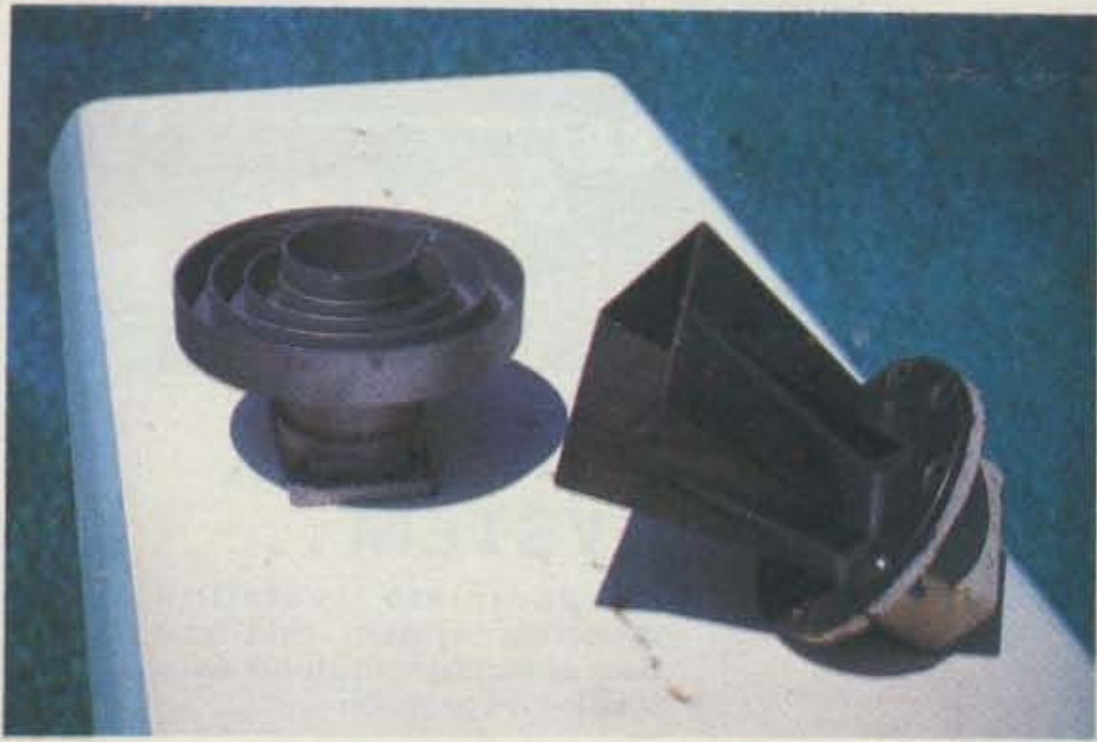
Fig. 7. Feeds may take on various shapes, but their sole purpose is to properly illuminate the dish. I had a chance to test several of the feedhorns sold today. My spectrum analyzer showed a drastic difference in gain and efficiency on my particular dish, so feed matching to the dish is important.
