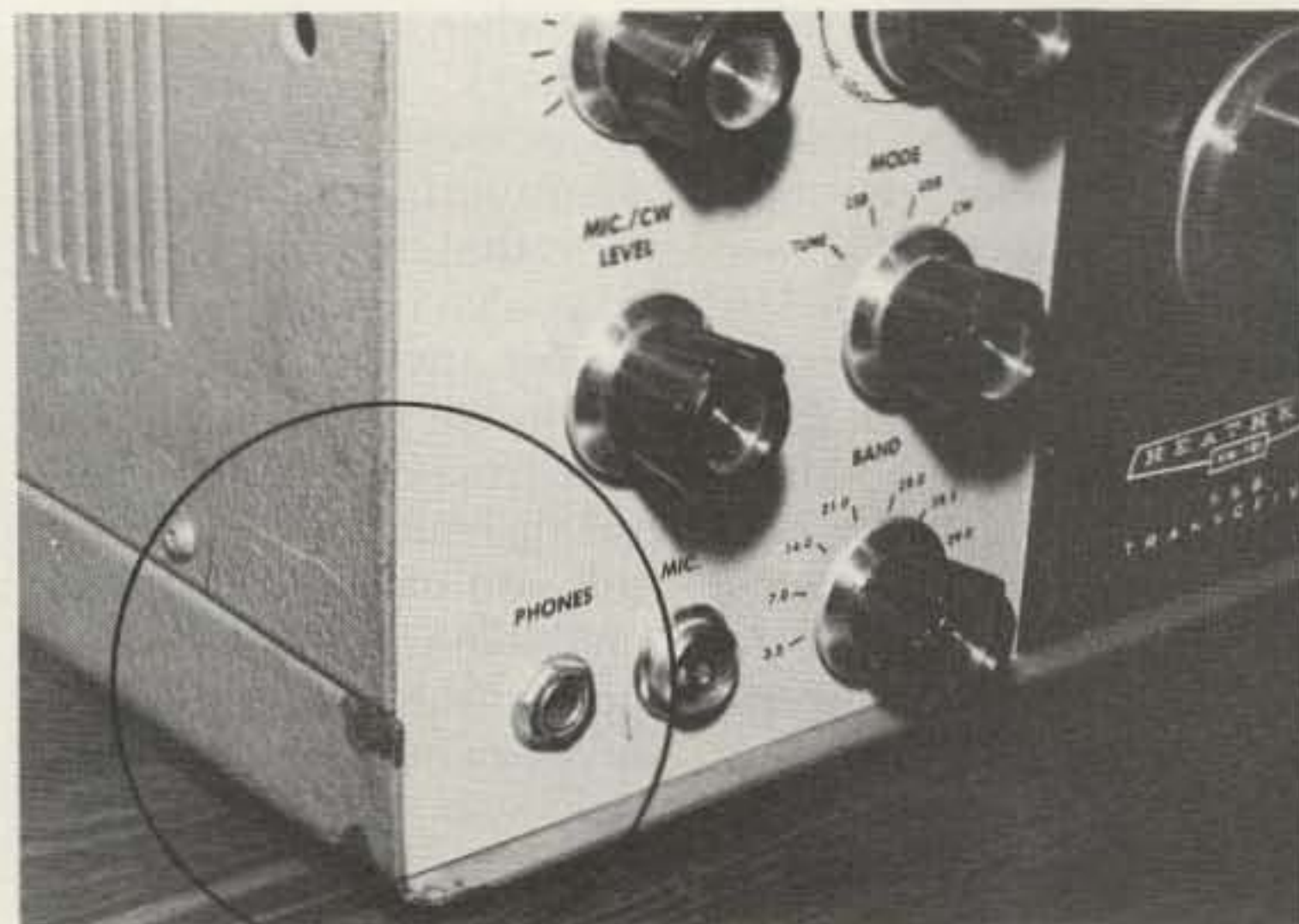
Don't let minor damage like chipped paint and superficial scratches (circled area) deter you from a good buy on an otherwise clean, operable rig.
