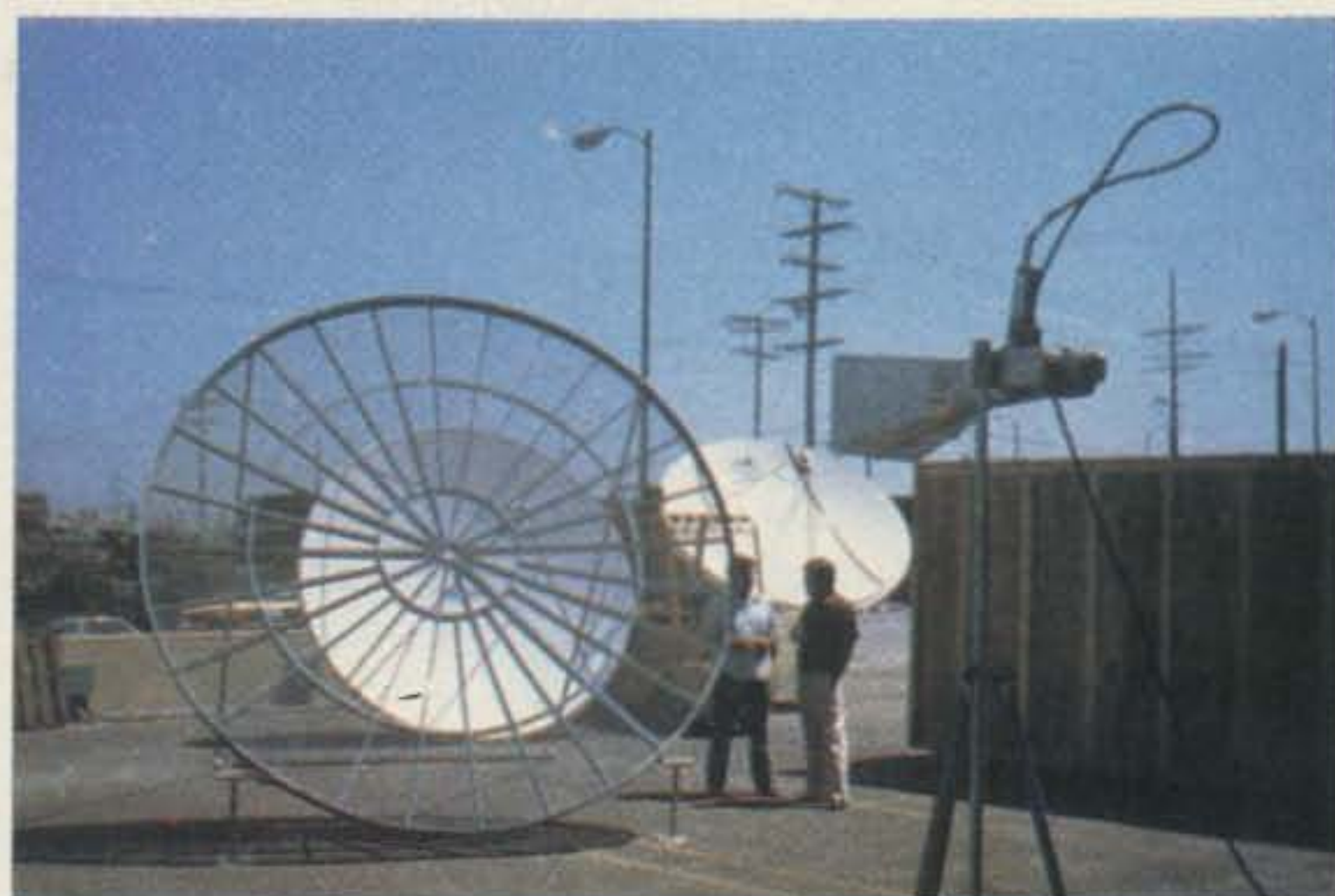
Fig. 3. Carve out a piece from a very large metal ball and you have the spherical antenna. It is possible to receive several satellites at once using separate feeds or you can simply mount the feed and LNA on a tripod and move it from satellite to satellite.
