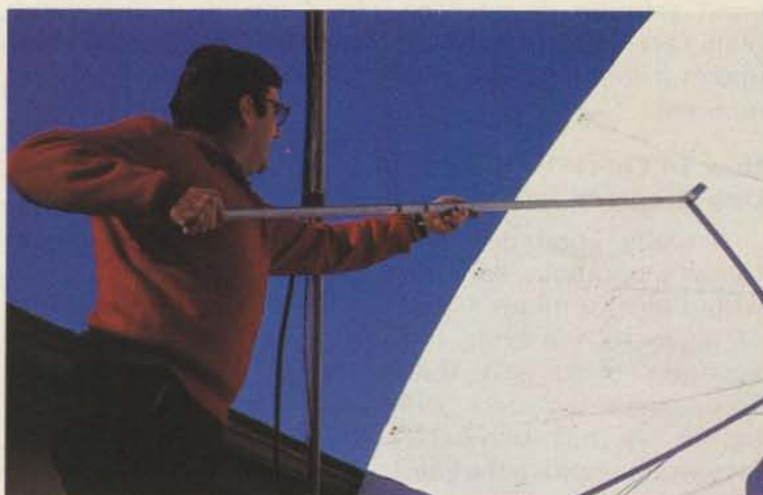
Fig. 3. A long pole or length of wall molding will reach anywhere on a dish and is safer. Tape the mirror to the pole like a hinge so it rests flat on the dish. Very few inexpensive dishes will pass this test. When you find one that does, buy it!
