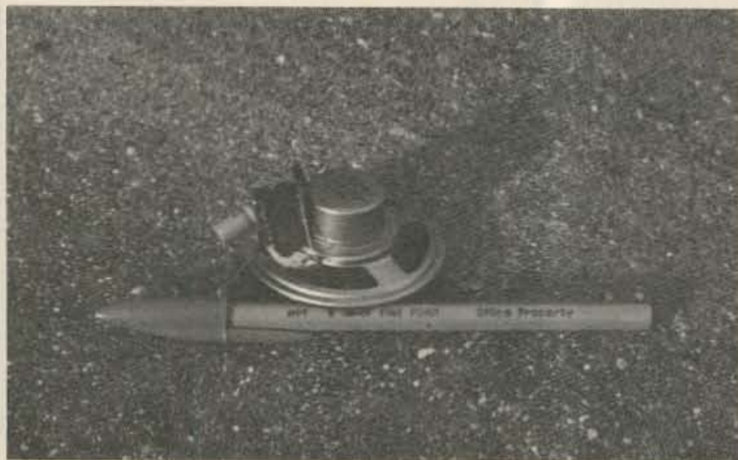
Fig. 1. The simplest cpo. The IC is a 7404 low-power Schottky hex inverter. C is a 5- to 30- \mu F electrolytic selected for desired pitch. The speaker is a 2-inch, 8-Ohm unit.
