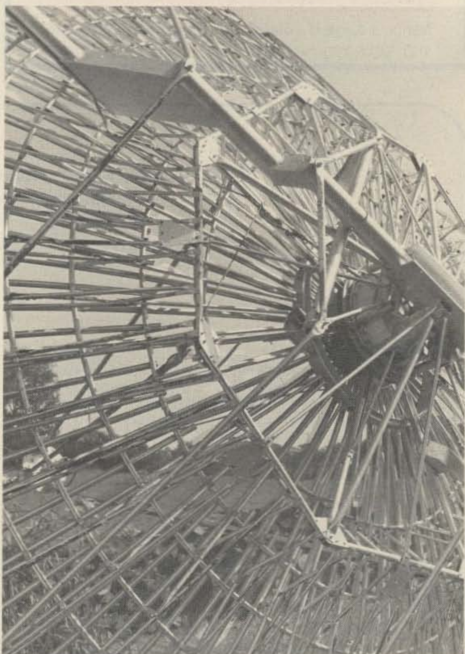
The dish, which is almost 16 feet in diameter, has a frame built from PVC pipe and electrical conduit. The supporting bar, which spans the dish, is the only piece that Tex did not fabricate himself.
