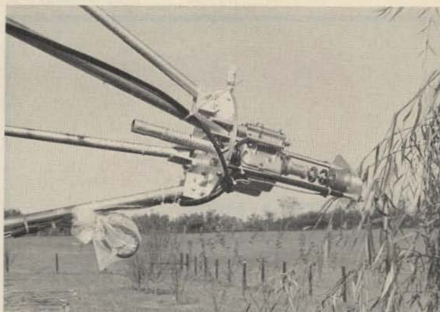
The feed assembly allows the horn polarization to be changed via a TV rotor and there is provision for very fine adjustments of the horn location. This allows the receive signal to be maximized.
