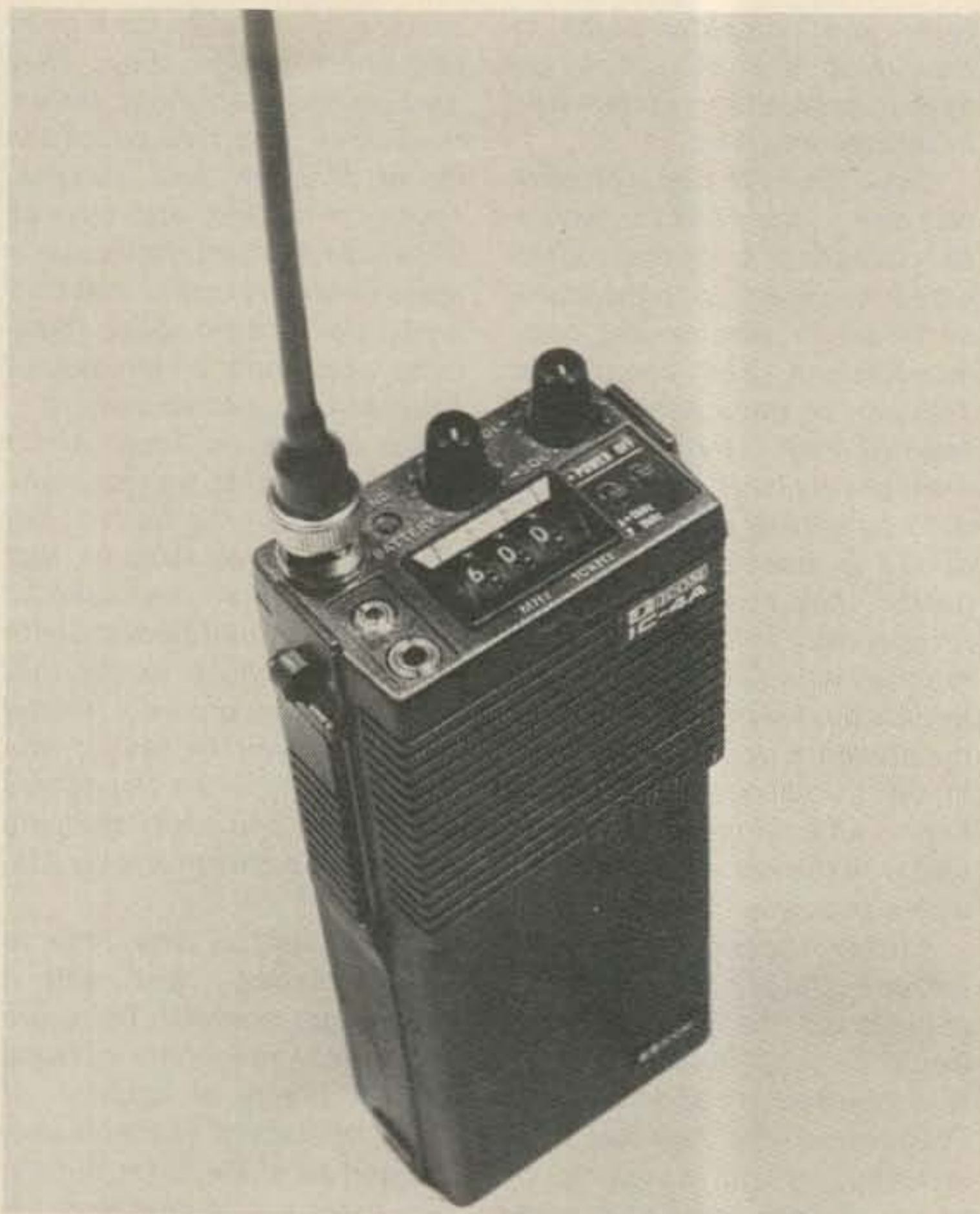
Photo A. The IC-4A hand-held 440-MHz FM transceiver. (Photo by Michael D. Landis)
