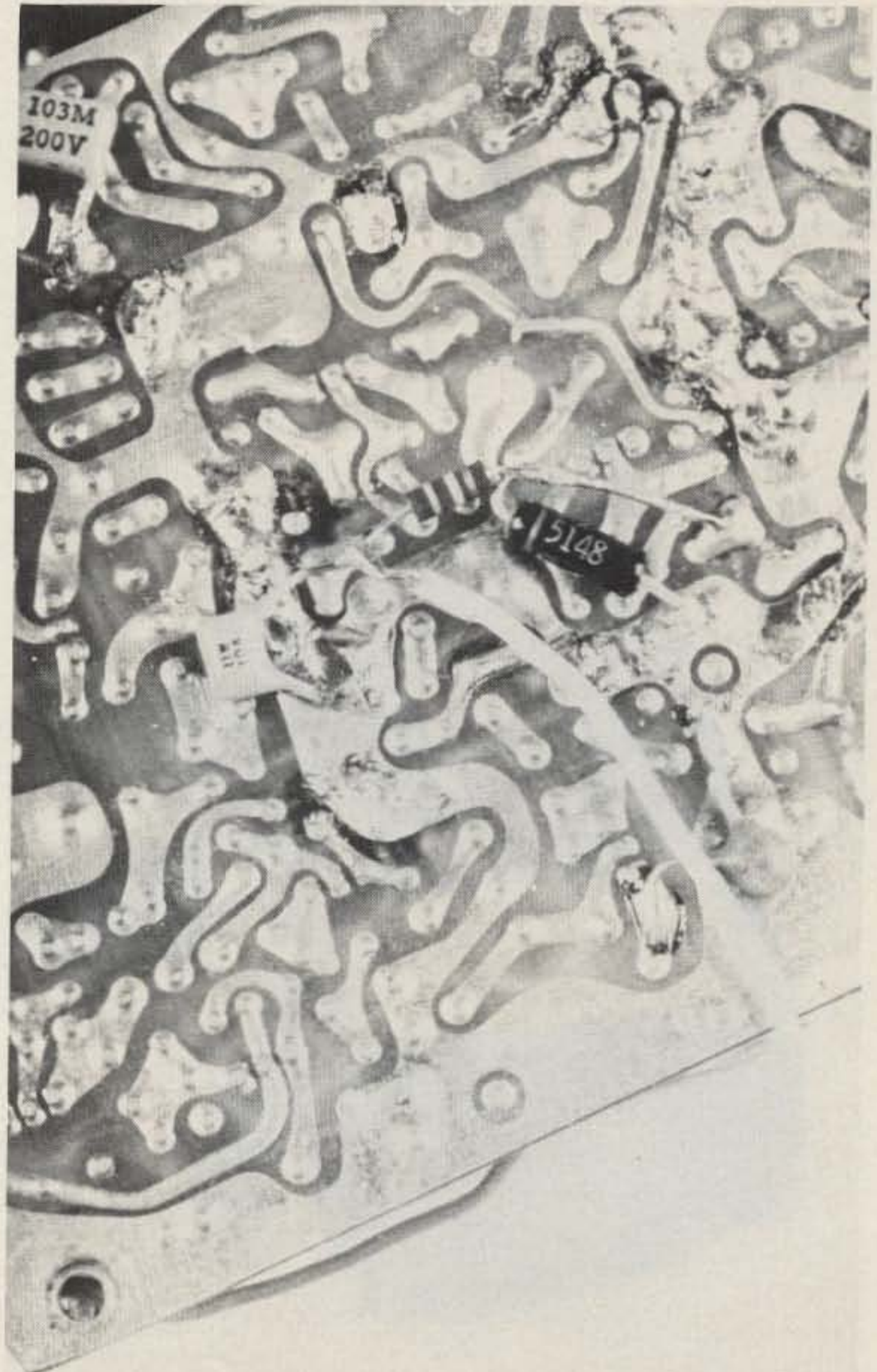
Fig. 6. Mounting of the varactor diode, C1', and R1' on the receiver board.
