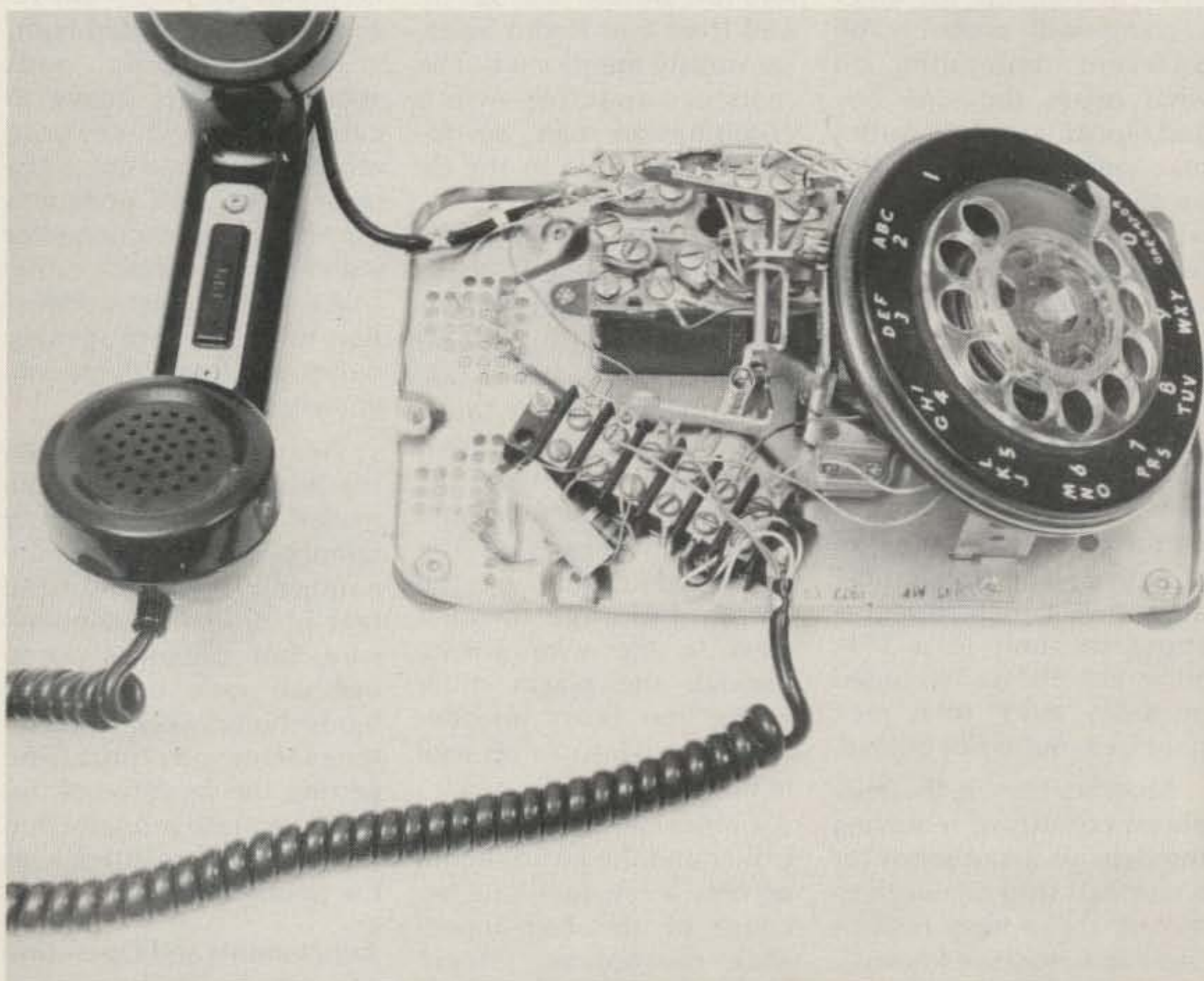
Photo C. Modified telephone set. Note the push-to-talk button in the handset and the resistor-capacitor combination mounted on the added terminal strip.
