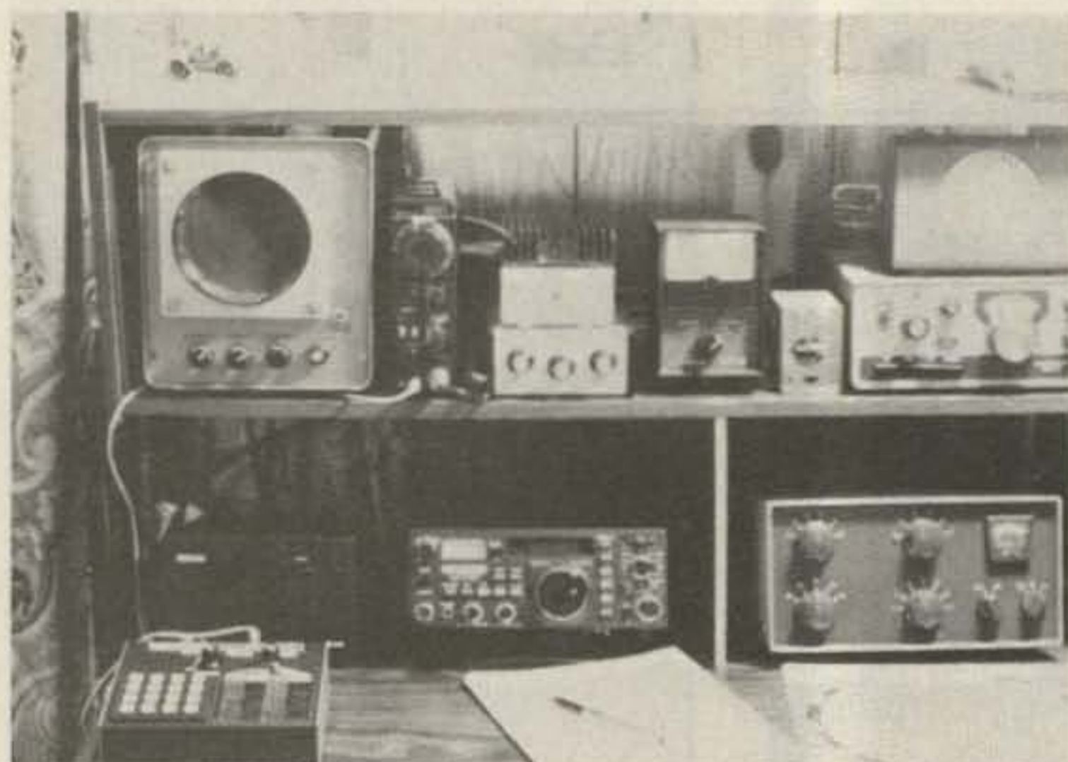
Amateur satellite setup at K4TWJ includes Icom 202 and 40-Watt amplifier for uplink, Icom 730 for downlink. 12-volt power for the 40-Watt amplifier is pulled from the Icom 730's PS15 power supply. SSTV capability included. The programmable Morsematic keyer was used for contacting RS5 and RS7 robots. SF radio desk with upper shelf holding 2-meter gear proves a great convenience for satellite operations.
