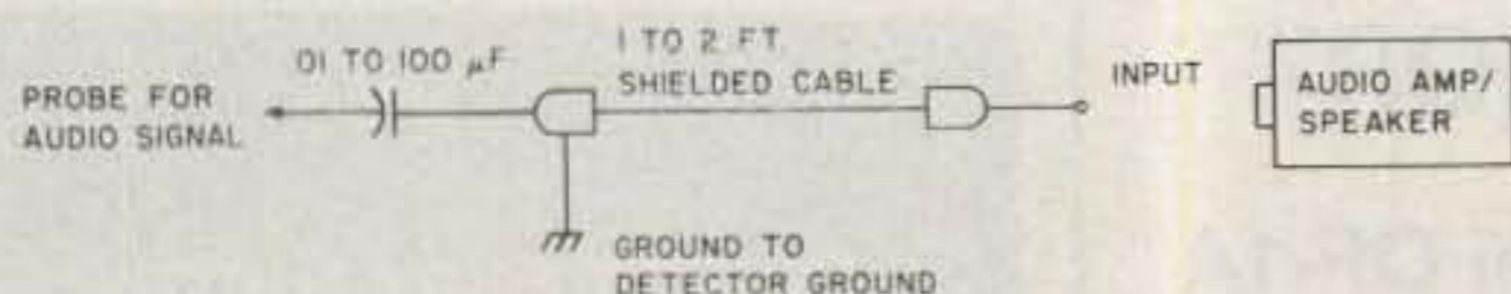
Fig. 6. Arrangement to probe for detector audio circuit. A hiss shows you have located a suitable point to connect the audio output.
