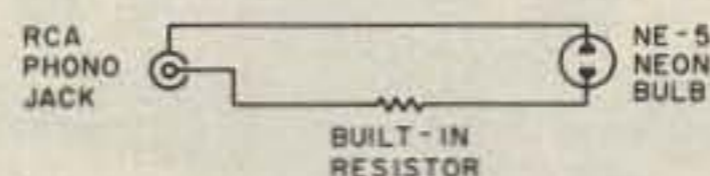
Fig. 1. One scientific circuit for detection of antenna voltage transients.
