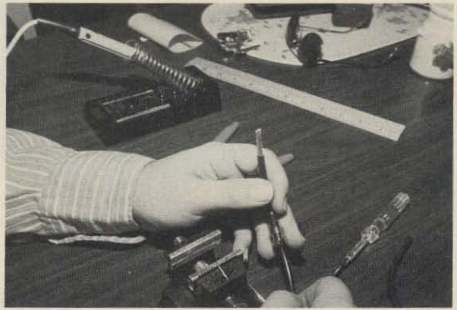
Once the layer of covering material is removed, you will find the tightly twisted shield braid exposed. Here you can see the exposed braid and the UG-175 adapter.
