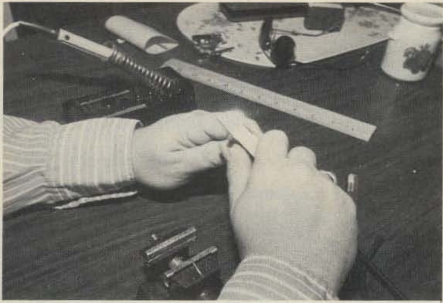
Cutting the outer covering of a piece of coax requires a sharp knife and a firm but gentle score around the plastic covering. If you cut too deeply, you risk cutting the outer braid of the coax.
