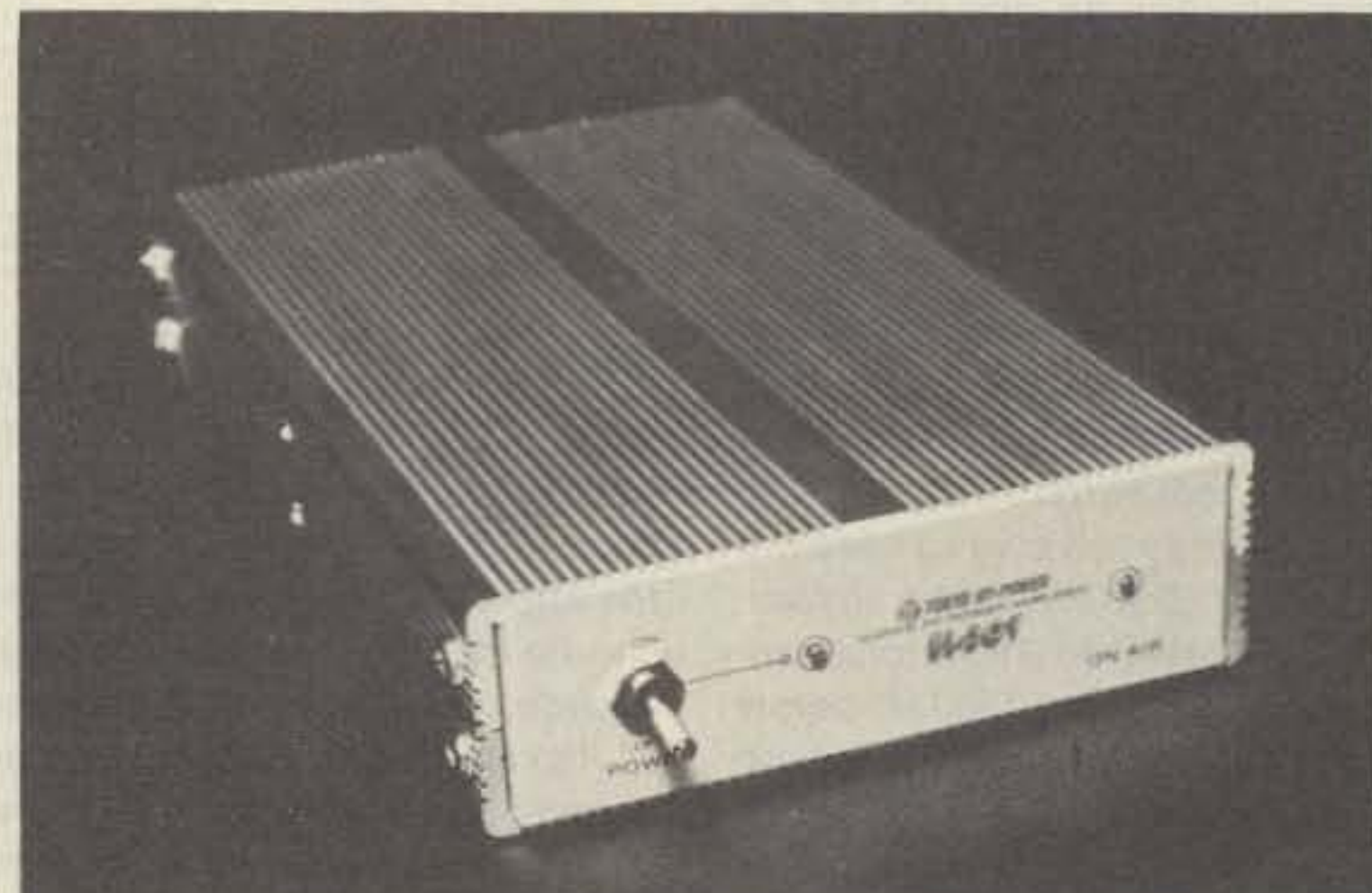
Encomm's HL-30V VHF linear amplifier.
