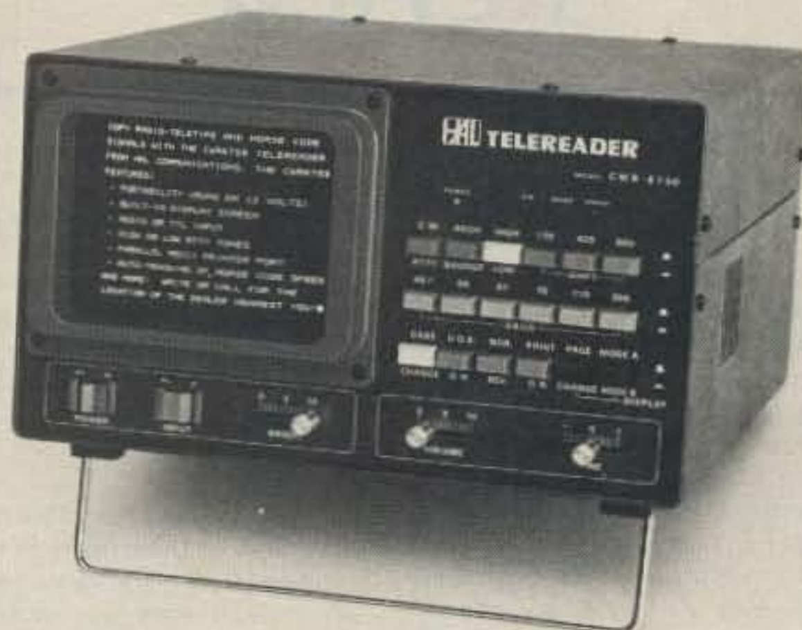
Hal's CWR6750 Telereader receive-only RTTY/CW terminal.
