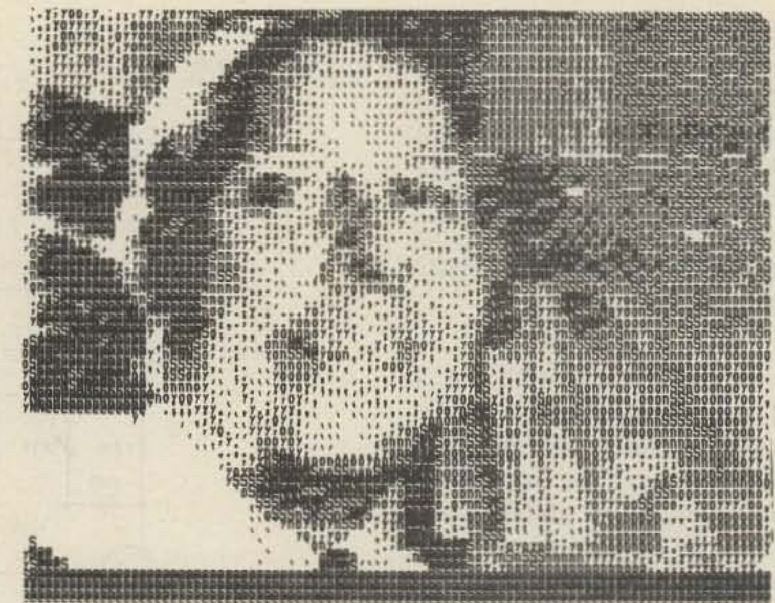
Fig. 3. Hard-copy picture produced by dot-matrix printer set for 16.5 characters per inch horizontally and 12 lines per inch vertically.
