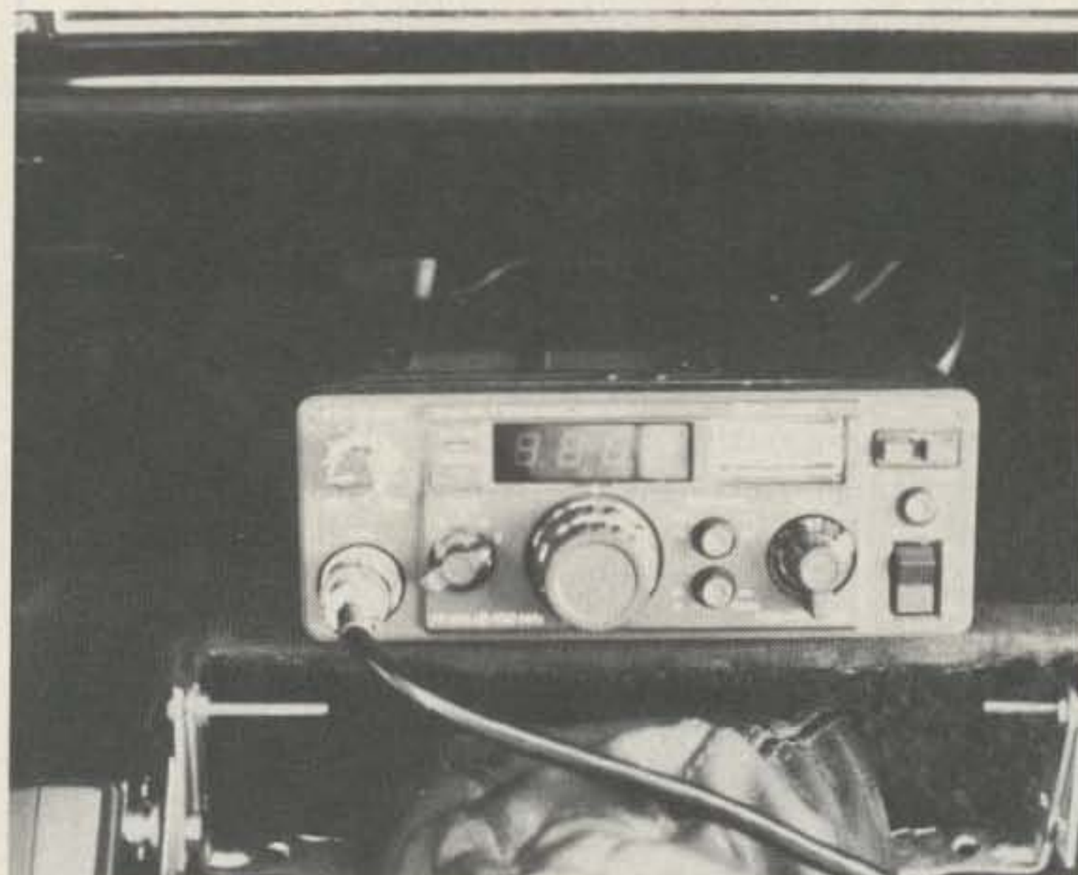
Fig. 6. A second (or third!) rig can be used with the bracket of Fig. 5. If front feet don't secure the rig, use a heavy rubber band. Note the mike mount on the left side of the bracket.
