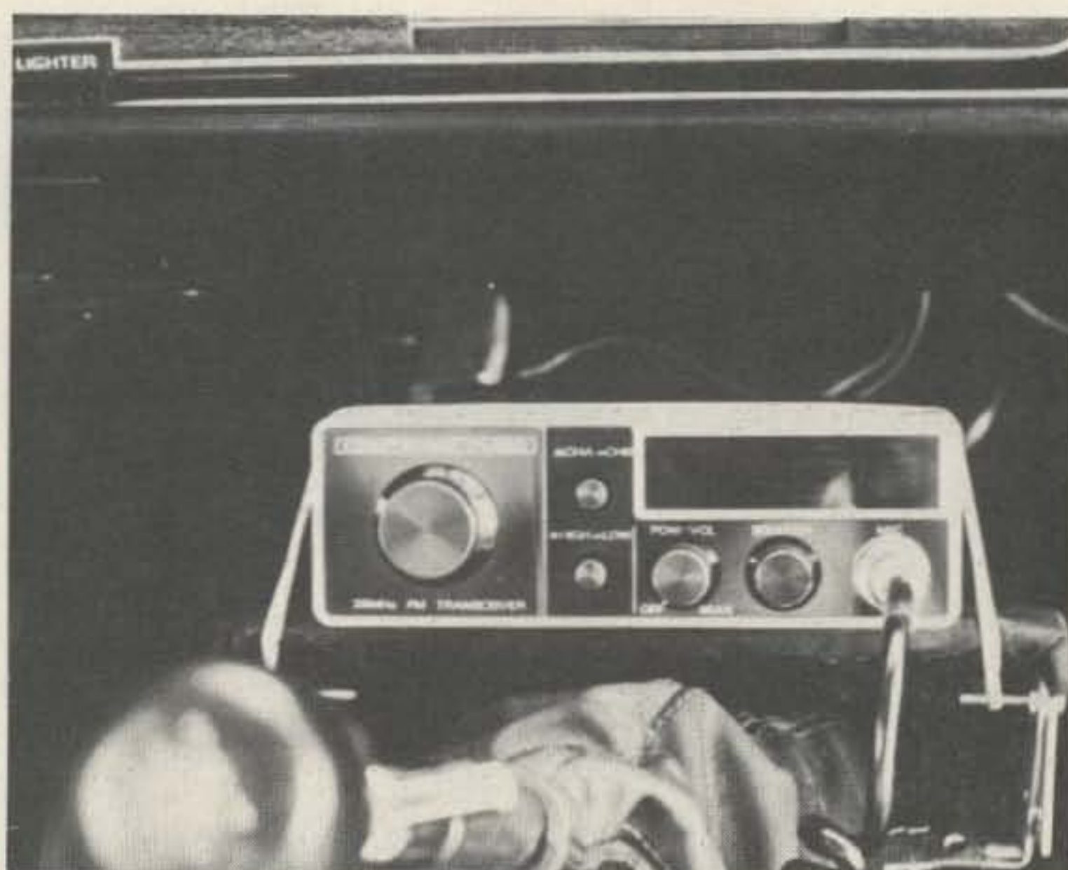
Fig. 5. This rig-mounting bracket is ideally suited to rapid installation artists. The unit is merely placed on the mount and secured with a heavy rubber band. Either top or bottom-mounted speakers can be used with this arrangement.
