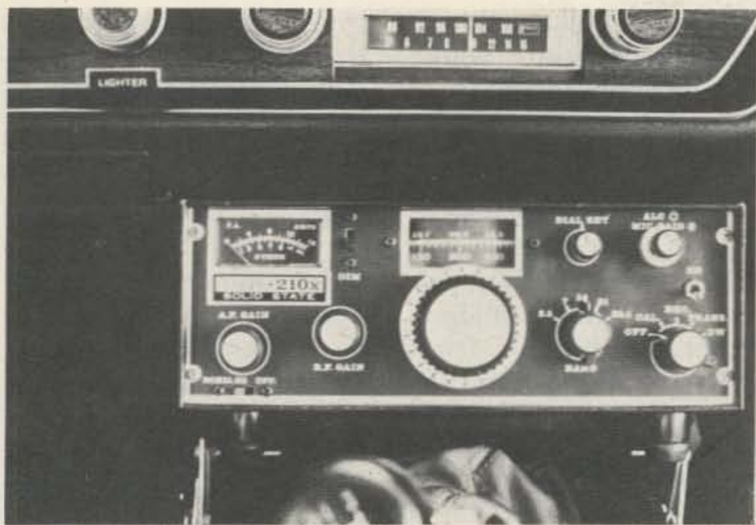
Fig. 4. Low-band transceiver is side-slid into position with its front feet catching on the bracket. The rear of the rig is sitting on the transmission hump. The squeezed position assists in securing the rig, eliminating need for a hold-down strap.
