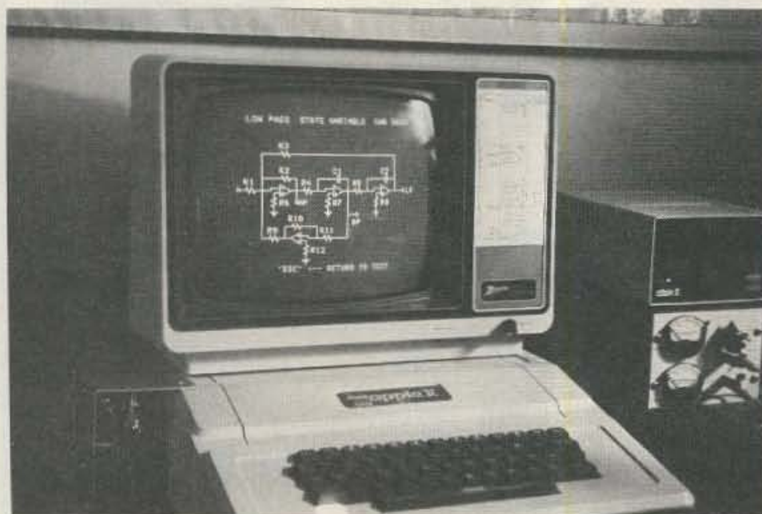
Fig. 1. Schematic of an active audio filter as it would appear within a program. This is typical of the type of schematic which may be incorporated in your programs.
