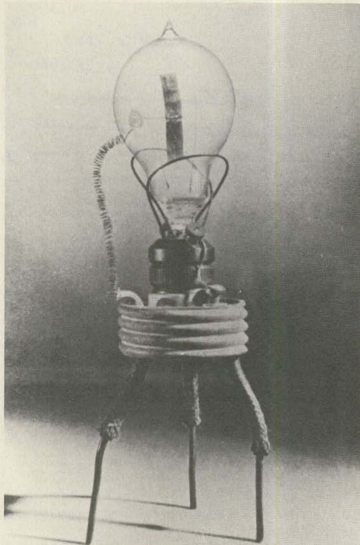
One of the Edison lamps used by Fleming in early experiments.
