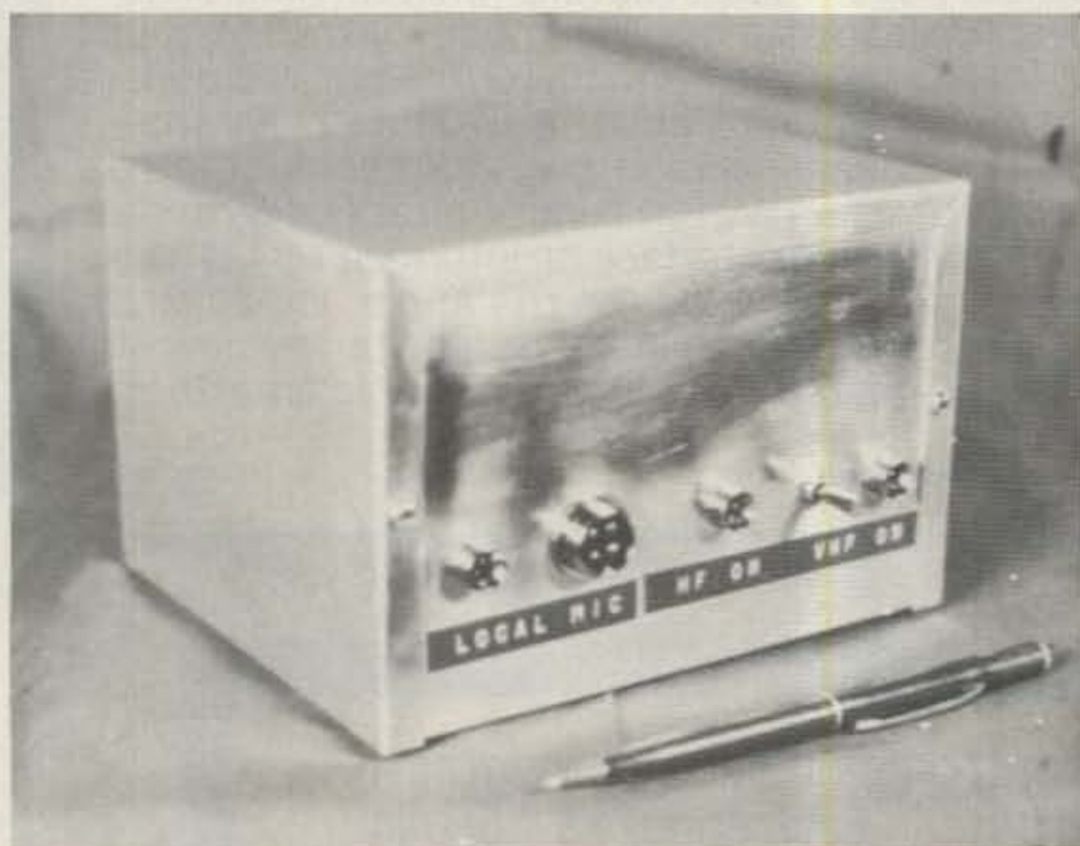
Photo A. Front view of the logic box.
